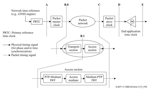
Figure 5 – Network reference model with access section
