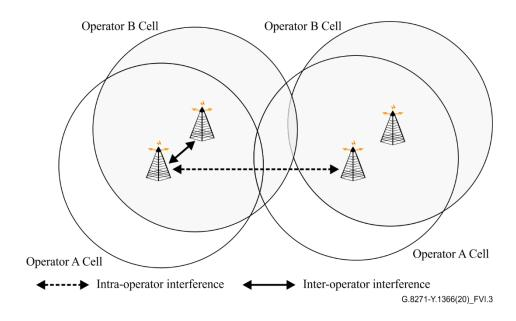
Figure VI.3 – Relationship between intra- and inter-operator interference
