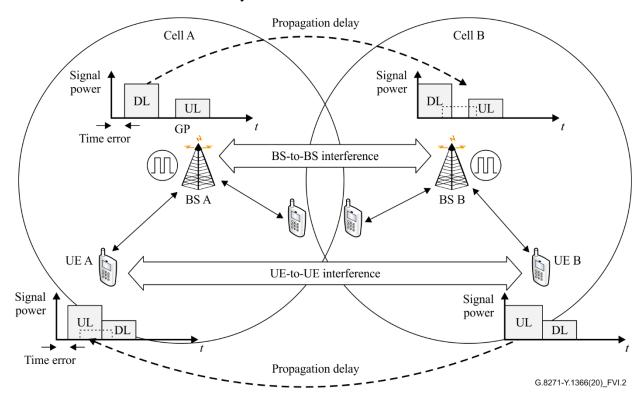
Figure VI.2 – Overview of interference patterns in TDD systems
