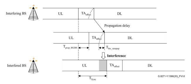
Figure VI.6 – BS to BS interference at UL to DL switching point
