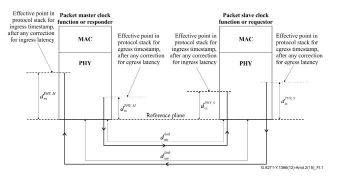
Figure I.1 – Illustration of delays between a packet slave clock function, or requestor, and a packet master clock function, or responder
