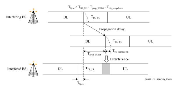
Figure VI.5 – BS to BS interference at DL to UL switching point
