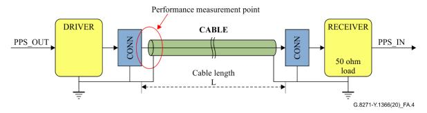
Figure A.4 – Unbalanced 1PPS 50  $\Omega$  measurement interface
