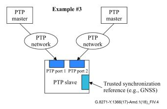
Figure IV.4 – Monitoring of semi-static asymmetry
