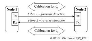
Figure IV.1 – Link asymmetry calibration process (performed separately on both fibres)
