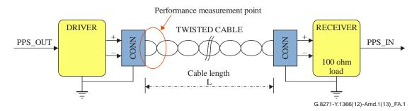
Figure A.1 – Balanced 1PPS V.11 interface
