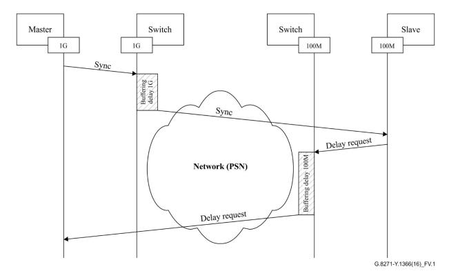
Figure V.1 – Speed mismatch example
