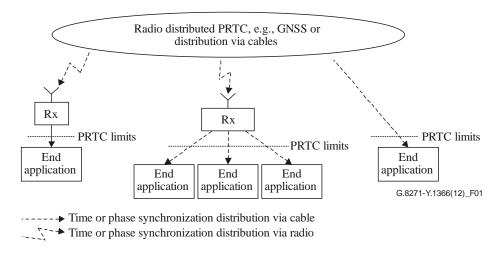
Figure 1 – Example of a distributed PRTC synchronization network
