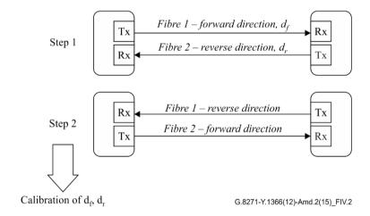
Figure IV.2 – Link asymmetry calibration process (performed on both fibres at the same time)
