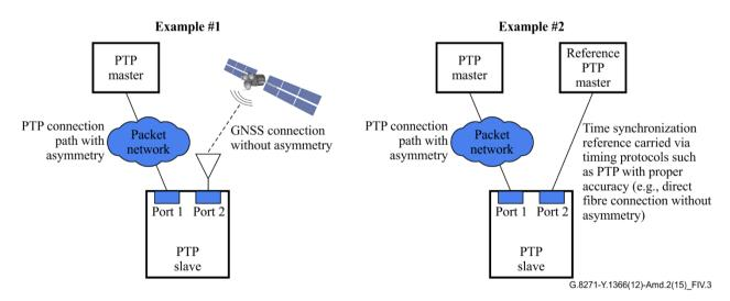
Figure IV.3 – PTP slave evaluating PTP connection asymmetry
