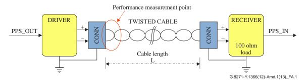
Figure A.1 – Balanced 1PPS V.11 interface
