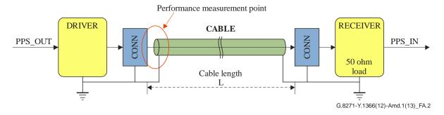
Figure A.2 – Unbalanced 1PPS 50  $\Omega$  measurement interface
