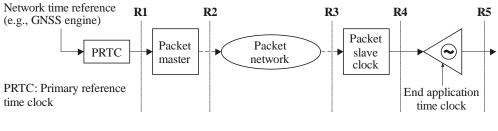
→ Physical timing signal (for phase and/or time synchronization)
