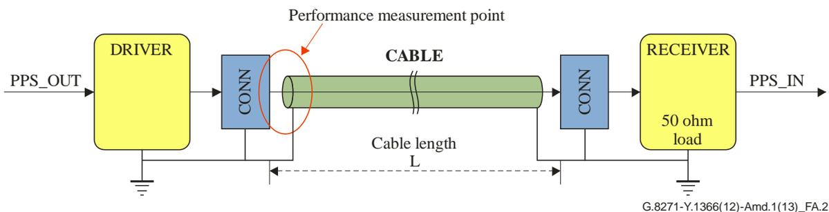
**Figure A.2 – Unbalanced 1PPS 50 Ω measurement interface**
