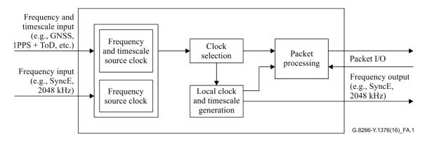
Figure A.1 – PEC-M functional model
