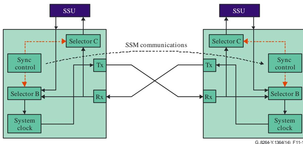
**Figure 11-1 – Simplified SSM channel**
