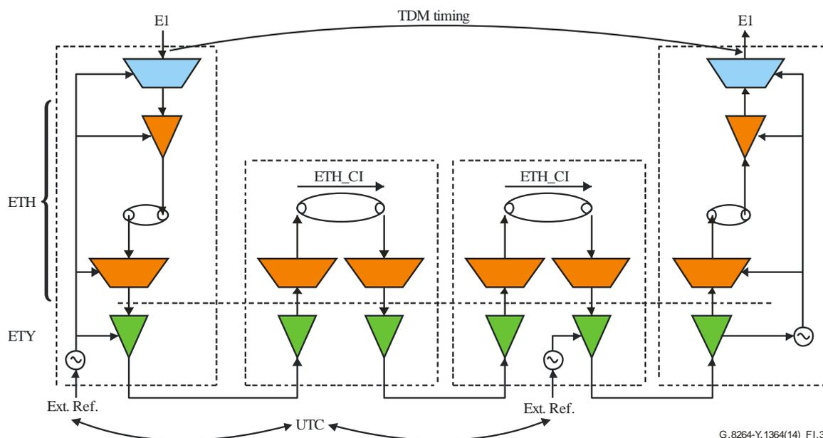
**Figure I.3 – TDM over Ethernet network**
