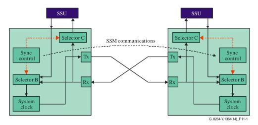
Figure 11-1 – Simplified SSM channel
