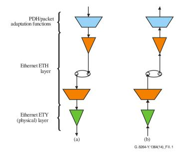
Figure II.1 – Functional blocks within CES IWF
