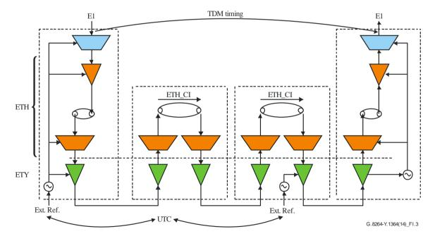
Figure I.3 – TDM over Ethernet network
