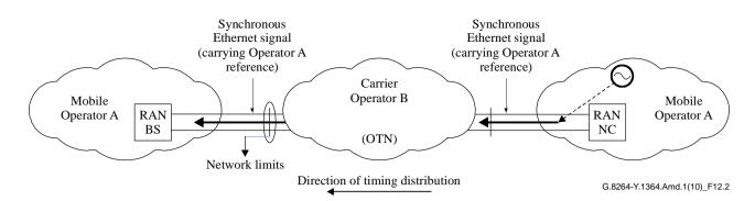
Figure 12-2 – Illustration of a timing transparent transport of the synchronous Ethernet client signals in the multi-operator context
