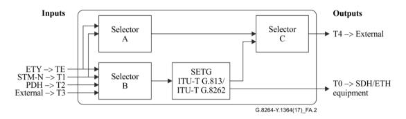
Figure A.2 – Hybrid SDH/synchronous Ethernet SETS function
