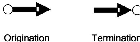
**Figure 8-3 – Timing flow origination and termination**
