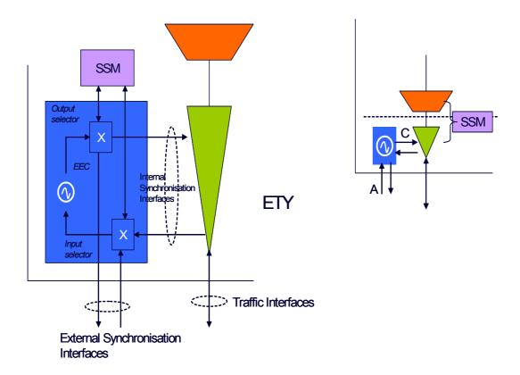
Figure A.1 – Synchronous Ethernet equipment – High level representation of synchronization sub-system selection mechanism
