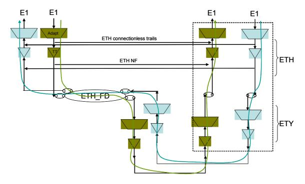
Figure I.2 – ITU-T G.8010 Ethernet network architecture showing circuit emulation and timing trails
