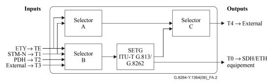
Figure A.2 – Hybrid SDH/synchronous Ethernet "SETS" function
