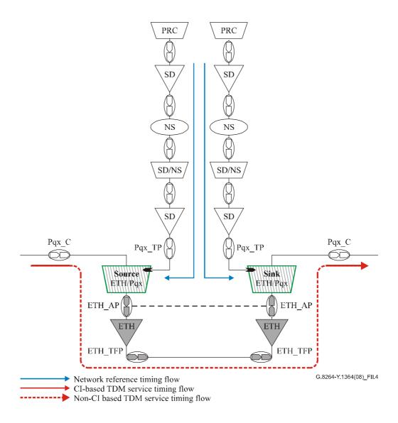
Figure II.4 – Functional models for differential timing
