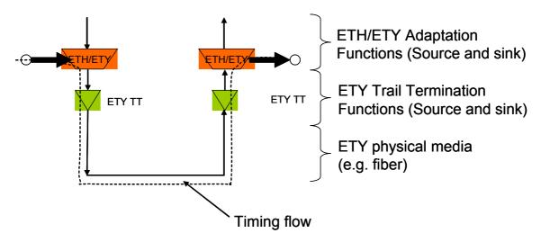
Figure II.2 – Functional model for Ethernet timing (synchronous Ethernet PHY)
