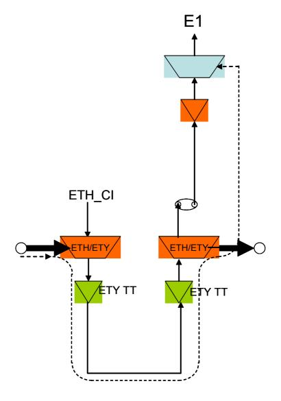
Figure II.3 – Example of using physical layer timing to provide timing to a ETH/PDH adaptation function
