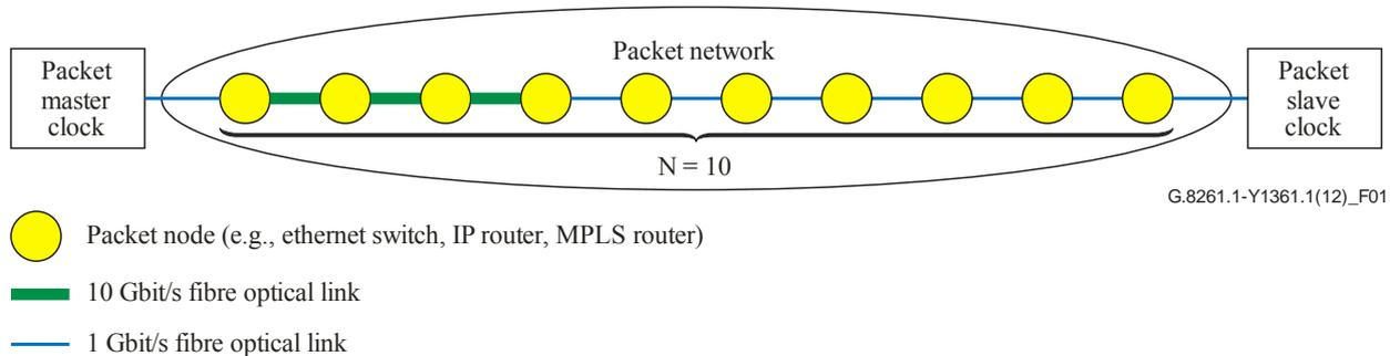
**Figure 1 – HRM-1 for packet delay variation network limits**
