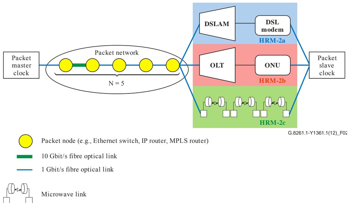
**Figure 2 – HRM-2 for packet delay variation network limits**
