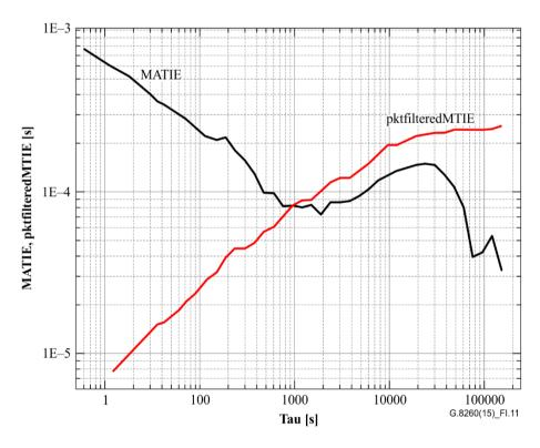
Figure I.11 – Example MATIE and pkfilteredMTIE data
