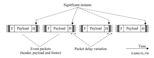
Figure 6 – Packet timing signal
