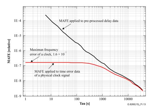
Figure I.13 – MAFE applied to pre-processed delay data and to time error data of physical clock
