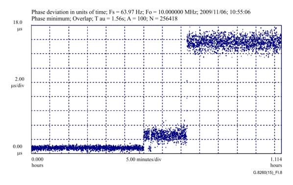
Figure I.8 – Minimum tracking statistic shows three distinct sections
