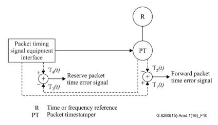
Figure 10 – Configuration for packet timing signal equipment interface measurement
