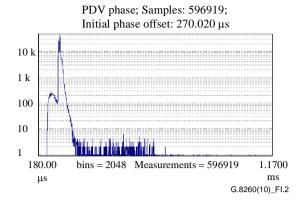
Figure I.2 – Measured packet delay and corresponding PDV histogram
