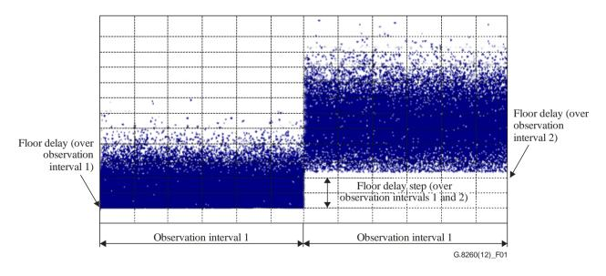
Figure 1 – Illustration of observed floor delays and floor delay step
