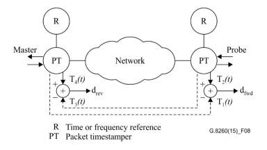
Figure 8 – Configuration for packet delay sequence measurement
