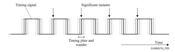
Figure 5 – Physical layer timing signal
