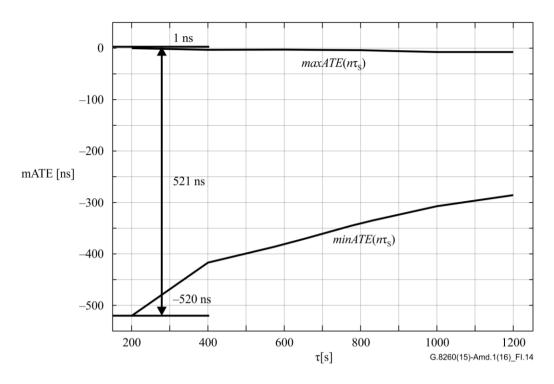
Figure I.14 – Example of average time error calculation
