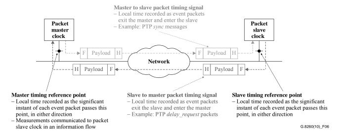
Figure 7 – Packet timing signal flow and timing reference points
