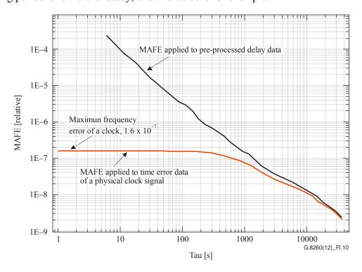
Figure I.10 – MAFE applied to pre-processed delay data and to time error data of physical clock
