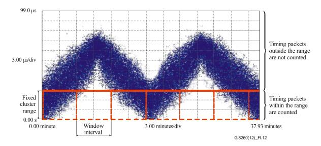
Figure I.12 – Example of PDV metric studying the population of packets within a fixed cluster range starting at the observed floor delay
