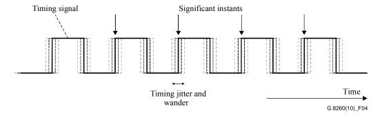
Figure 5 – Physical-layer timing signal
