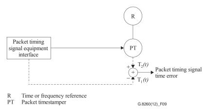
Figure 9 – Configuration for packet timing signal equipment interface measurement
