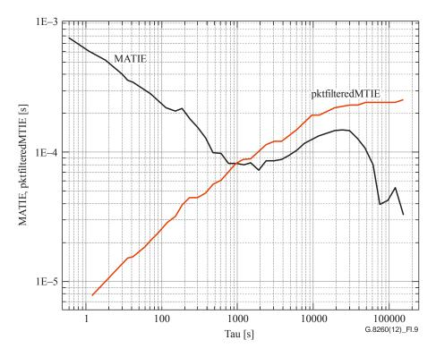
Figure I.9 – The black curve represents MATIE applied to pre-processed delay data. The red curve depicts *pktfiltered*MTIE, see I.4.2, with a 960s averaging function. These values are for example.
