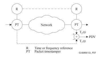
Figure 8 – Configuration for PDV measurement
