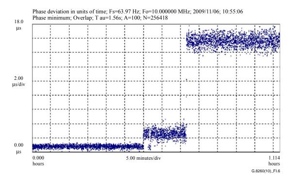
Figure I.6 – Minimum tracking statistic shows three distinct sections
