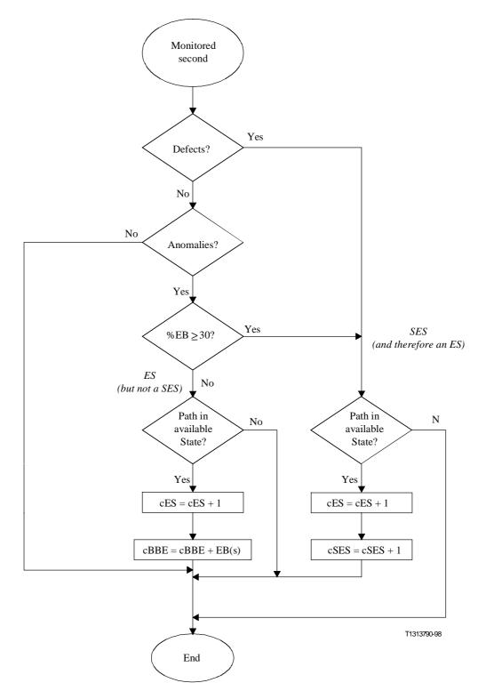
Figure I.1/G.826 – Flow chart illustrating the recognition of anomalies, defects, errored blocks, ES, SES and BBE
