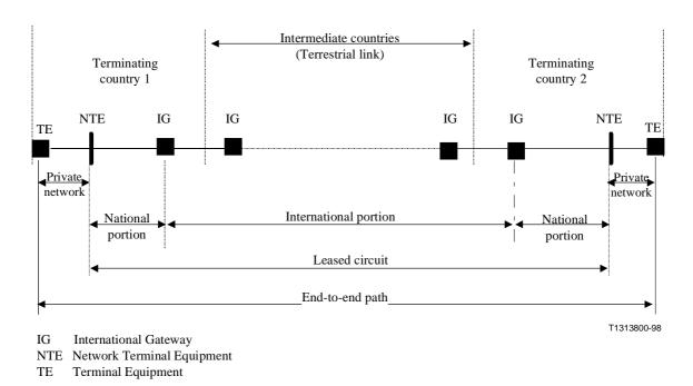
Figure III.1/G.826 – Digital path composed of two private networks and a leased circuit provided by a public network operator
