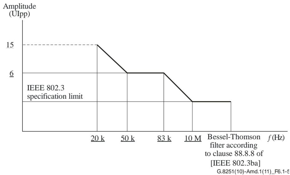
**Figure 6.1-5 – OTL4.4 per lane input sinusoidal jitter tolerance limit**
