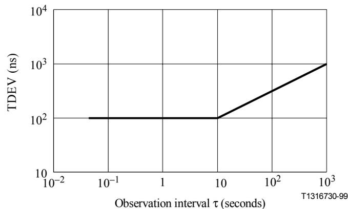
**Figure 4/G.824 – TDEV limit for 1544 kbit/s reference signals**
