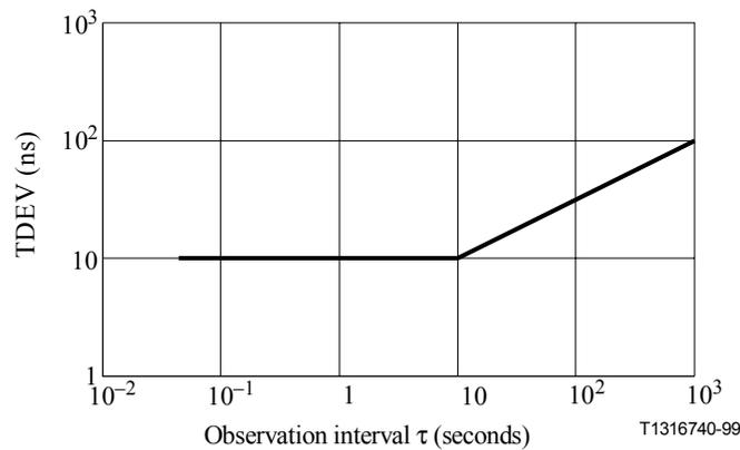
**Figure 5/G.824 – TDEV limit for 1544 kbit/s reference signals suitable for timing an Option-2 SEC**
