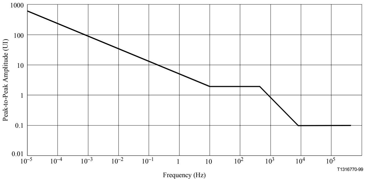
**Figure 8/G.824 – Jitter and wander tolerance of 32 064 kbit/s input ports**
