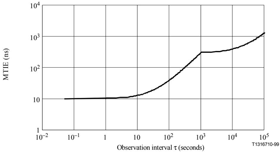
**Figure 2/G.824 – MTIE limit at the output of a Primary Reference Clock**
