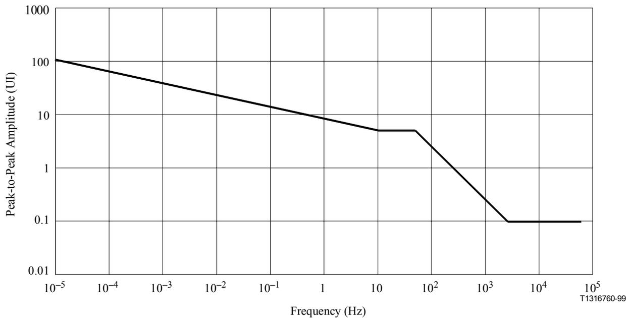
**Figure 7/G.824 – Jitter and wander tolerance of 6312 kbit/s input ports**
