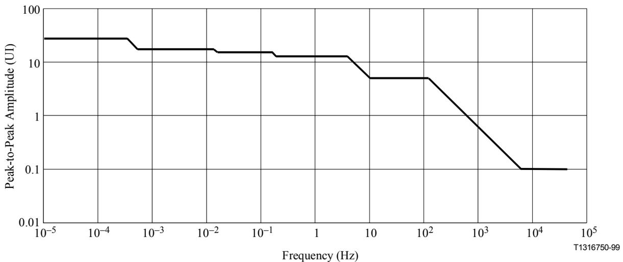
**Figure 6/G.824 – Jitter and wander tolerance of 1544 kbit/s input ports**
