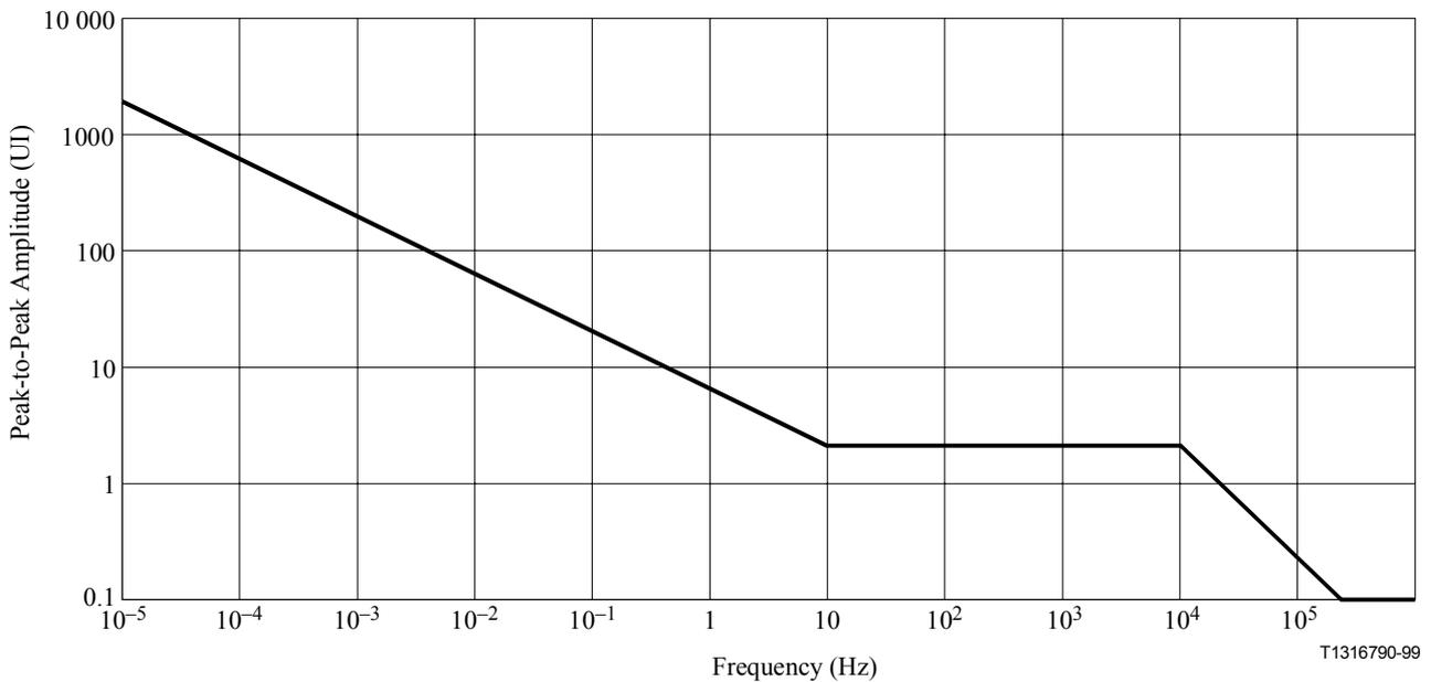
**Figure 10/G.824 – Jitter and wander tolerance of 97 728 kbit/s input ports**
