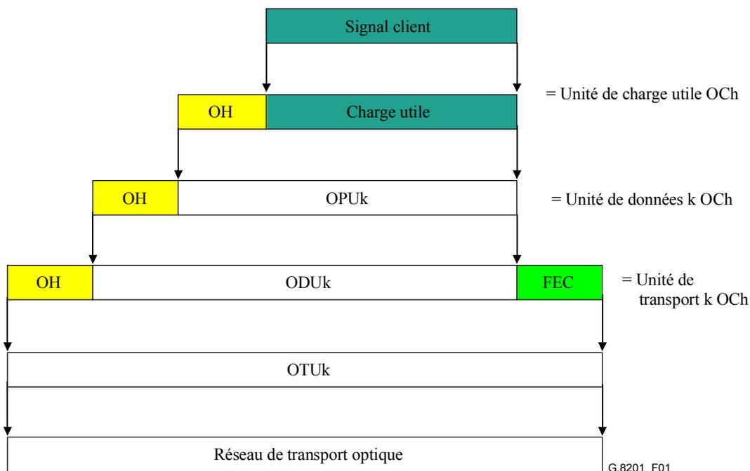
Figure 1/G.8201 – Structure du signal OTN
