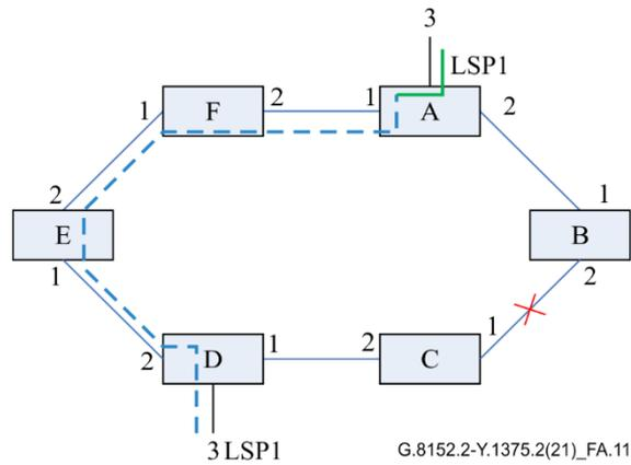
**Figure A.11 – Steering for link failure**
