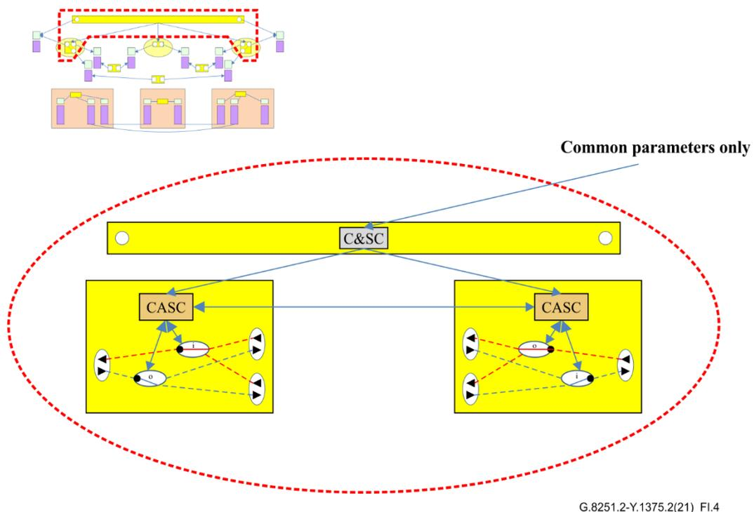
**Figure I.4 – Showing a high-level abstract controller in a 1:1 case**
