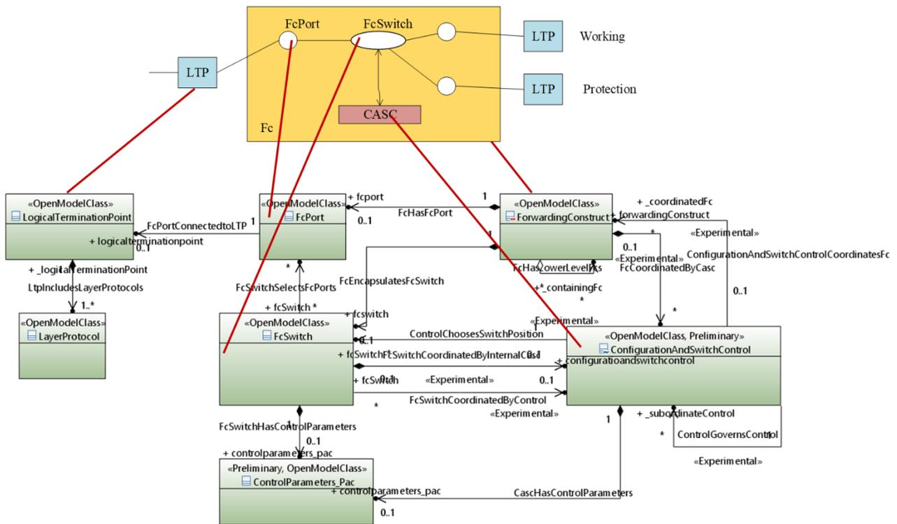
**Figure 7-2 – Simplified resilience model for MPLS-TP linear protection**
