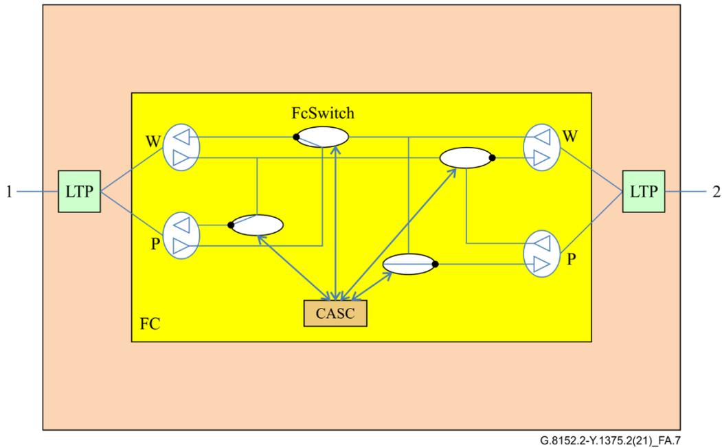
**Figure A.7 – Wrapping: Node B with failure on link between node B and node C**
