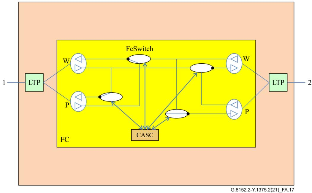
**Figure A.17 – Wrapping: Node B with failure on link between node B and node C**
