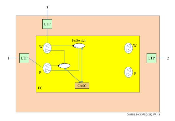
Figure A.13 – Steering: Node A with failure on link between node B and node C
