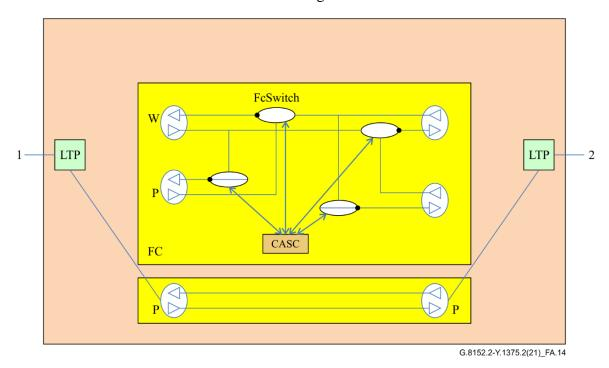
Figure A.14 - Steering: Node E and node F with failure on link between node B and node C
