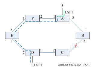
Figure A.11 – Steering for link failure
