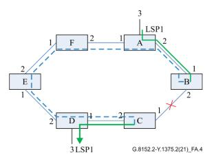
Figure A.4 – Wrapping for link failure
