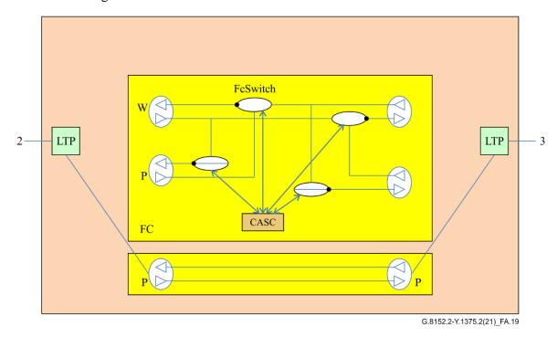
Figure A.19 – Short-wrapping: Node D with failure on the link between node B and node C
