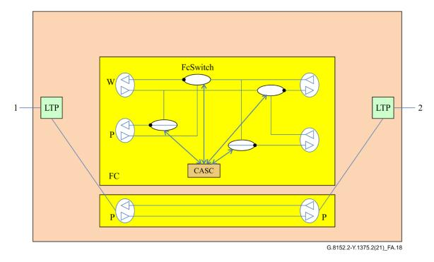
Figure A.18 – Short-wrapping: Node E and node F with failure on link between node B and node C
