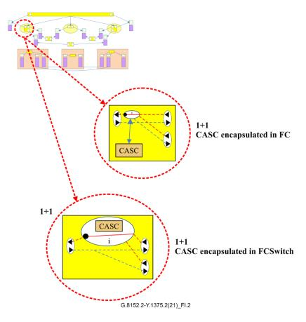
Figure I.2 – Detail of a nodal view of 1+1 switches
