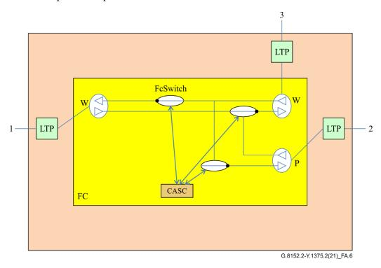
Figure A.6 – Wrapping: Node D (no failure in ring)
