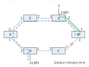
Figure A.16 – Short-wrapping for link failure
