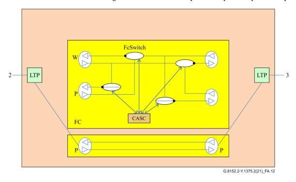
Figure A.12 – Steering: Node D with failure on link between node B and node C
