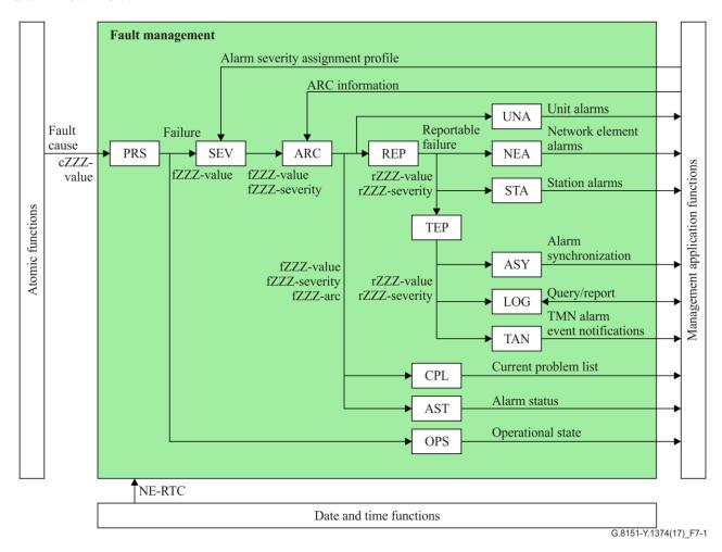
Figure 7-1 – Fault management within the MPLS-TP NEF
