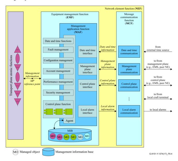
Figure 6.4 – MPLS-TP equipment management function
