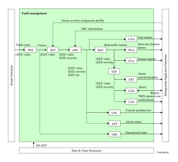
Figure 7-1/G.8151/Y.1374– Fault management within the T-MPLS NEF
