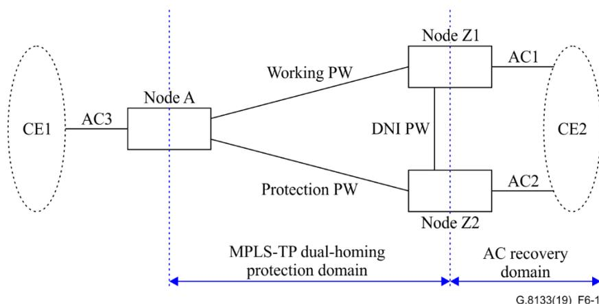
**Figure 6-1 – One-side MPLS-TP dual-homing reference network**
