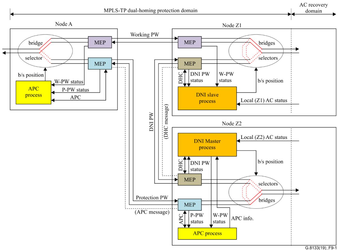
**Figure 9-1 – MPLS-TP Dual-homing protection architecture**
