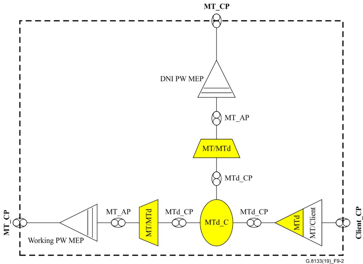
**Figure 9-3 – MPLS-TP dual-homing protection sub-layer (Z2)**
