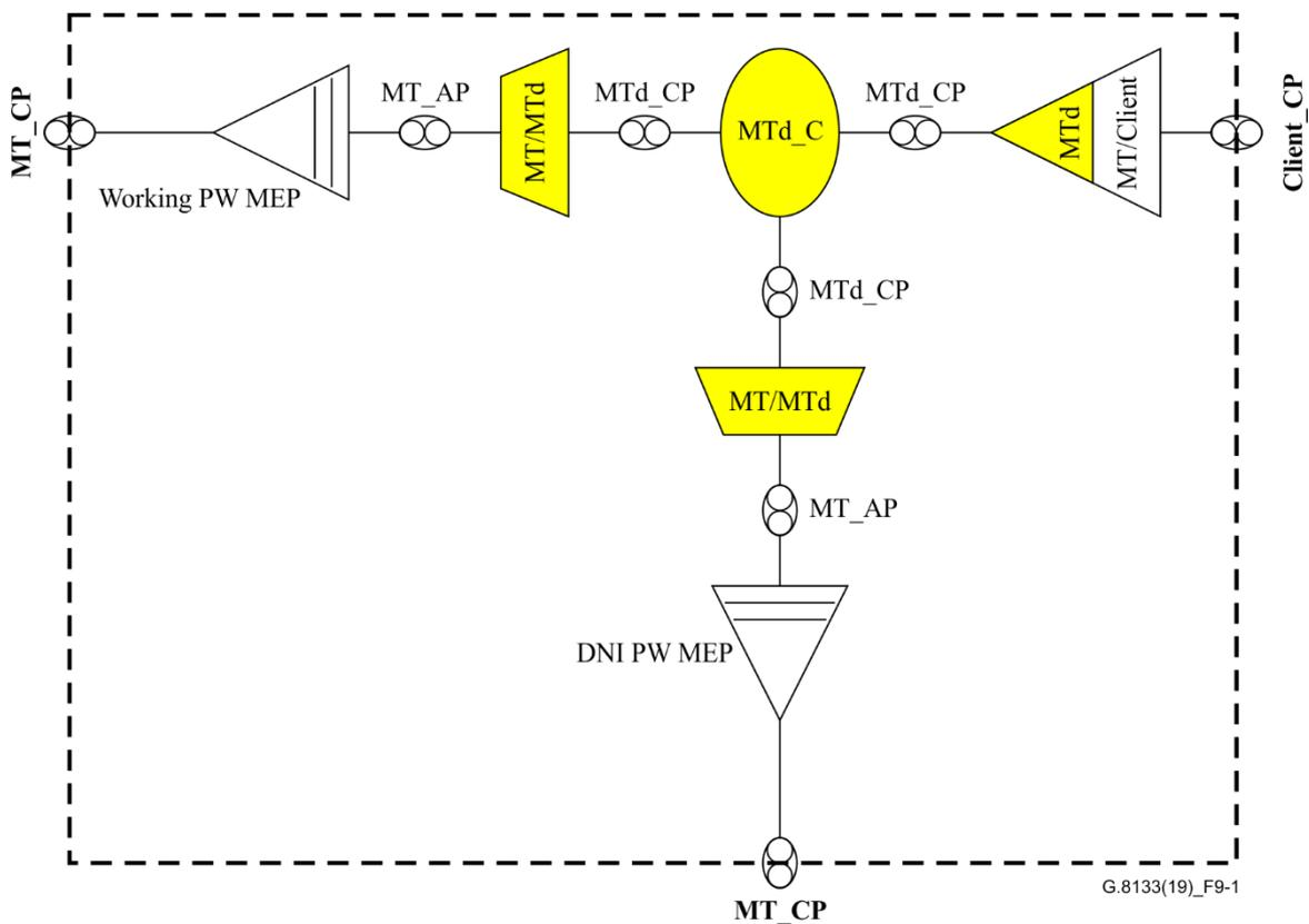
**Figure 9-2 – MPLS-TP dual-homing protection sub-layer (Z1)**
