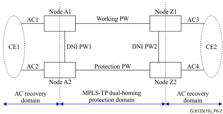
**Figure 6-2 – Two-side MPLS-TP dual-homing reference network**
