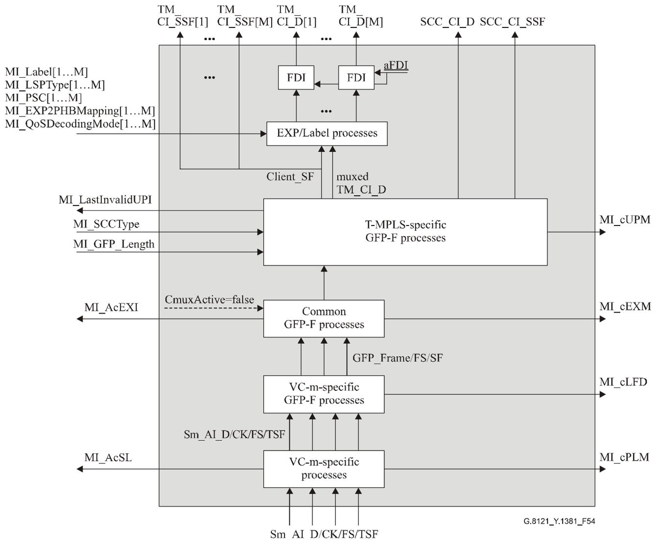
**Figure 54/G.8121/Y.1381 – Sm/TM\_A\_Sk process diagram**
