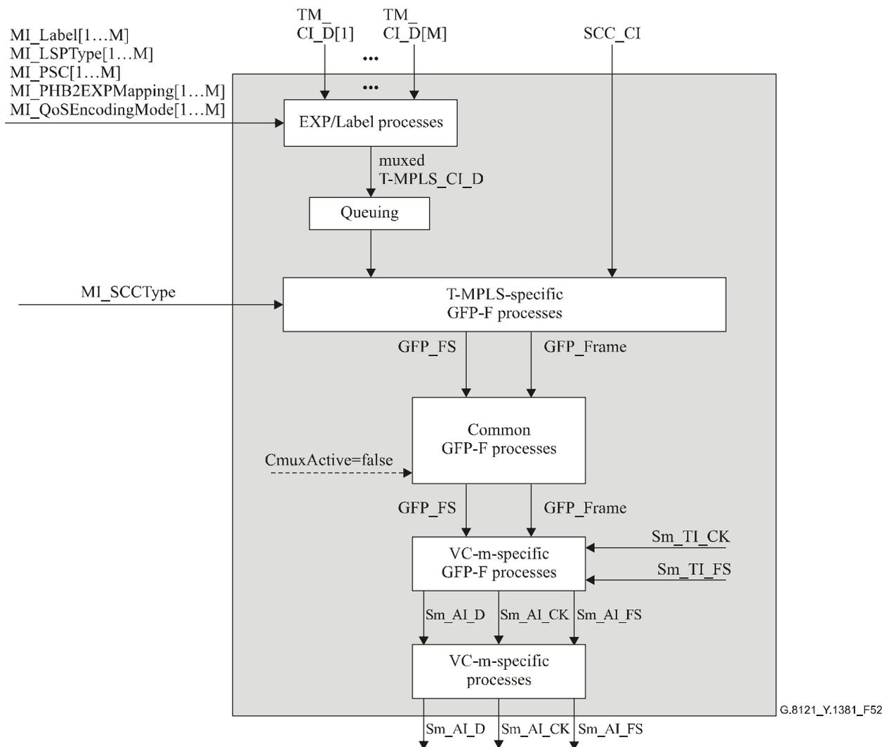
**Figure 52/G.8121/Y.1381 – Sm/TM\_A\_So process diagram**
