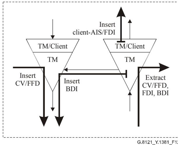
**Figure 12/G.8121/Y.1381 – T-MPLS OAM insertion and extraction in MPLS path endpoint**
