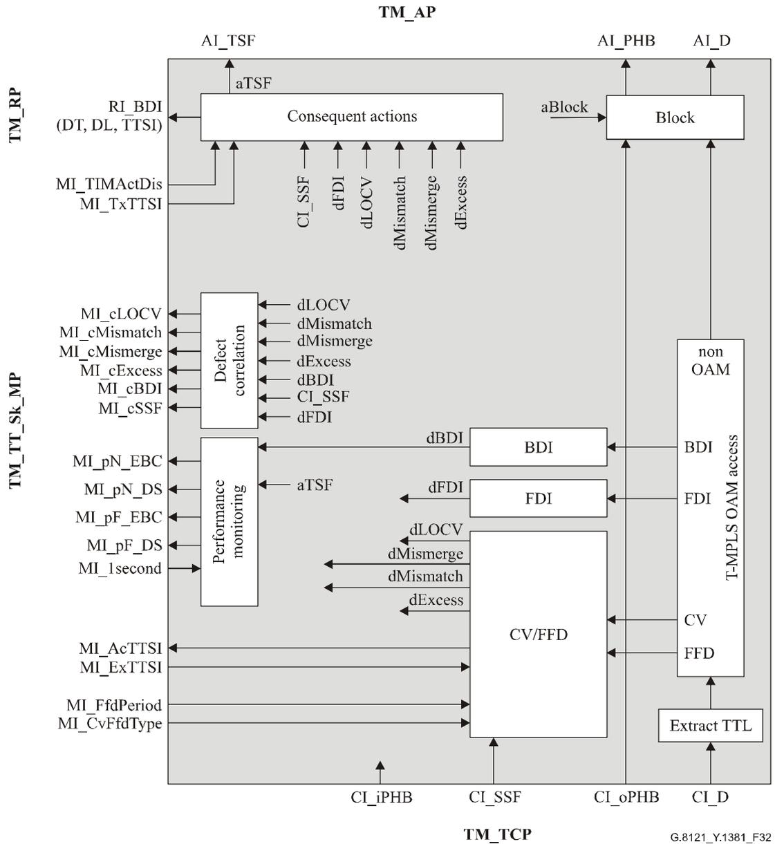
Figure 32/G.8121/Y.1381 – TM\_TT\_Sk process diagram
