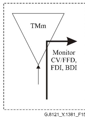
**Figure 15/G.8121/Y.1381 – T-MPLS OAM monitoring in T-MPLS NIM**
