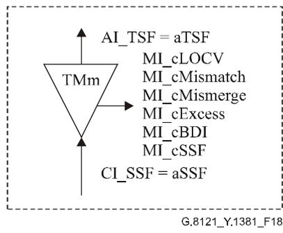
**Figure 18/G.8121/Y.1381 – Fault Management in T-MPLS non-intrusive monitor function**
