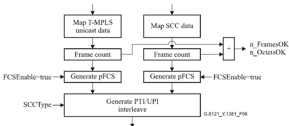
Figure 6/G.8121/Y.1381 – T-MPLS-specific GFP-F source process
