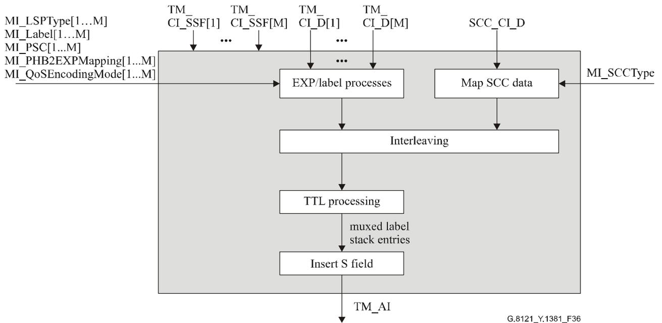
**Figure 36/G.8121/Y.1381 – TM/TM\_A\_So process diagram**
