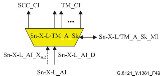
**Figure 49/G.8121/Y.1381 – Sn-X-L/TM\_A\_Sk symbol**
