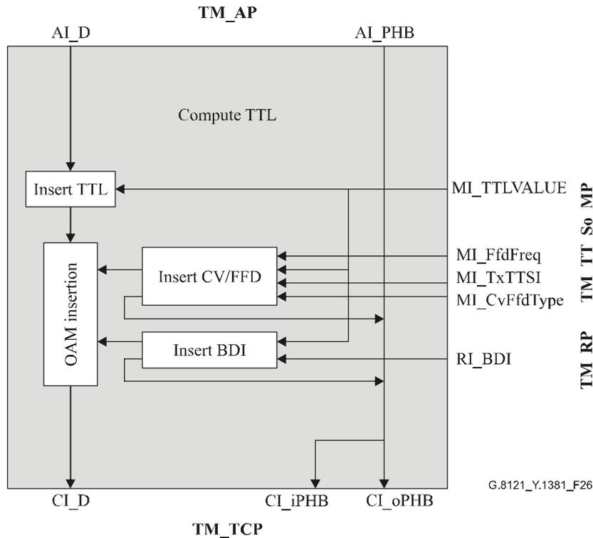
**Figure 26/G.8121/Y.1381 – TM\_TT\_So process diagram**
