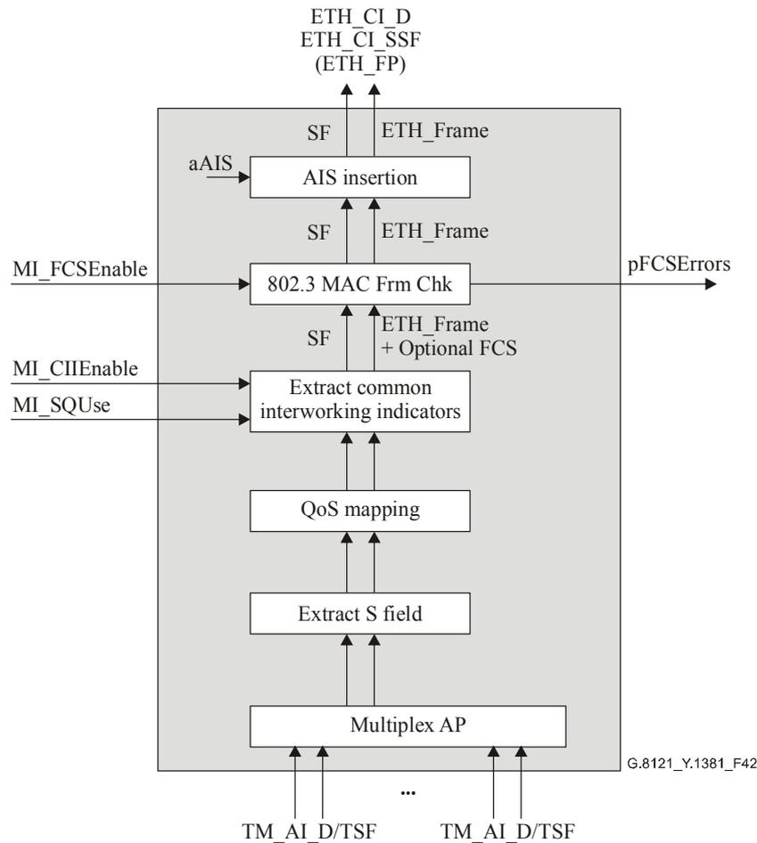
**Figure 42/G.8121/Y.1381 – TM/ETH\_A\_Sk process diagram**
