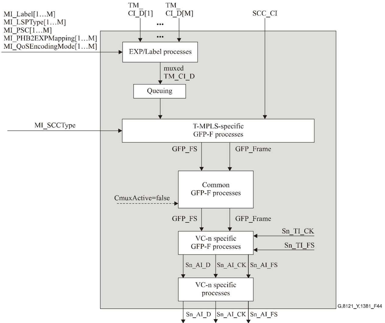
**Figure 44/G.8121/Y.1381 – Sn/TM\_A\_So process diagram**
