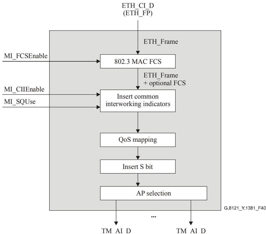
**Figure 40/G.8121/Y.1381 – TM/ETH\_A\_So process diagram**
