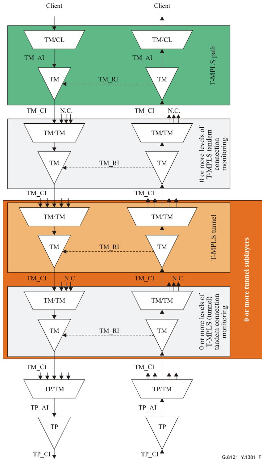
**Figure 11/G.8121/Y.1381 – T-MPLS sublayer stacking example**
