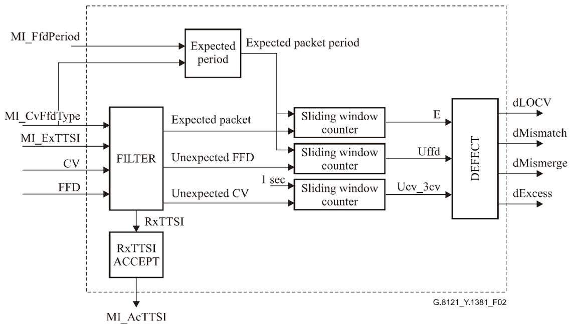
**Figure 2/G.8121/Y.1381 – CV/FFD process block diagram**
