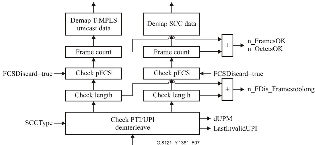
Figure 7/G.8121/Y.1381 – T-MPLS-specific GFP-F sink process
