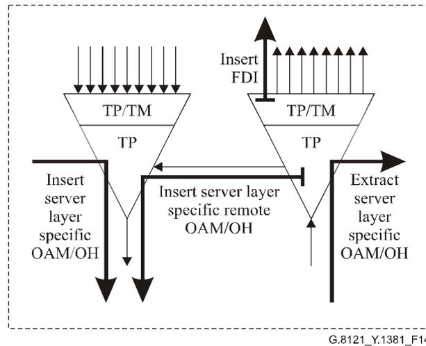
**Figure 14/G.8121/Y.1381 – T-MPLS OAM insertion and extraction in T-MPLS server layer endpoint**
