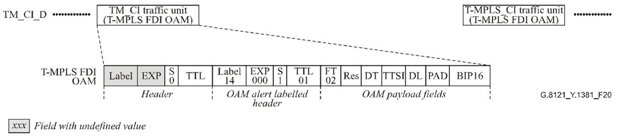
**Figure 20/G.8121/Y.1381 – T-MPLS Characteristic Information Data (TM\_CI\_D) downstream of Signal Fail location**
