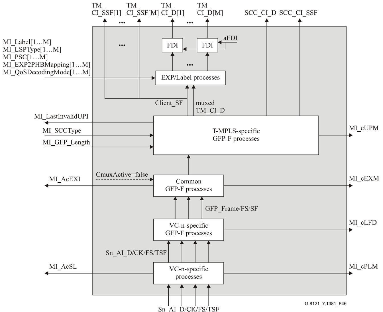
**Figure 46/G.8121/Y.1381 – Sn/TM\_A\_Sk process diagram**
