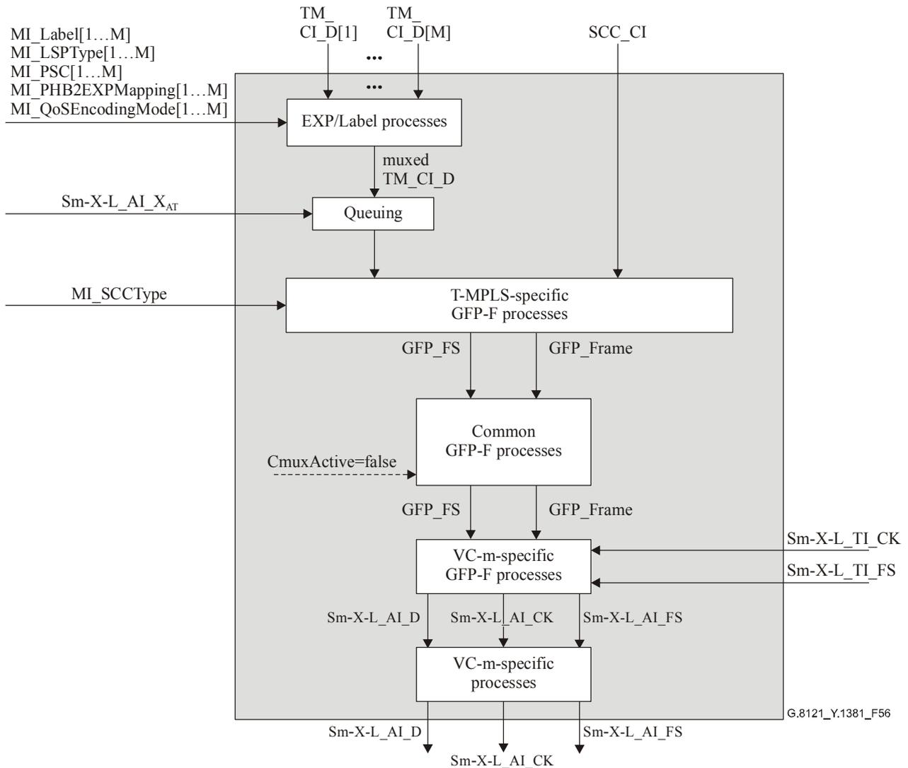
**Figure 56/G.8121/Y.1381 – Sm-X-L/TM\_A\_So process diagram**
