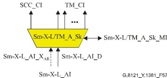
Figure 57/G.8121/Y.1381 – Sm-X-L/TM\_A\_Sk symbol
