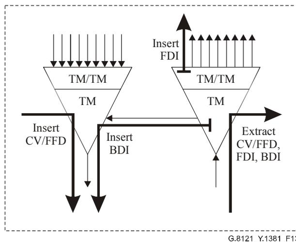
**Figure 13/G.8121/Y.1381 – T-MPLS OAM insertion and extraction in T-MPLS tunnel endpoint**
