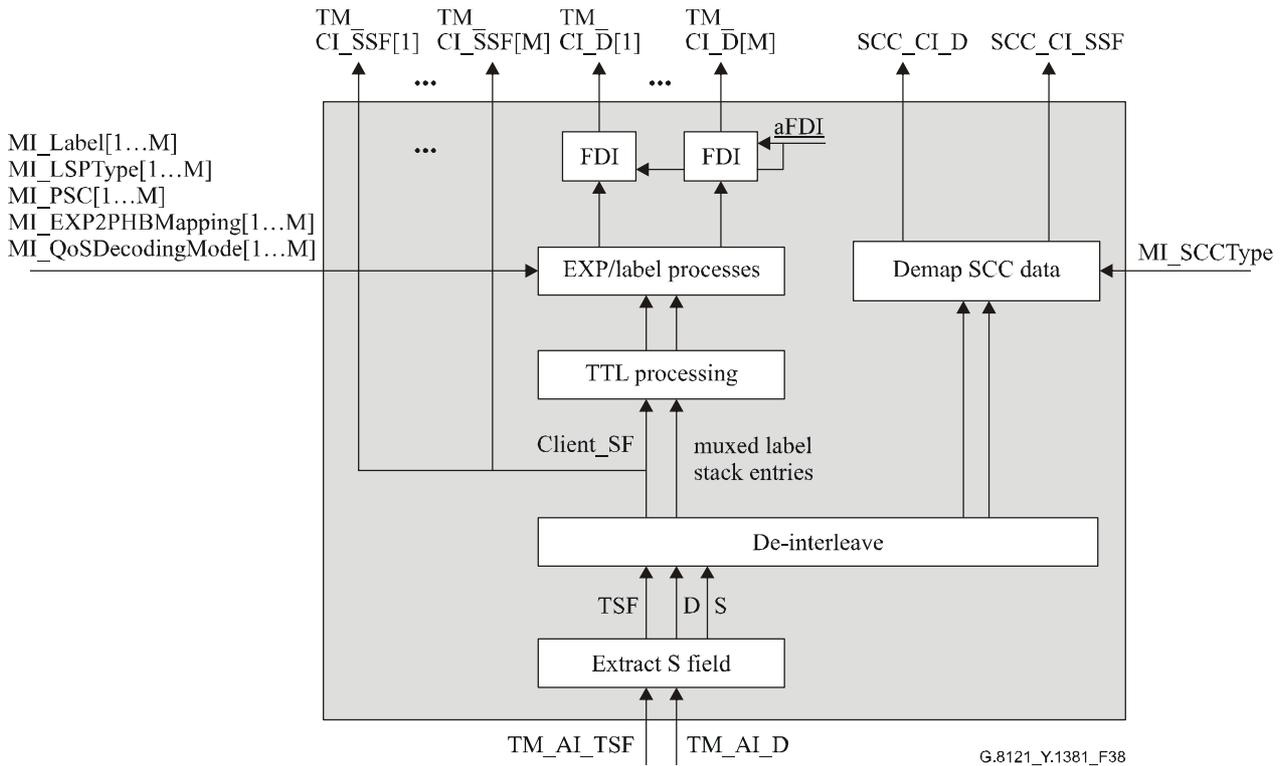
**Figure 38/G.8121/Y.1381 – TM/TM\_A\_Sk process diagram**
