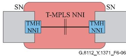
**Figure 6-6 – T-MPLS NNI between service nodes**
