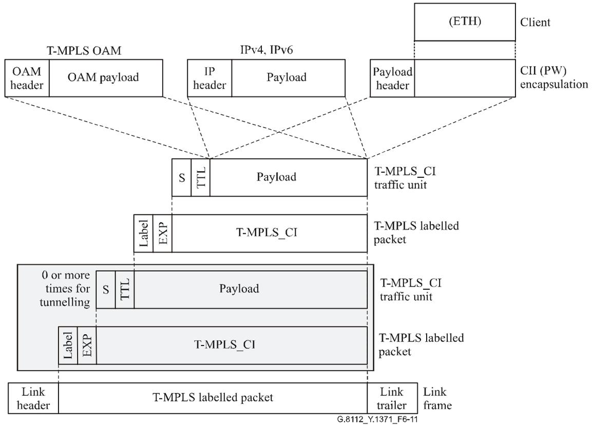
**Figure 6-11 – T-MPLS principle information containment**
