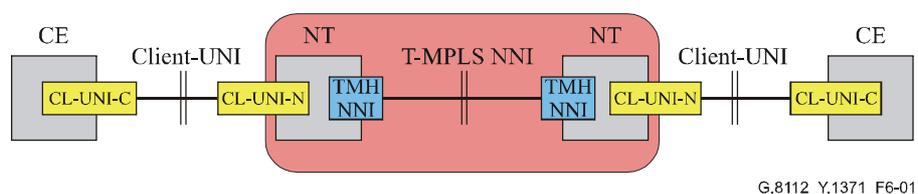
**Figure 6-1 – Locations of Ethernet client-UNI and T-MPLS NNI**
