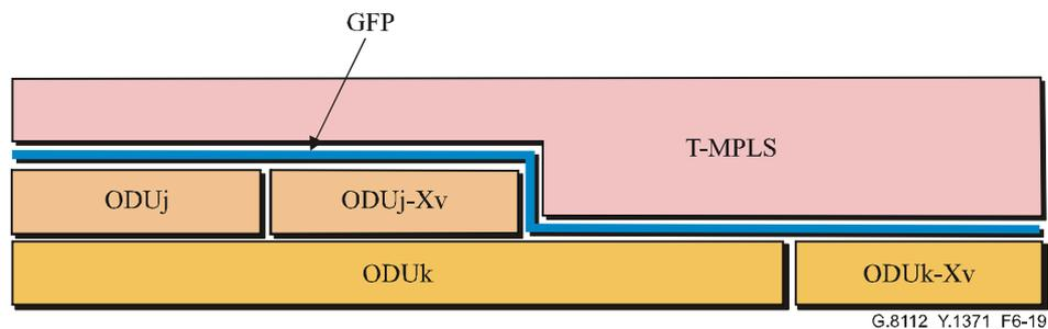
Figure 6-19 – Components of the T-MPLS over OTH NNI
