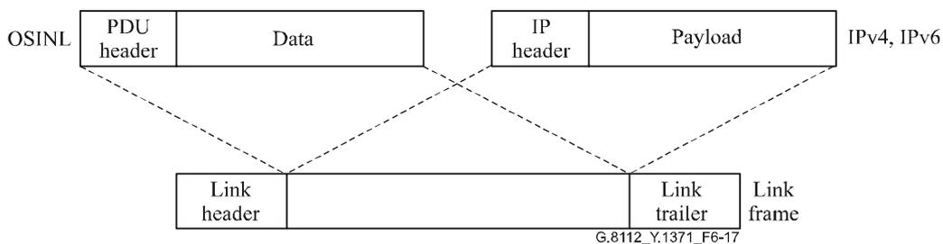
**Figure 6-17 – T-MPLS control frame over shared trail SCN links**
