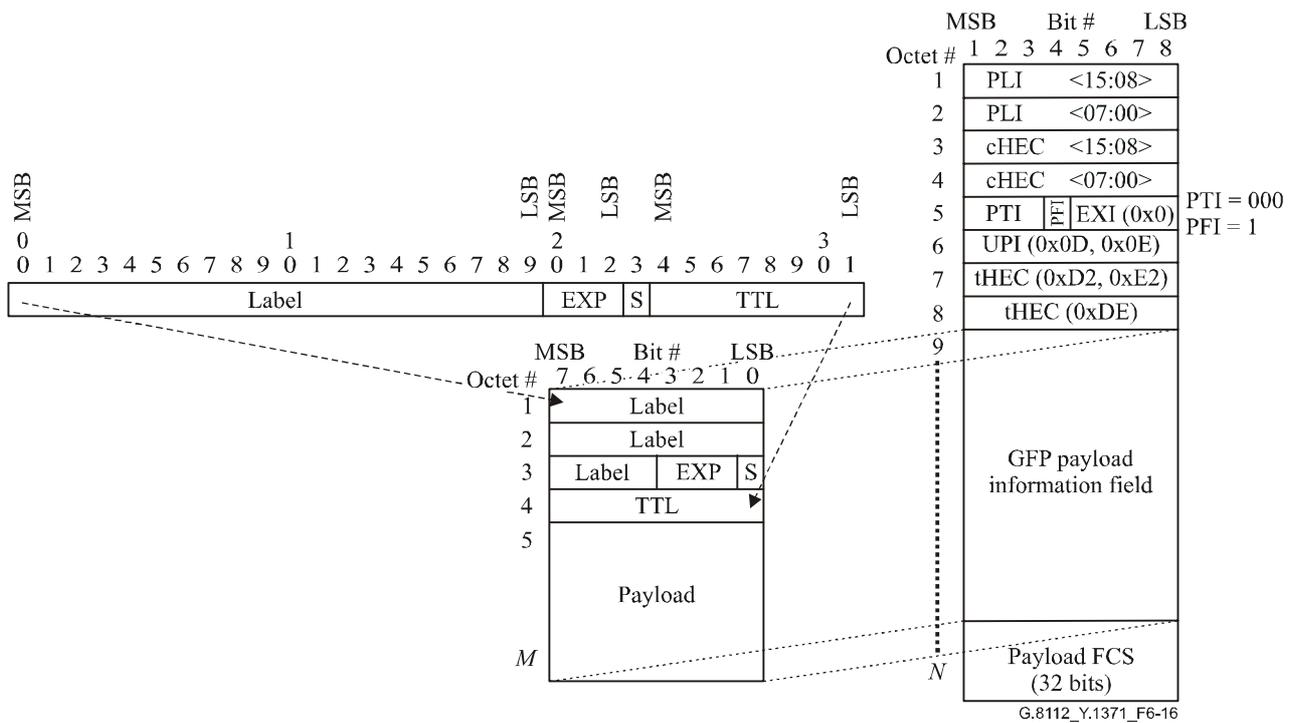
**Figure 6-16 – Mapping T-MPLS labelled packet into GFP-F link frame**
