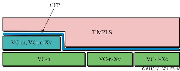
Figure 6-18 – Components of the T-MPLS over SDH NNI using GFP-F encapsulation
