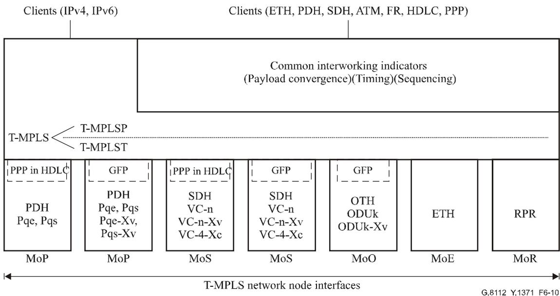
**Figure 6-10 – Structure of the T-MPLS network node interfaces**
