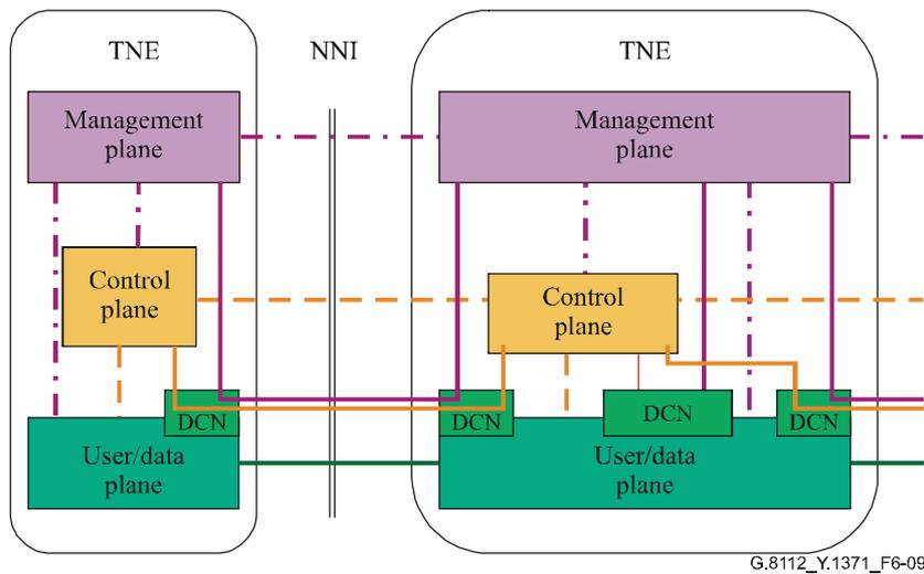
**Figure 6-9 – Three planes of T-MPLS NNI**
