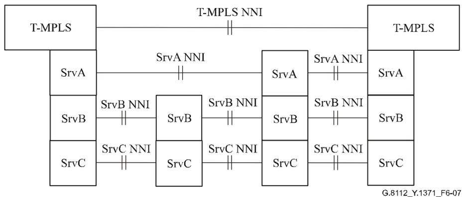
**Figure 6-7 – Example of layer networks in T-MPLS NNI in case of interconnecting two T-MPLS layer service nodes**
