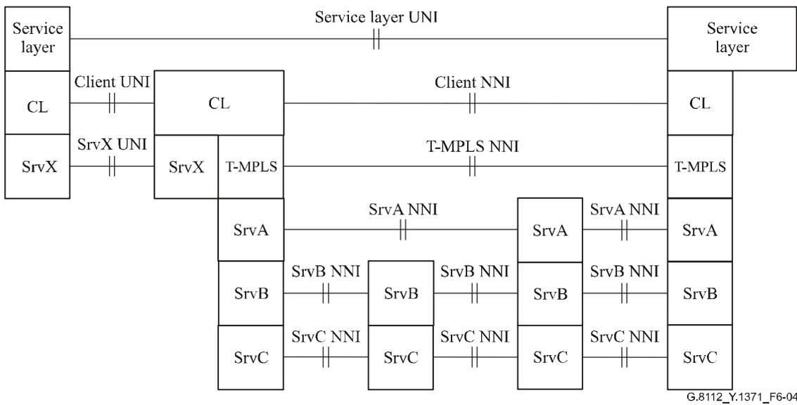
**Figure 6-4 – Example of layer networks in client UNI and T-MPLS NNI in case of access link to a client's layer service node**
