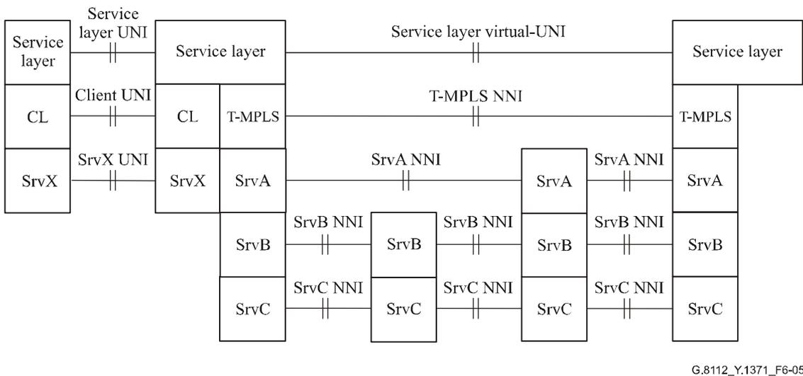
**Figure 6-5 – Example of layer networks in service layer UNI and T-MPLS NNI supporting an extended service layer UNI (virtual UNI) to a service node**
