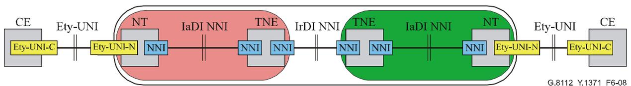
**Figure 6-8 – Locations of T-MPLS NNI in a multi-operator network**
