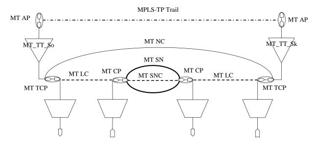
Figure 6-4 – MPLS-TP layer network example
