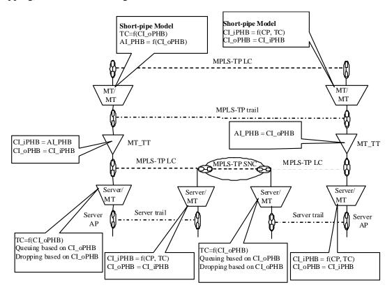
Figure 10-1 – Reference diagram for the short-pipe model
