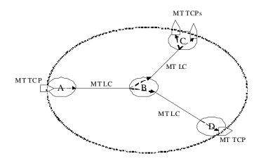
Figure 6-8 – MPLS-TP p2mp network connection using MPLS-TP p2p link connections
