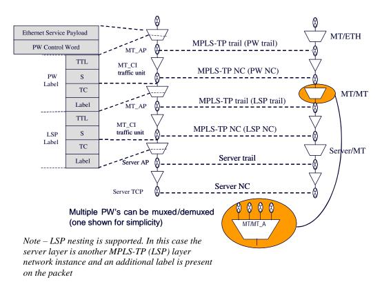
Figure 6-5 – MPLS-TP layer network structure example
