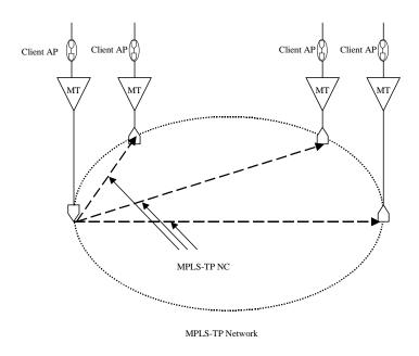
Figure 6-7 – Point-to-multipoint MPLS-TP connection
