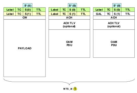
$<sup>^{\</sup>star}$ ) The MTS label stack entry fields are removed by the physical media adaptation so urce function
