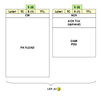
Figure I.3 – MPLS-TP network adapted and characteristic information traffic units (reference point 3)
