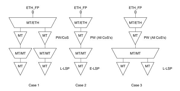
Figure 6-6 – Examples of QoS processing in MT/Client A function
