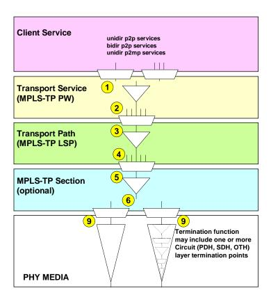
Figure I.1 – MPLS-TP network architecture (layer view) example
