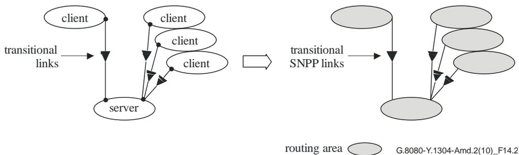
**Figure 14-2 – Multilayer routing topology representation of Figure 14**
