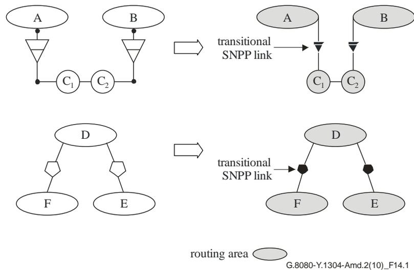
**Figure 14-1 – Multilayer routing topology representations**
