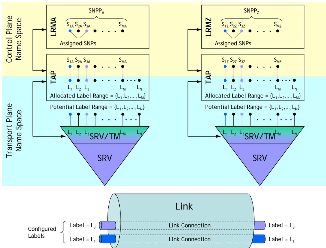
**Figure 33.2 – Control plane and transport plane link resource model**
