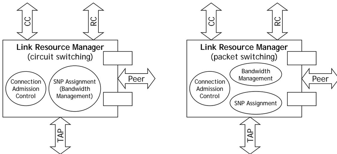
**Figure 23.1 – Basic LRM functions for circuit switching and packet switching**
