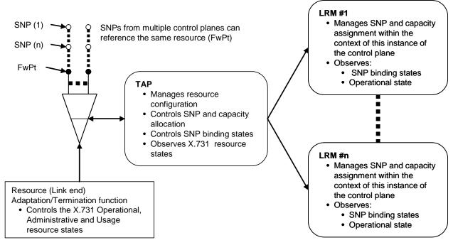
FwPt (Forwarding Port) – The (unbound) end of a link connection. It is converted into a FwP (Forwarding Point) when it is bound to a subnetwork connection. The binding does not change the resource label.
