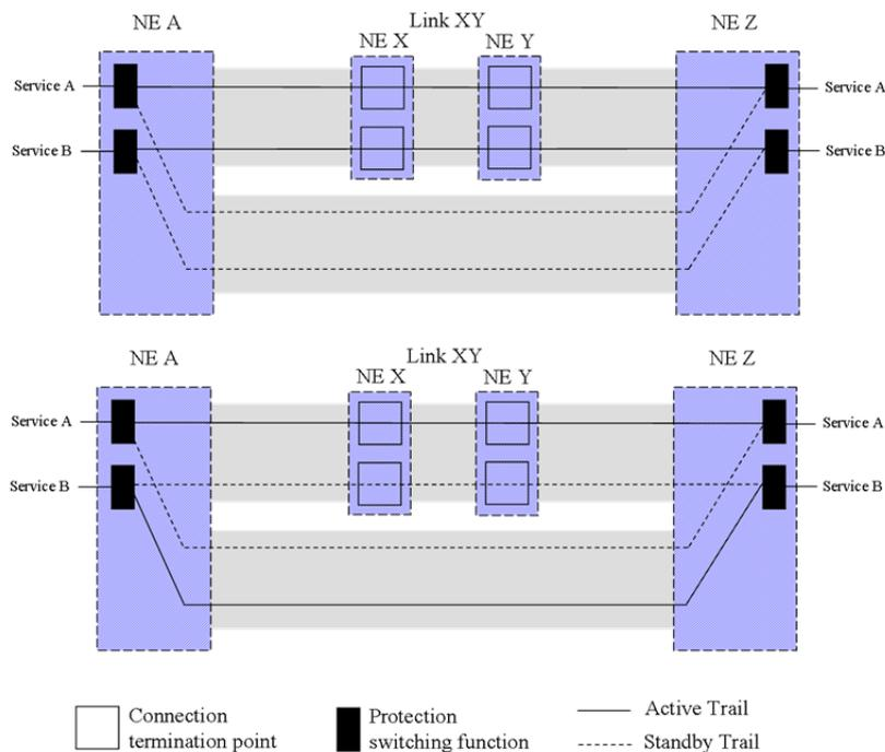
**Figure VII.1 – Load sharing in a dynamic bandwidth network**
