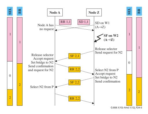
Figure 24-5 – 3-phase protocol example (multiple failures)
