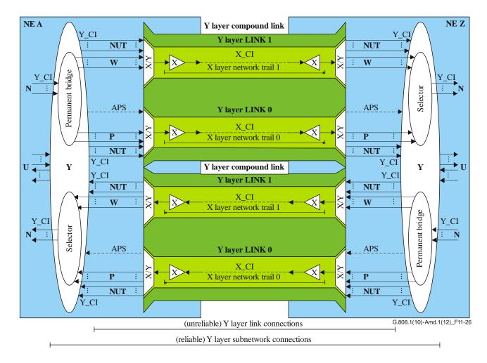
$Figure \ 11\text{-}26-1\text{+}1\ compound\ link\ subnetwork\ connection\ group\ protection}$  with inherent monitoring (CL-SNCG/I) functional model
