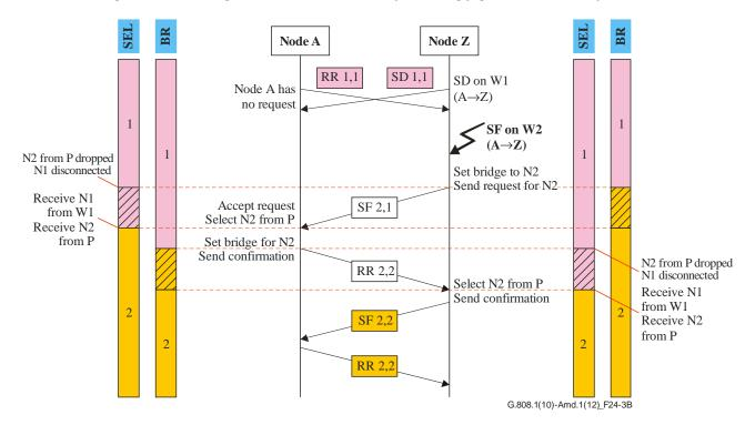
Figure 24-3B – 2-phase protocol example for (1:1)<sup>n</sup> architecture (multiple failures)
