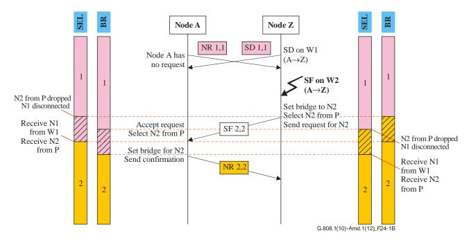
Figure 24-1B – 1-phase protocol example for (1:1)<sup>n</sup> architecture (multiple failures)
