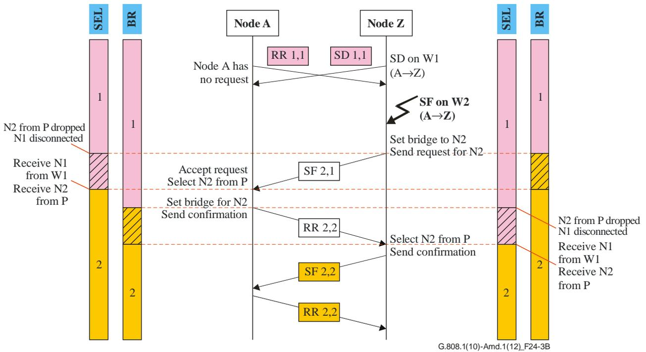
**Figure 24-3B – 2-phase protocol example for (1:1)<sup>n</sup> architecture (multiple failures)**
