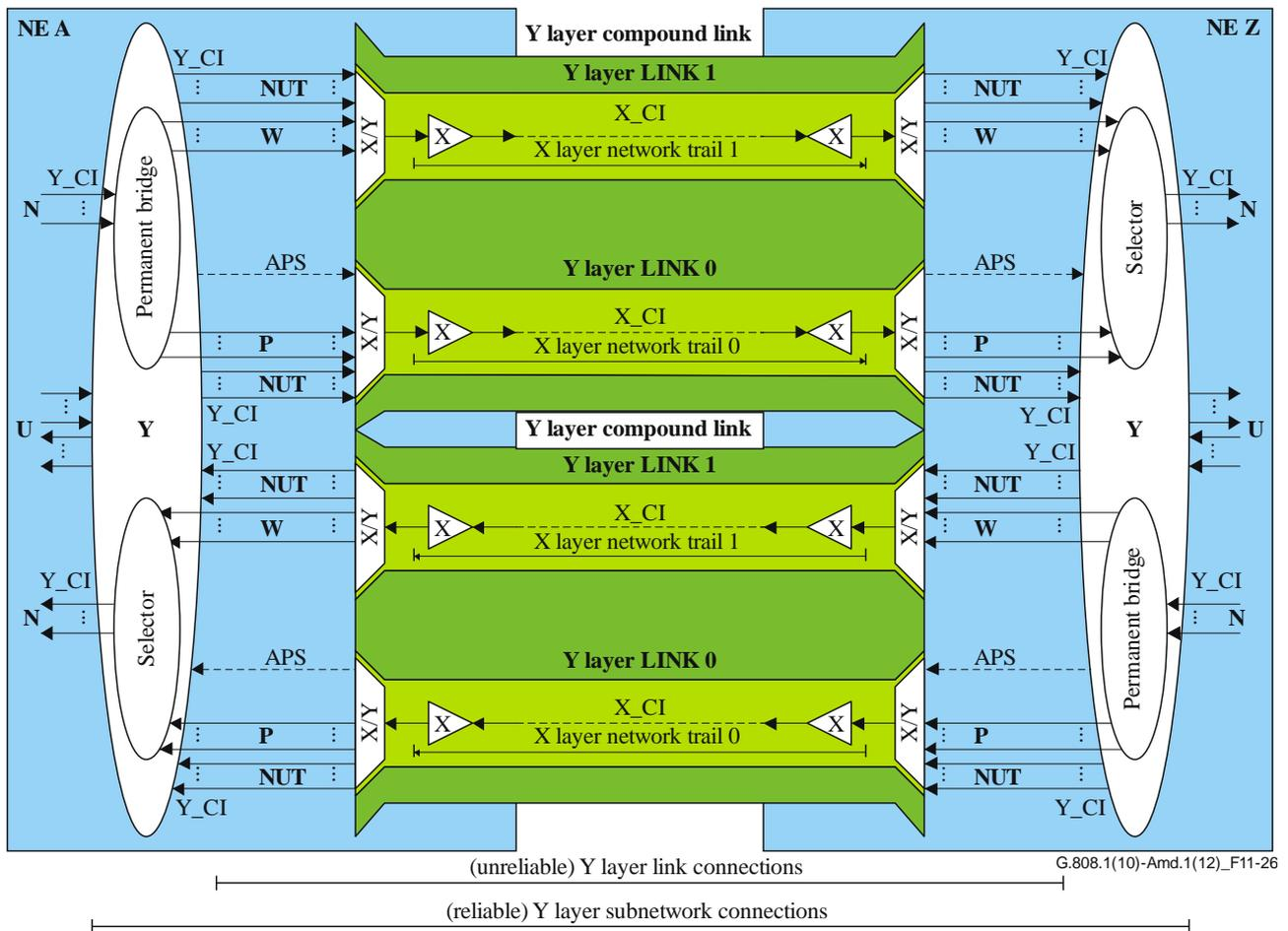
**Figure 11-26 – 1+1 compound link subnetwork connection group protection with inherent monitoring (CL-SNCG/I) functional model**
