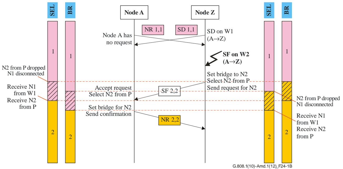
**Figure 24-1B – 1-phase protocol example for (1:1)<sup>n</sup> architecture (multiple failures)**
