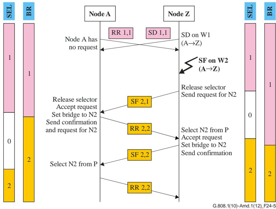
**Figure 24-5 – 3-phase protocol example (multiple failures)**
