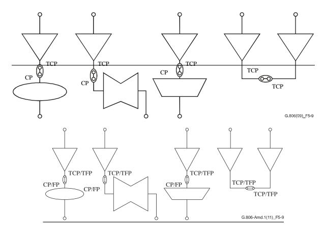
Figure 5-9 – Binding involving a termination of connection<u>/flow</u> points (TCP-CP<u>/TFP-FP</u> and TCP-TCP<u>/TFP-FP</u> binding)
