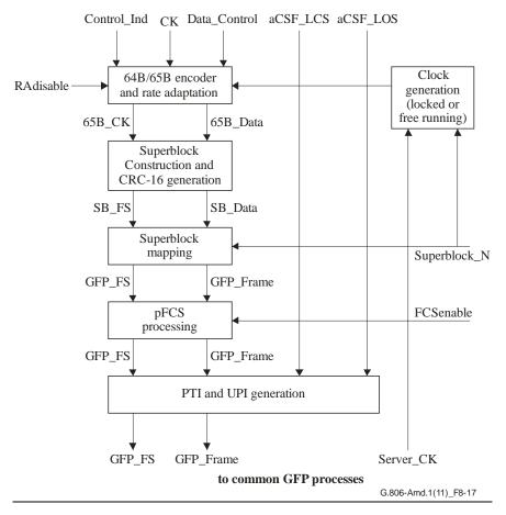
Figure 8-17 – Client-specific GFP-T source processes
