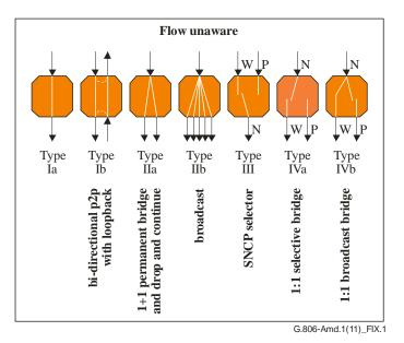
Figure IX.1 – Basic flow unaware forwarding process types
