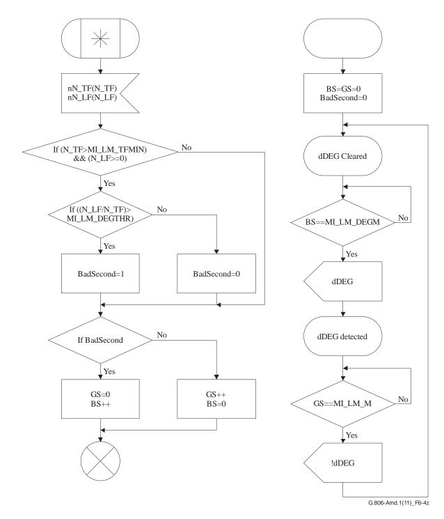
Figure 6-4z – dDEG detection and clearance process
