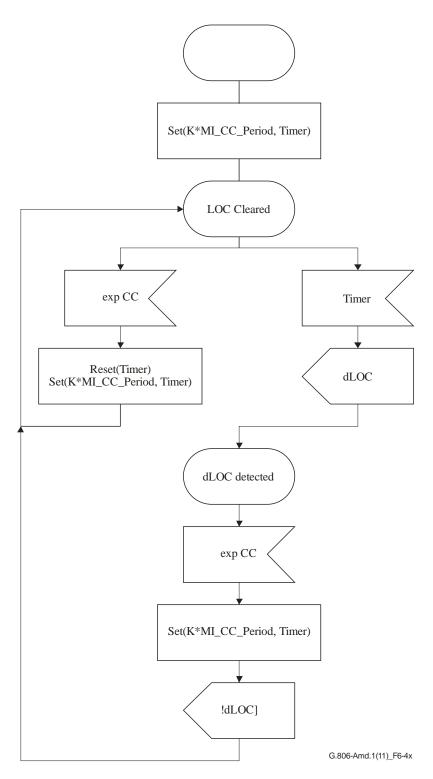
Figure 6-4x – dLOC detection and clearance process
