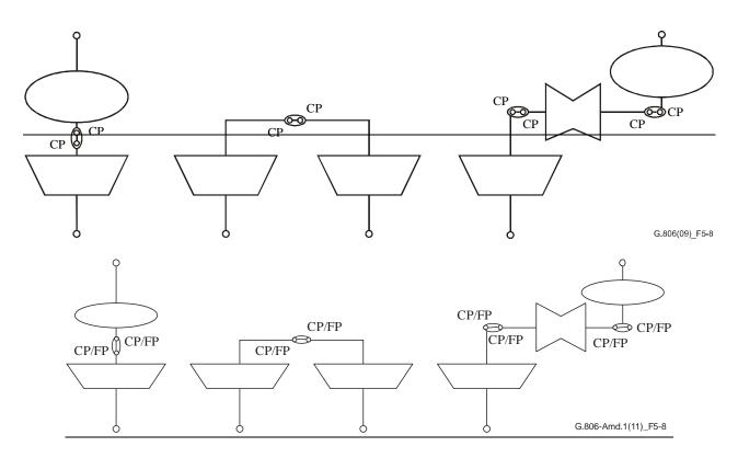
Figure 5-8 – Binding of connection<u>/flow</u> points (CP-CP binding)
