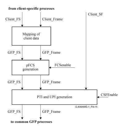
Figure 8-15/G.806 – Client-specific GFP-F source processes
