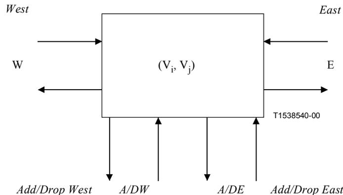
**Figure I.4/G.806 – Connection matrix example for 4-port groups**
