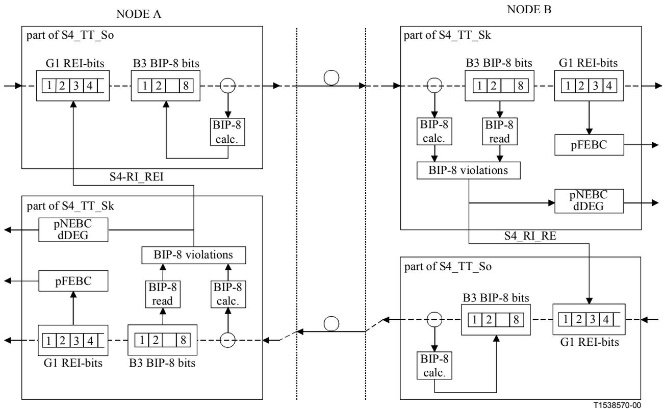
Figure II.3/G.806 – REI insertion control example (VC-4 path)
