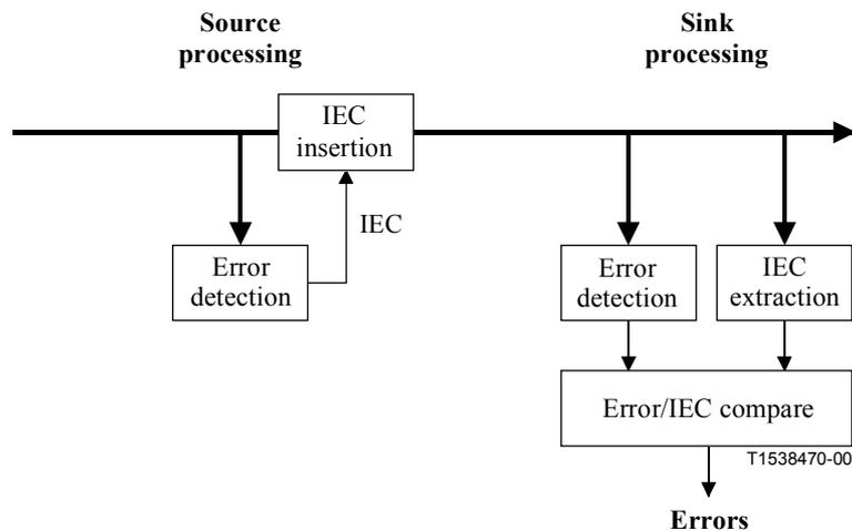
**Figure 8-6/G.806 – IEC based signal quality supervision**
