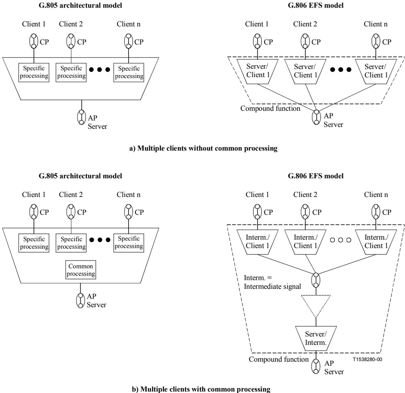
**Figure 5-6/G.806 – Comparison with ITU-T G.805 [11] multiplexing model**
