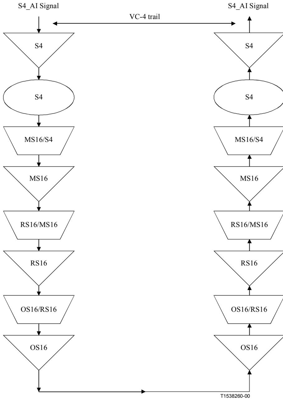
**Figure 5-4/G.806 – Example of a unidirectional VC-4 path in an SDH network**
