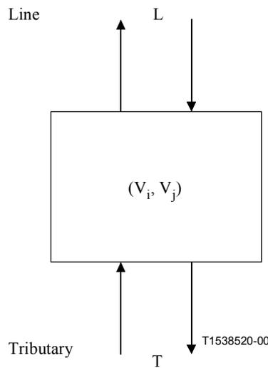
**Figure I.2/G.806 – Connection matrix example for 2-port groups**
