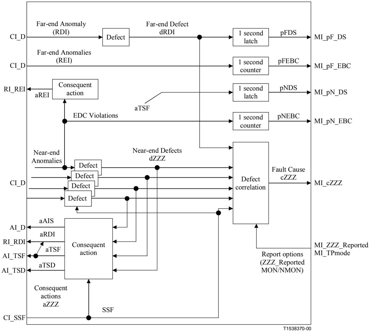
Figure 6-1/G.806 – Supervision process within trail termination functions
