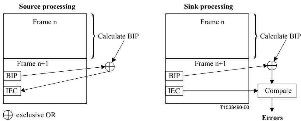
**Figure 8-7/G.806 – IEC based signal quality supervision example**
