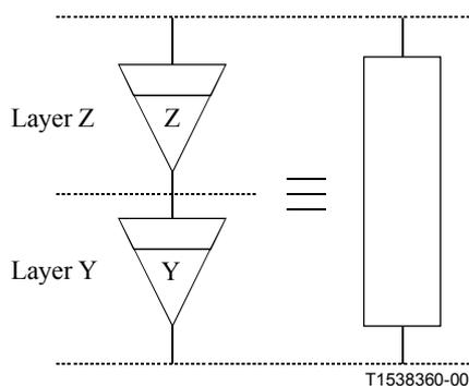
**Figure 5-14/G.806 – Compound function spanning multiple layers**
