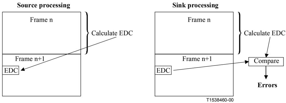
**Figure 8-5/G.806 – Signature based signal quality supervision example**
