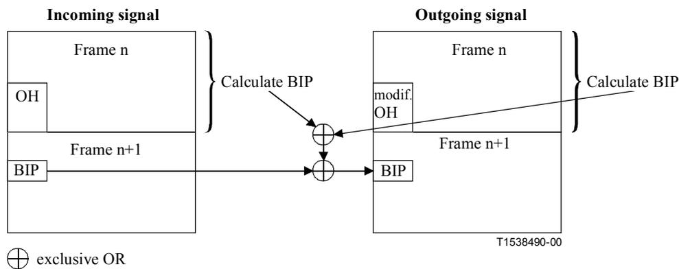
**Figure 8-8/G.806 – BIP correction; functionality**
