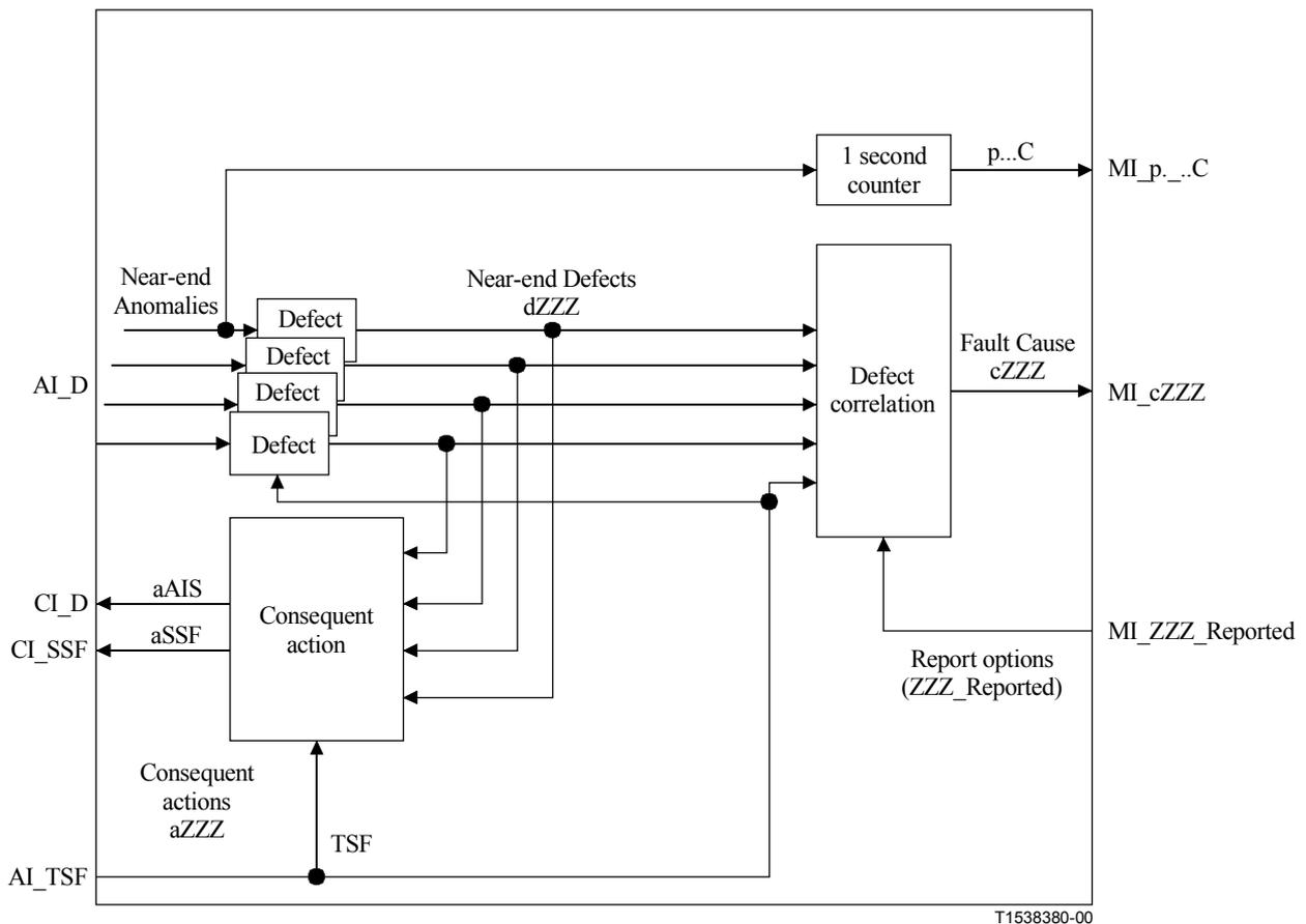
**Figure 6-2/G.806 – Supervision process within adaptation functions**
