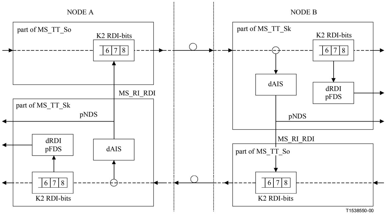
Figure II.1/G.806 – RDI insertion control example (multiplex section)
