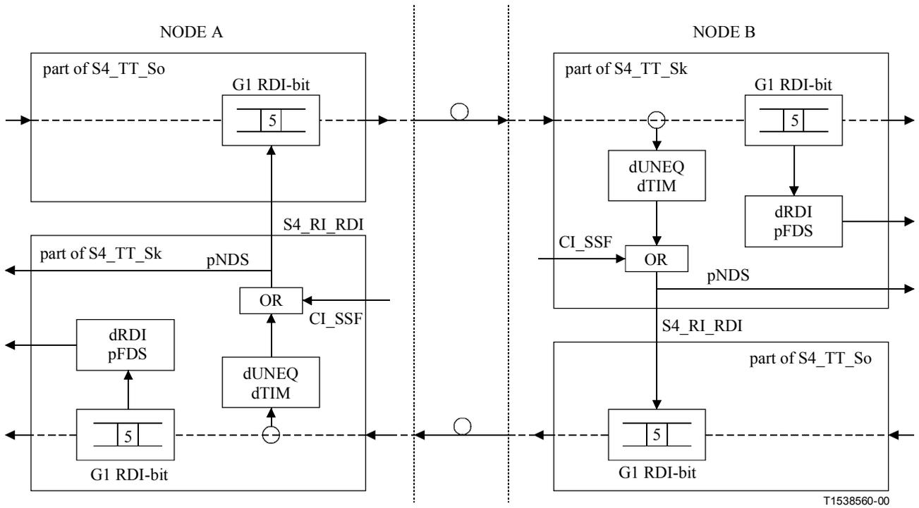
Figure II.2/G.806 – RDI insertion control example (VC-4 path)
