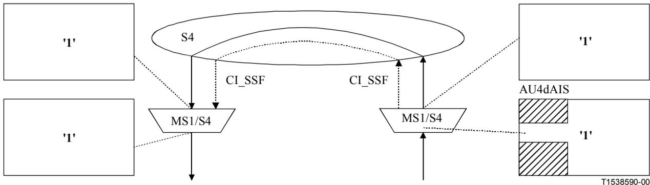
**Figure III.2/G.806 – All-ONES propagation from sink to source direction**
