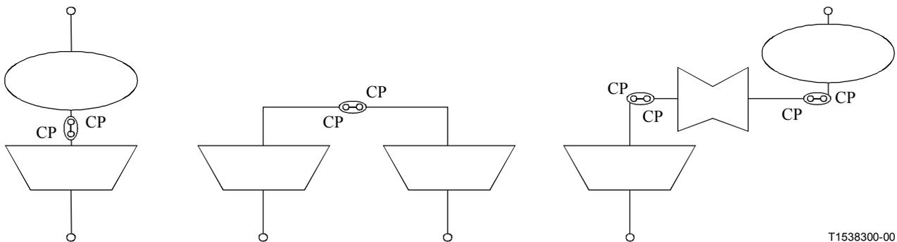
Figure 5-8/G.806 – Binding of connection points (CP-CP binding)
