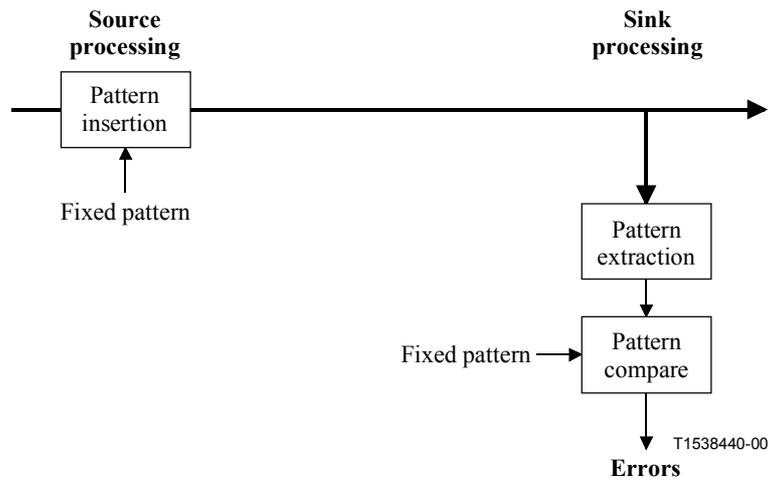
**Figure 8-3/G.806 – Pattern based signal quality supervision**
