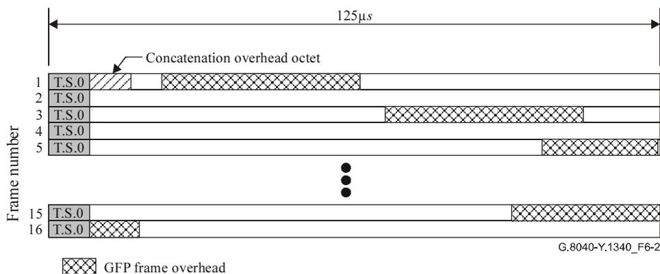
Figure 6-2/G.8040/Y.1340 – Octet-aligned mapping for GFP into the 2048 kbit/s signal
