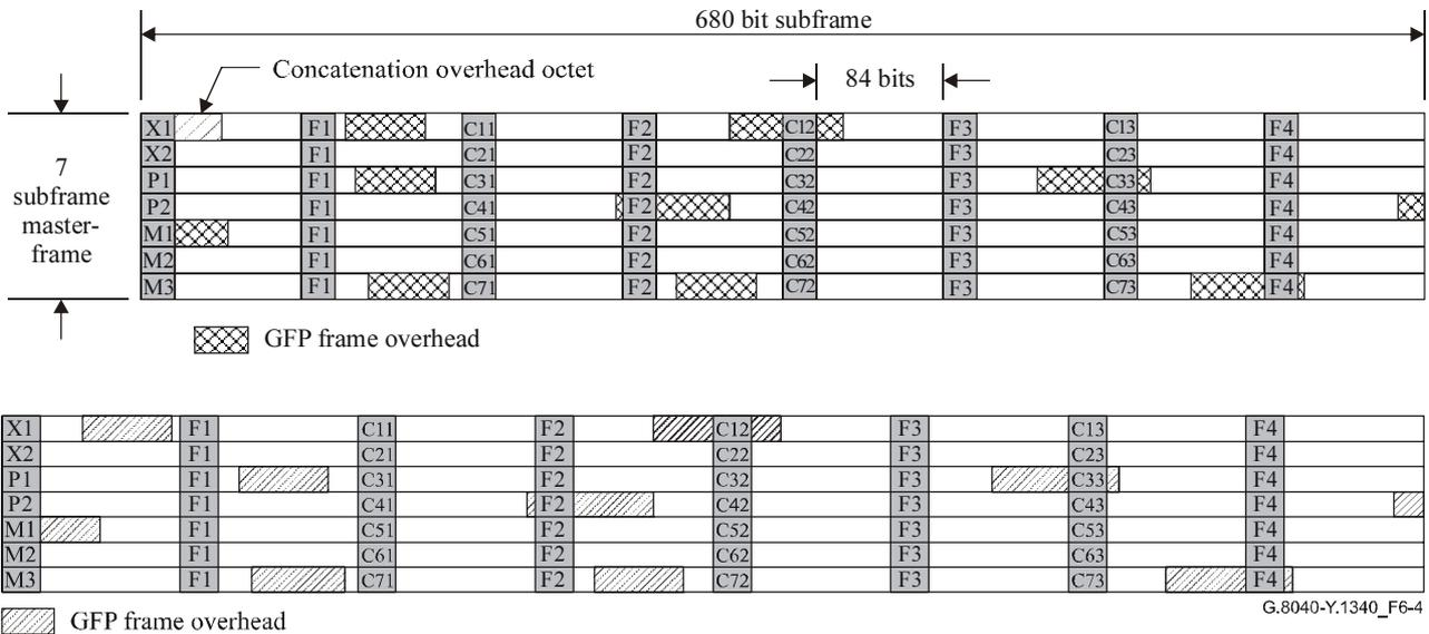
**Figure 6-4/G.8040/Y.1340 – GFP mapping into a 44 736 kbit/s signal frame**
