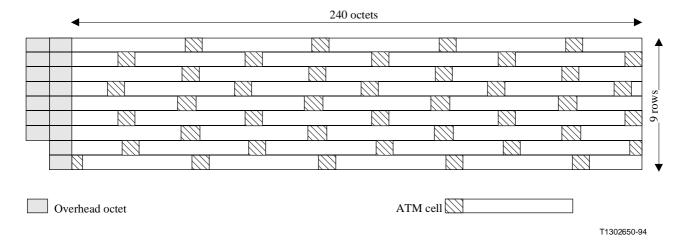
Figure 9-1/G.804 – Frame structure at 139 264 kbit/s
