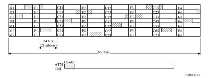
Figure 7-3/G.804 – Frame structure for 44 736 kbit/s used to transport ATM cells
