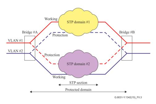
Figure II.3 – Overlapping between the protected domain and STP per VLAN
