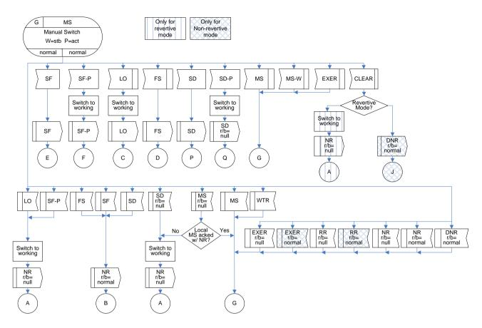
Figure IV.7 – MS(r/b=normal) state for 1:1 bidirectional protection switching
