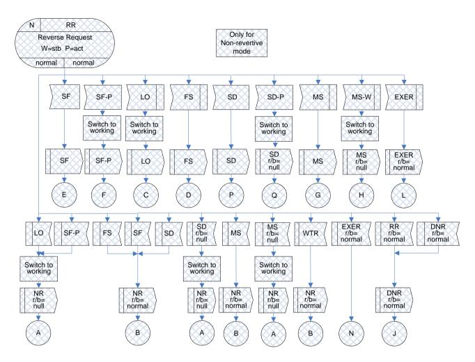
Figure IV.14 – RR(r/b=normal) state for 1:1 bidirectional protection switching
