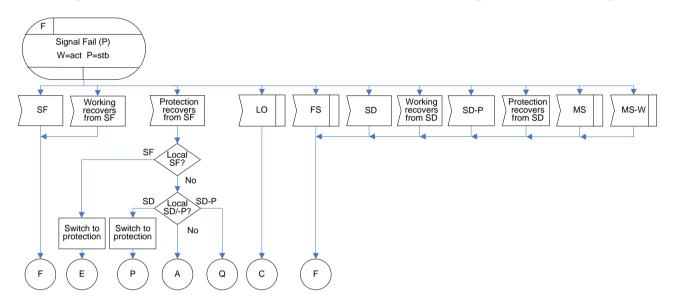
Figure IV.37 – SF-P(W=act/P=stb) state for 1+1 unidirectional protection switching
