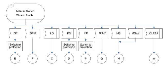
Figure IV.39 – MS(W=act/P=stb) state for 1+1 unidirectional protection switching
