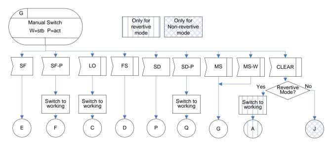
Figure IV.38 – MS(W=stb/P=act) state for 1+1 unidirectional protection switching
