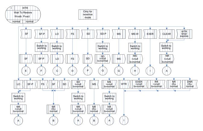
Figure IV.25 – WTR(r/b=normal) state for 1+1 bidirectional protection switching
