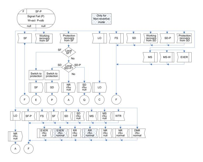
Figure IV.6 – SF-P(r/b=null) state for 1:1 bidirectional protection switching
