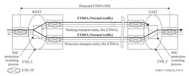
$Figure \ 10\text{-}11-1\text{:}1\ protection\ switching\ architecture\ (with\ broadcast\ bridge)}-Signal\ degrade\\ condition\ for\ working\ transport\ entity$
