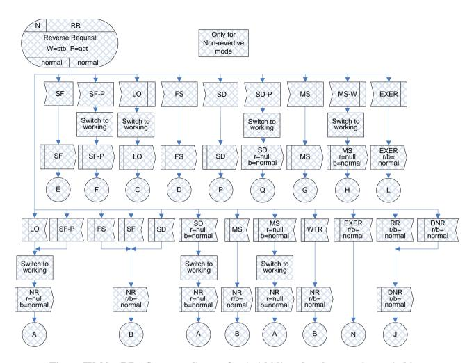
Figure IV.30 – RR(r/b=normal) state for 1+1 bidirectional protection switching
