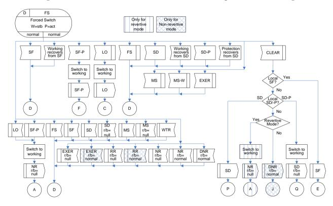
Figure IV.4 – FS(r/b=normal) state for 1:1 bidirectional protection switching
