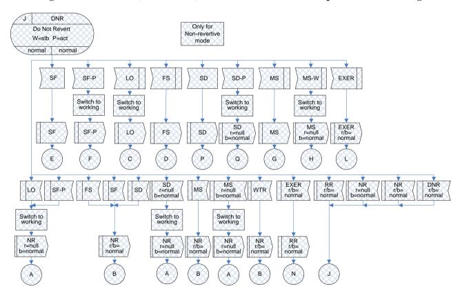
Figure IV.26 – DNR(r/b=normal) state for 1+1 bidirectional protection switching
