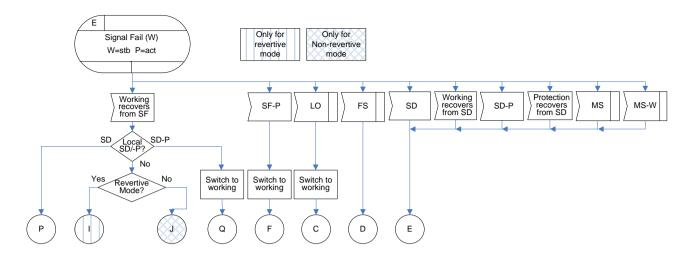
Figure IV.36 – SF(W=stb/P=act) state for 1+1 unidirectional protection switching
