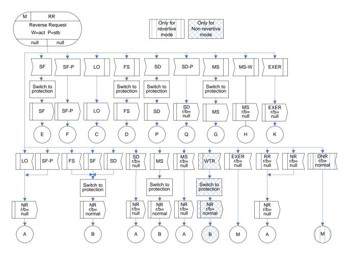
Figure IV.13 – RR(r/b=null) state for 1:1 bidirectional protection switching
