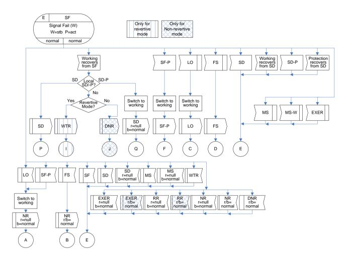
Figure IV.21 – SF(r/b=normal) state for 1+1 bidirectional protection switching
