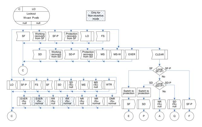
Figure IV.3 – LO(r/b=null) state for 1:1 bidirectional protection switching
