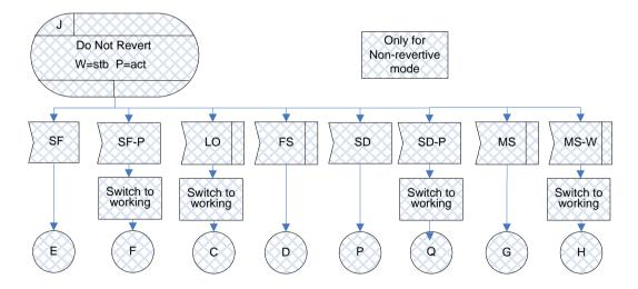
Figure IV.41 – DNR(W=stb/P=act) state for 1+1 unidirectional protection switching
