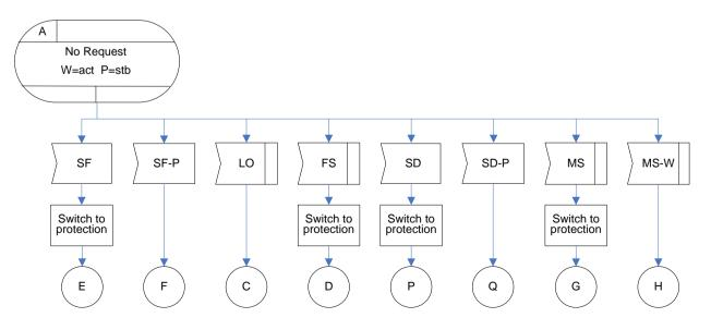
Figure IV.33 – NR(W=act/P=stb) state for 1+1 unidirectional protection switching
