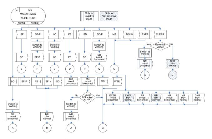
Figure IV.23 – MS(r/b=normal) state for 1+1 bidirectional protection switching
