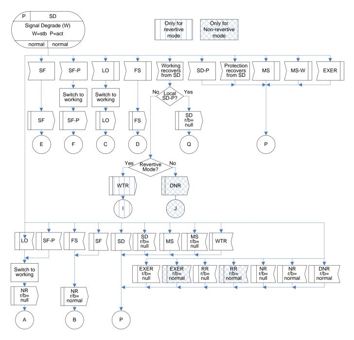
Figure IV.15 – SD(r/b=normal) state for 1:1 bidirectional protection switching
