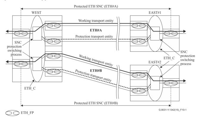
Figure 10-1 – ETH SNC/S protection switching architecture
