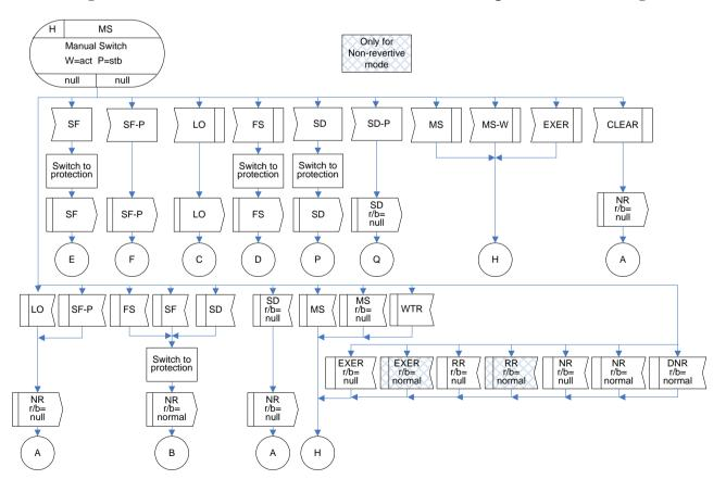
Figure IV.8 – MS(r/b=null) state for 1:1 bidirectional protection switching
