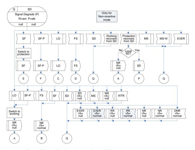
Figure IV.16 – SD(r/b=null) state for 1:1 bidirectional protection switching
