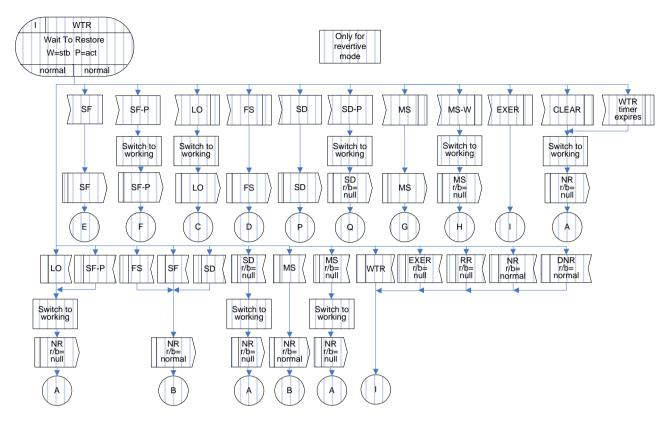
Figure IV.9 – WTR(r/b=normal) state for 1:1 bidirectional protection switching
