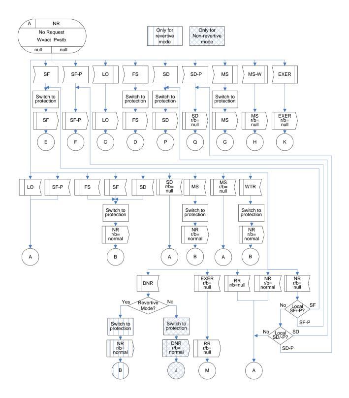
Figure IV.1 – NR(r/b=null) state for 1:1 bidirectional protection switching
