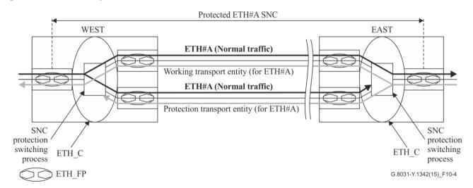
Figure 10-4 – 1+1 bidirectional protection switching architecture
