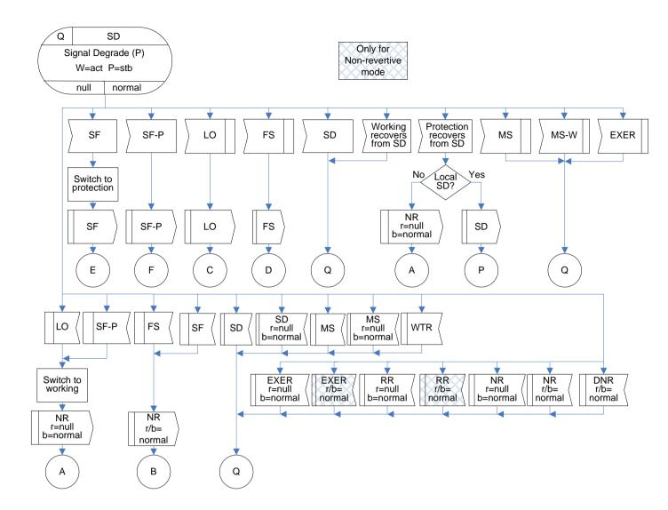
Figure IV.32 – SD(r=null, b=normal) state for 1+1 bidirectional protection switching
