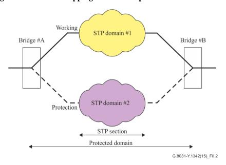
Figure II.2 – Overlapping between the protected domain and STP
