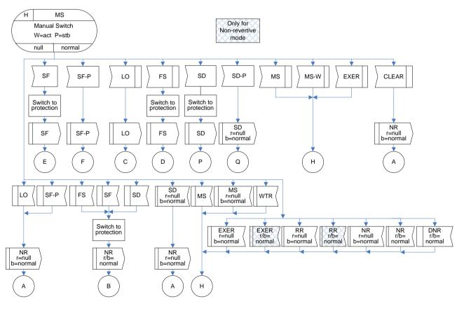
Figure IV.24 – MS(r=null, b=normal) state for 1+1 bidirectional protection switching
