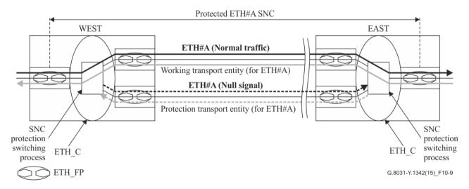
Figure 10-9 – 1:1 protection switching architecture
