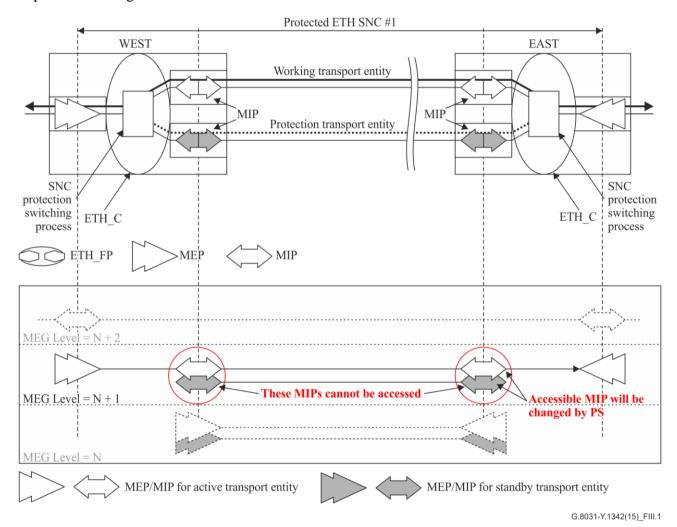
Figure III.1 – MEPs and MIPs for 1:1 bidirectional protection switching
