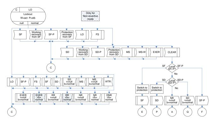
Figure IV.19 – LO(r=null, b=normal) state for 1+1 bidirectional protection switching
