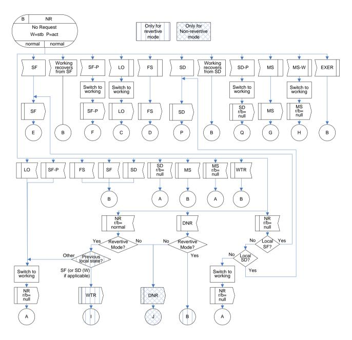
Figure IV.2 – NR(r/b=normal) state for 1:1 bidirectional protection switching
