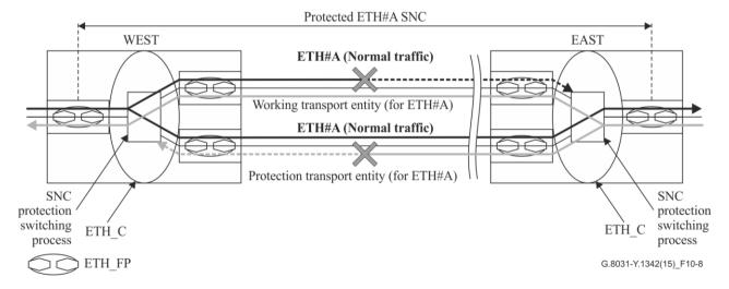
Figure 10-8 – 1+1 unidirectional protection switching architecture – Signal fail (or signal degrade) condition in both directions
