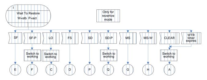
Figure IV.40 – WTR(W=stb/P=act) state for 1+1 unidirectional protection switching
