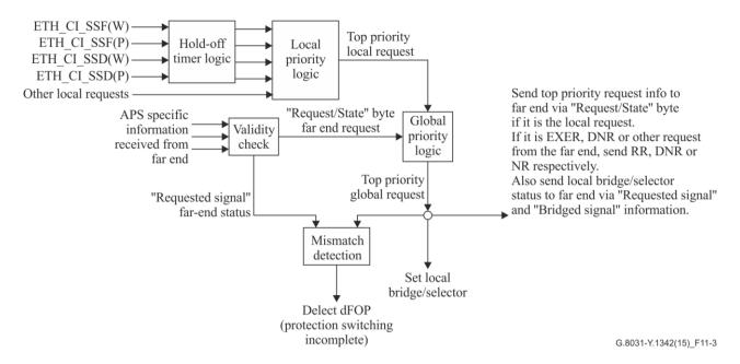
Figure 11-3 – Principle of 1+1/1:1 linear protection switching algorithm
