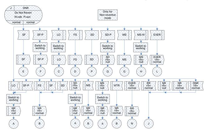
Figure IV.10 – DNR(r/b=normal) state for 1:1 bidirectional protection switching
