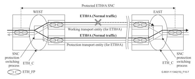
Figure 10-7-1+1 unidirectional protection switching architecture – Signal fail (or signal degrade) condition for working transport entity in the west-to-east direction
