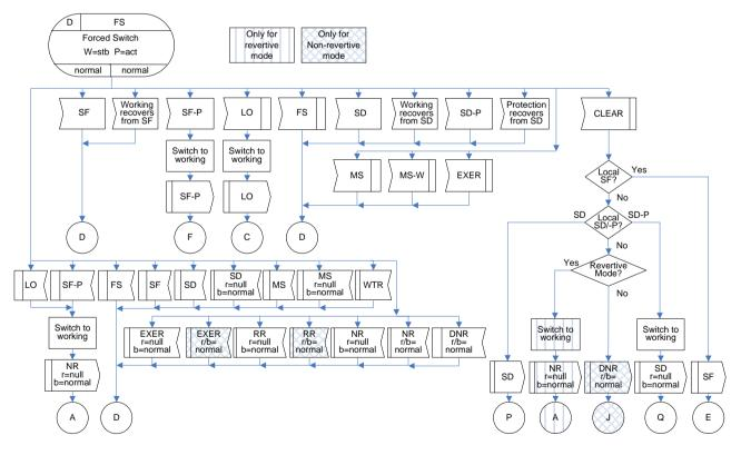
Figure IV.20 – FS(r/b=normal) state for 1+1 bidirectional protection switching
