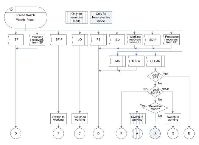
Figure IV.35 – FS(W=stb/P=act) state for 1+1 unidirectional protection switching
