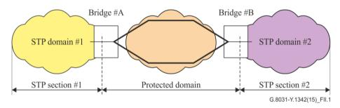
Figure II.1 – No overlapping between the protected domain and STP
