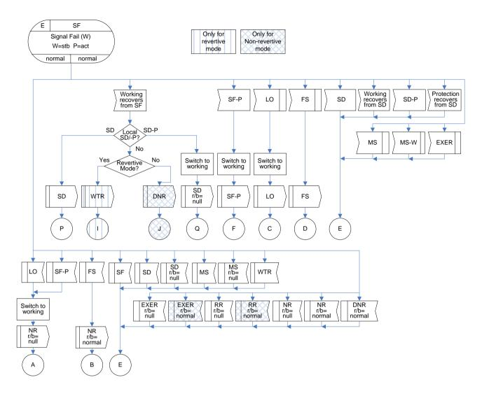
Figure IV.5 – SF(r/b=normal) state for 1:1 bidirectional protection switching
