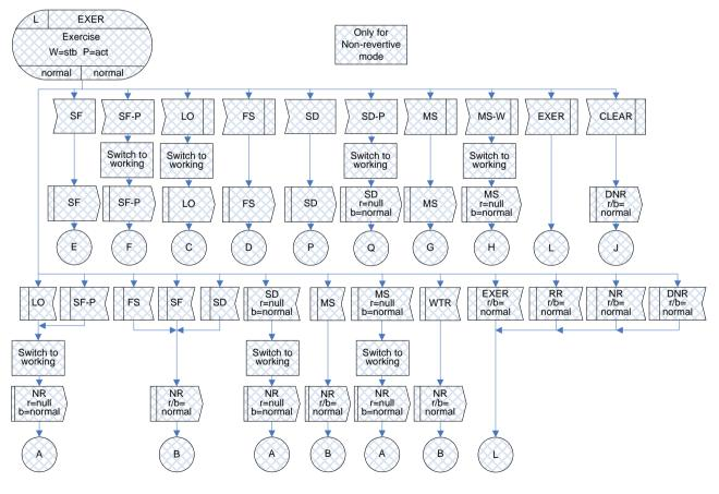
Figure IV.28 – EXER(r/b=normal) state for 1+1 bidirectional protection switching
