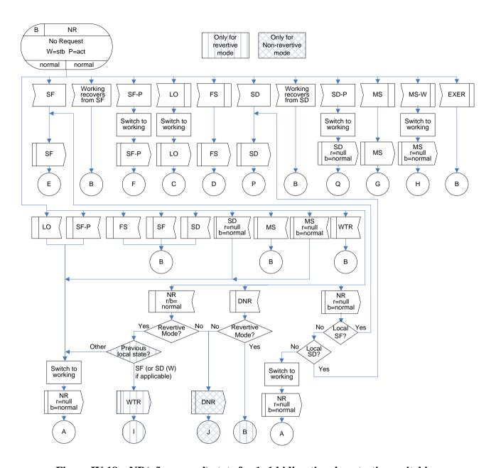
Figure IV.18 – NR(r/b=normal) state for 1+1 bidirectional protection switching
