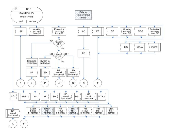
Figure IV.22 – SF-P(r=null, b=normal) state for 1+1 bidirectional protection switching
