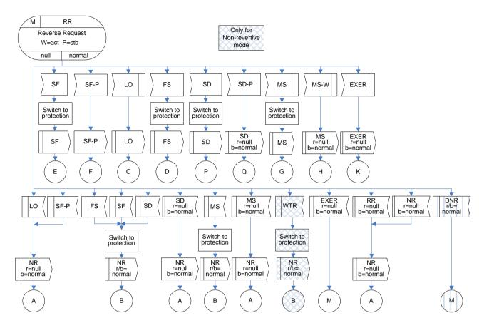
Figure IV.29 – RR(r=null, b=normal) state for 1+1 bidirectional protection switching
