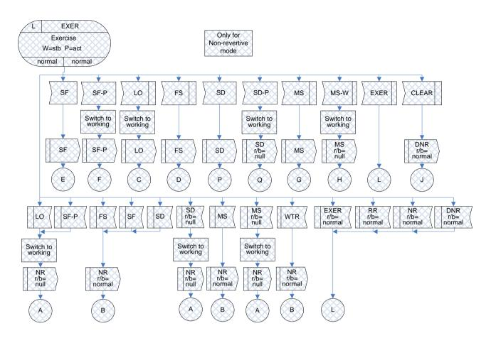
Figure IV.12 – EXER(r/b=normal) state for 1:1 bidirectional protection switching
