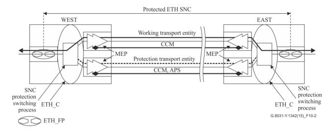
Figure 10-2 – MEPs in ETH SNC/S protection switching architecture
