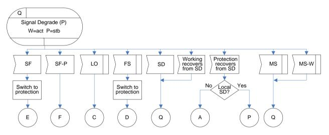
Figure IV.43 – SD(W=stb/P=act) state for 1+1 unidirectional protection switching
