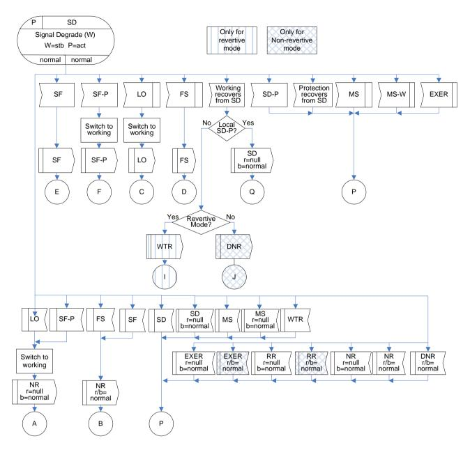
Figure IV.31 – SD(r/b=normal) state for 1+1 bidirectional protection switching
