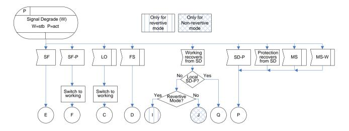
Figure IV.42 – SD(W=stb/P=act) state for 1+1 unidirectional protection switching
