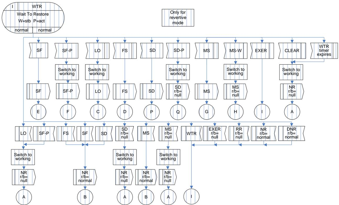
**Figure IV.9 – WTR(r/b=normal) state for 1:1 bidirectional protection switching**
