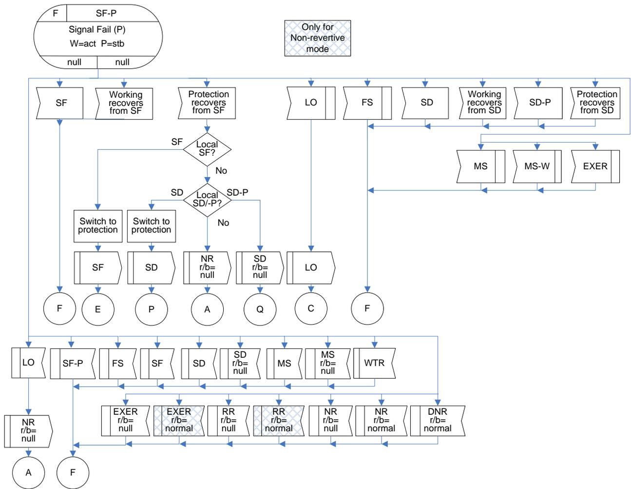
Figure IV.6 – SF-P(r/b=null) state for 1:1 bidirectional protection switching
