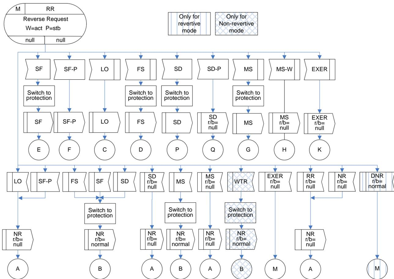
**Figure IV.13 – RR(r/b=null) state for 1:1 bidirectional protection switching**
