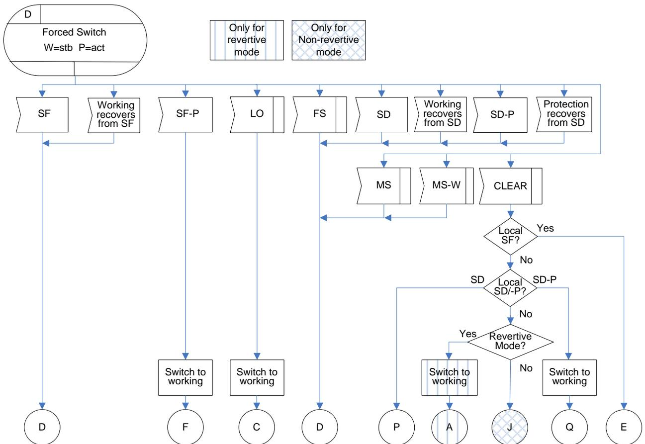
**Figure IV.35 – FS(W=stb/P=act) state for 1+1 unidirectional protection switching**
