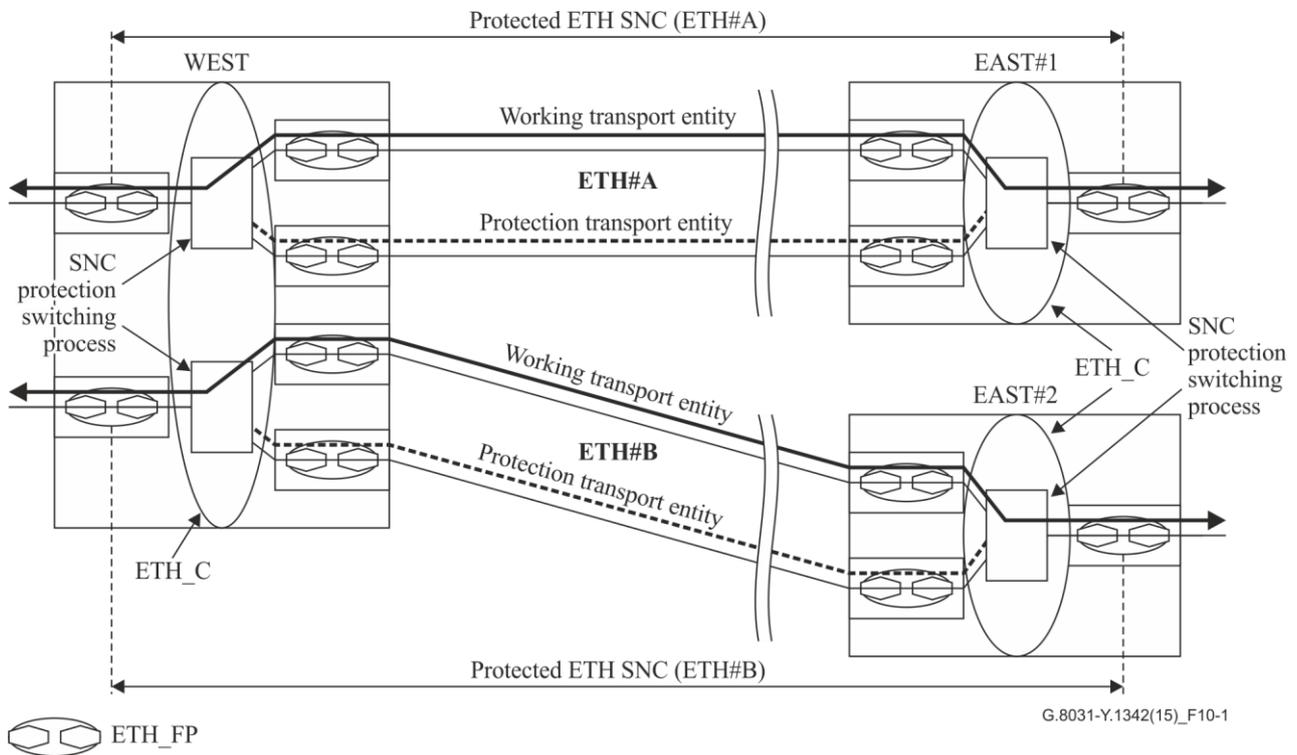
**Figure 10-1 – ETH SNC/S protection switching architecture**
