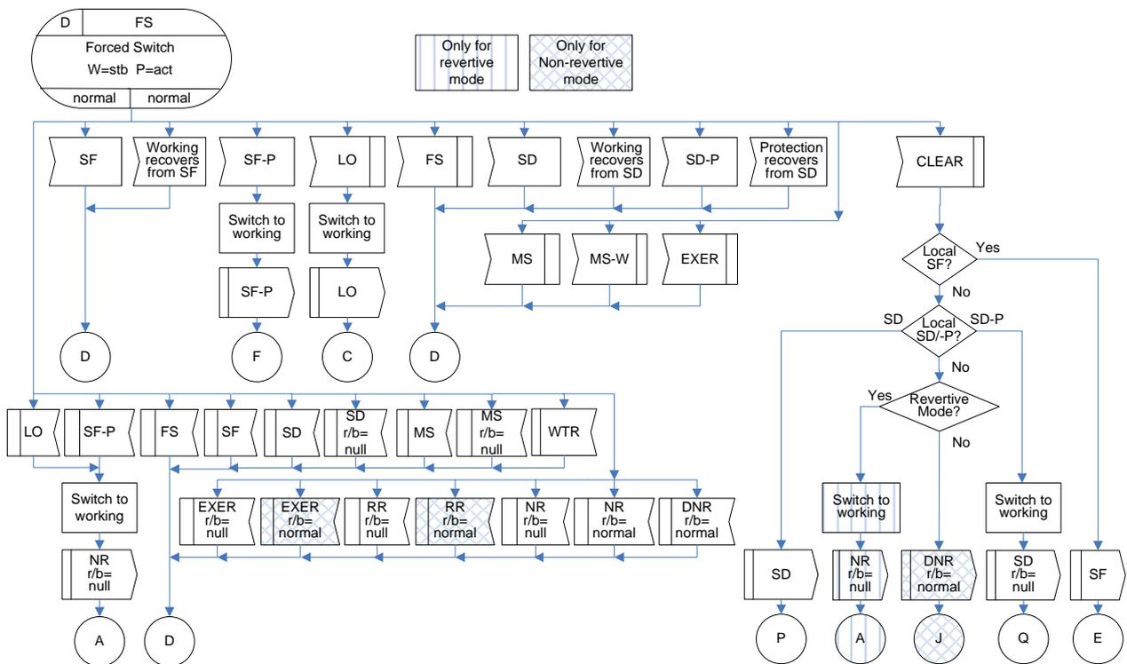
Figure IV.4 – FS(r/b=normal) state for 1:1 bidirectional protection switching
