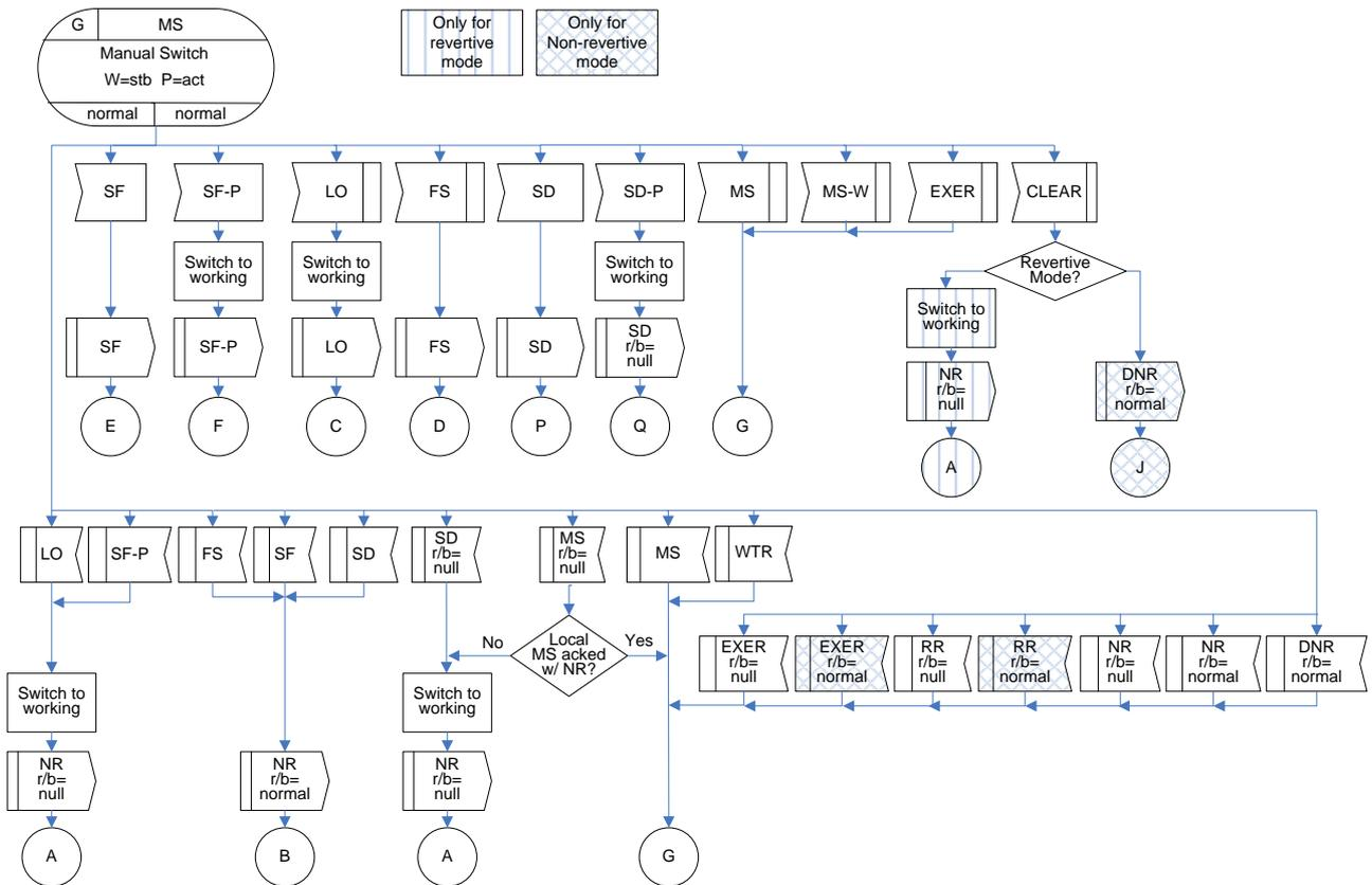
Figure IV.7 – MS(r/b=normal) state for 1:1 bidirectional protection switching
