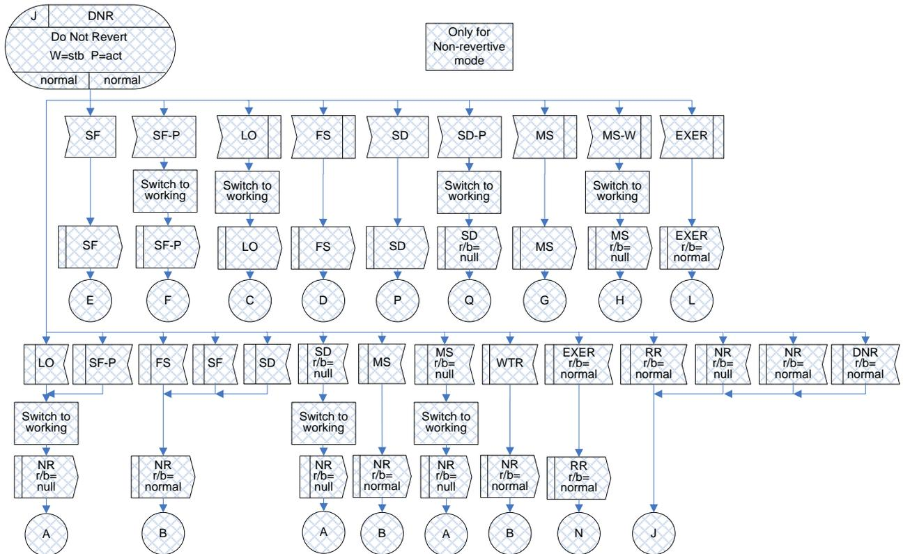
**Figure IV.10 – DNR(r/b=normal) state for 1:1 bidirectional protection switching**
