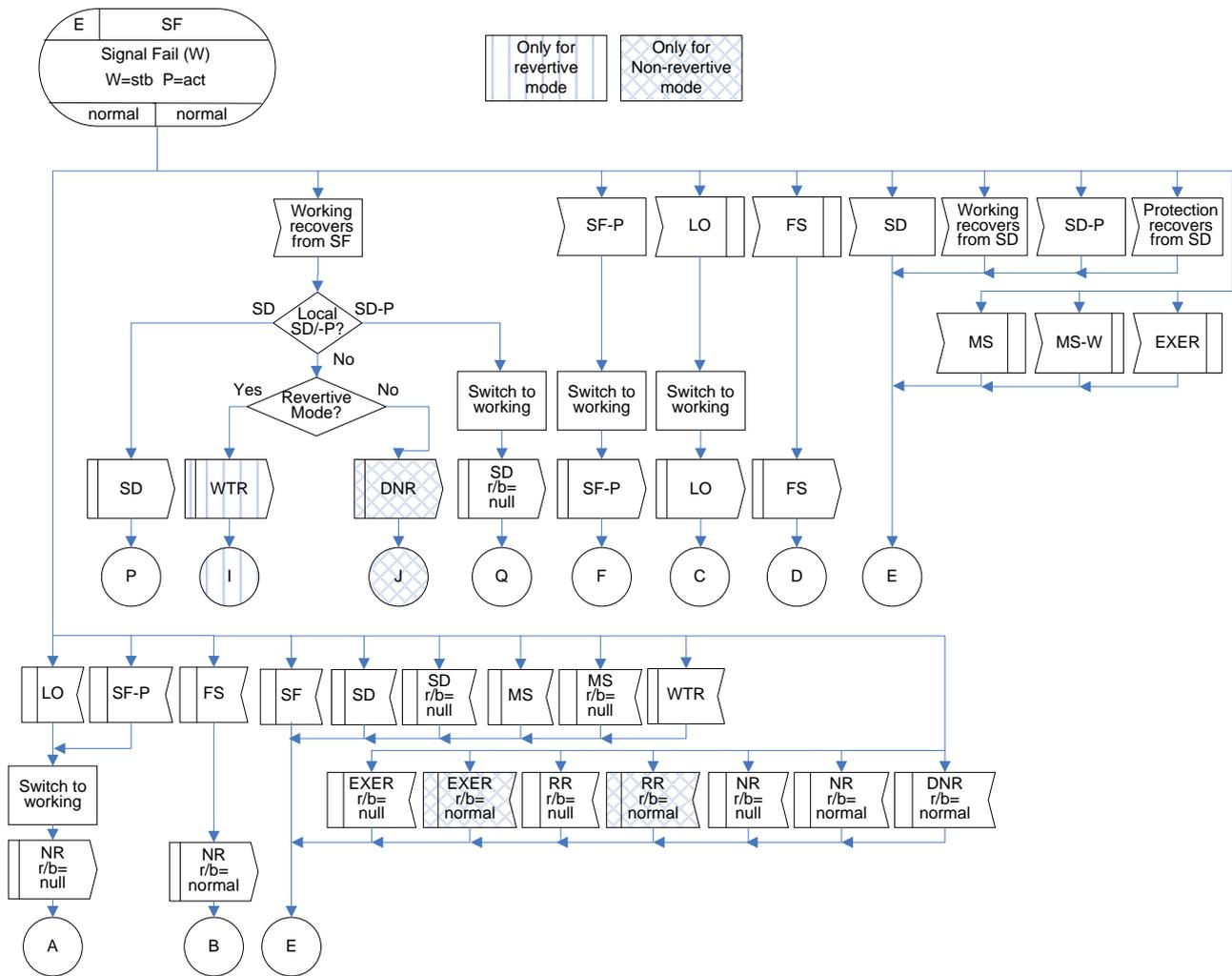
**Figure IV.5 – SF(r/b=normal) state for 1:1 bidirectional protection switching**
