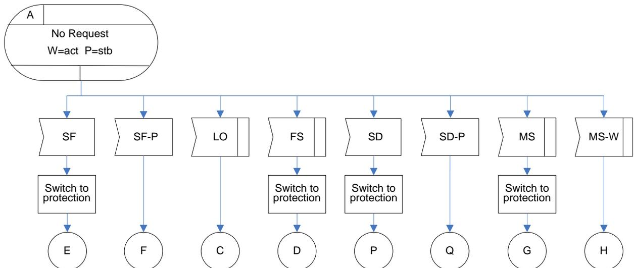
Figure IV.33 – NR(W=act/P=stb) state for 1+1 unidirectional protection switching
