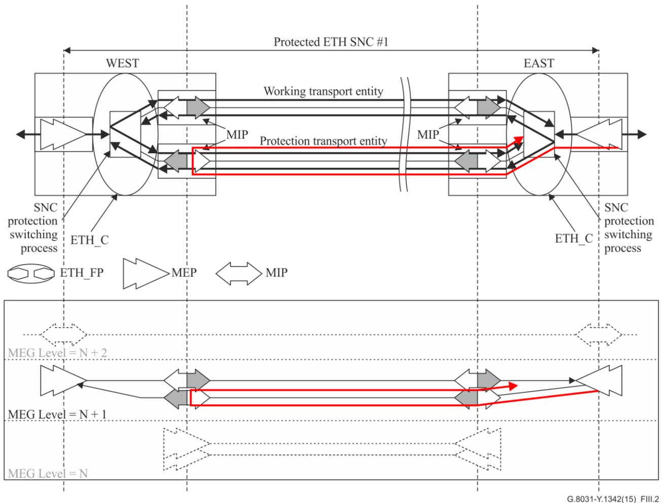
**Figure III.2 – MEPs and MIPs for 1+1 unidirectional protection switching**
