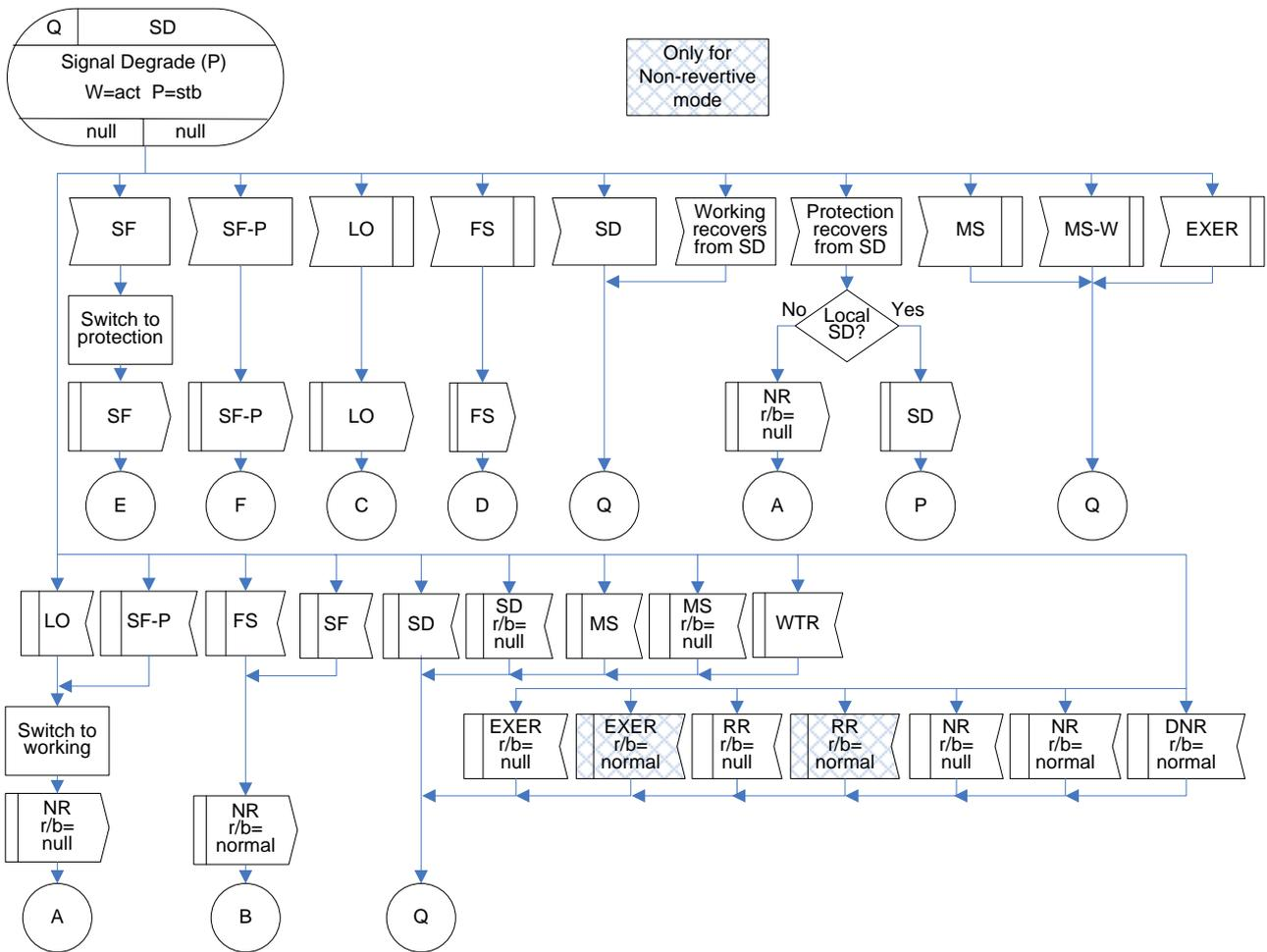
**Figure IV.16 – SD(r/b=null) state for 1:1 bidirectional protection switching**
