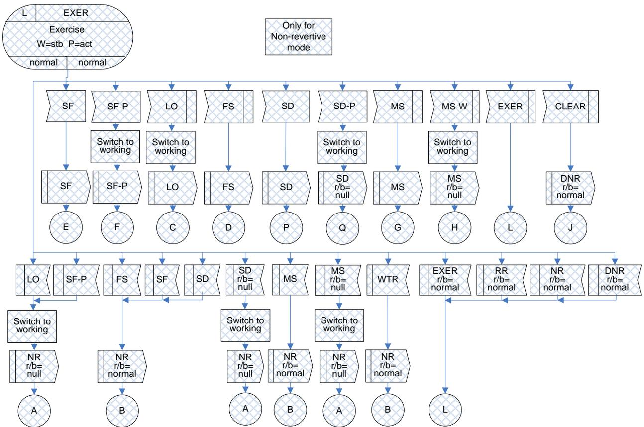
Figure IV.12 – EXER(r/b=normal) state for 1:1 bidirectional protection switching
