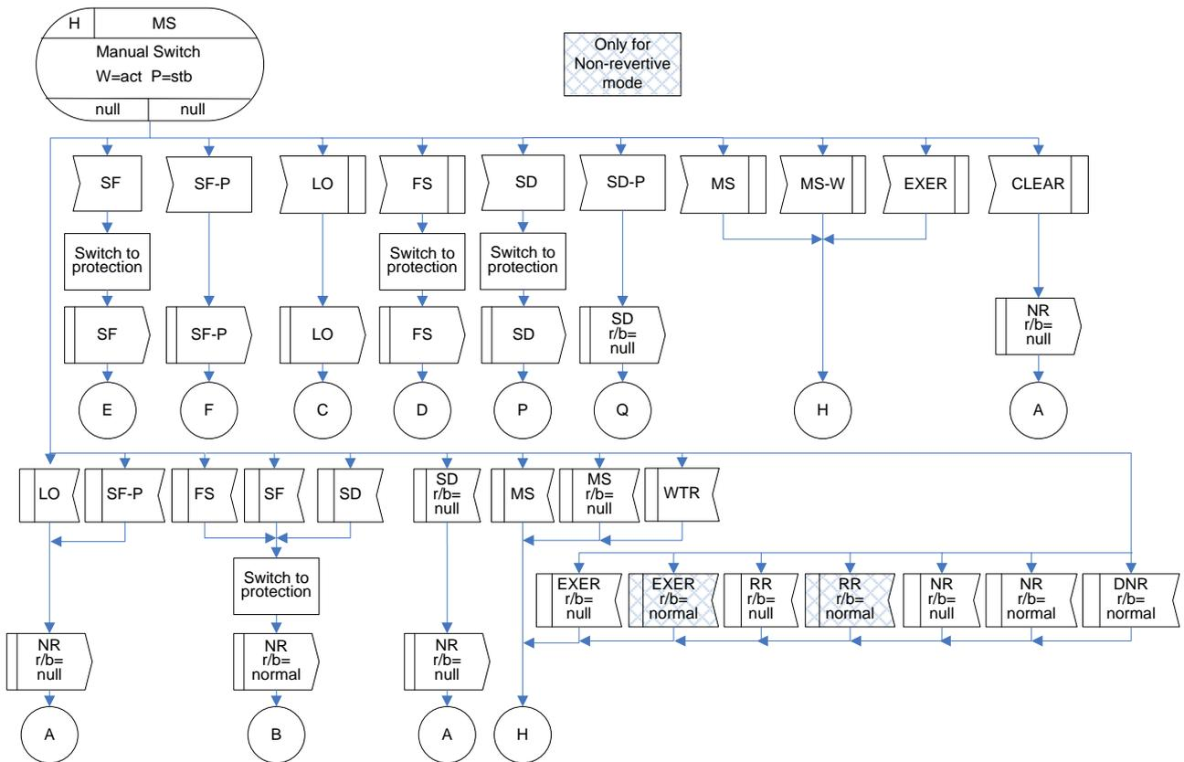
Figure IV.8 – MS(r/b=null) state for 1:1 bidirectional protection switching
