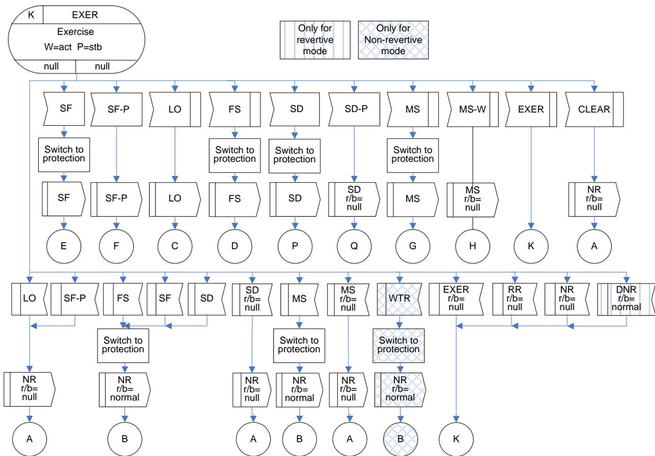
Figure IV.11 – EXER(r/b=null) state for 1:1 bidirectional protection switching
