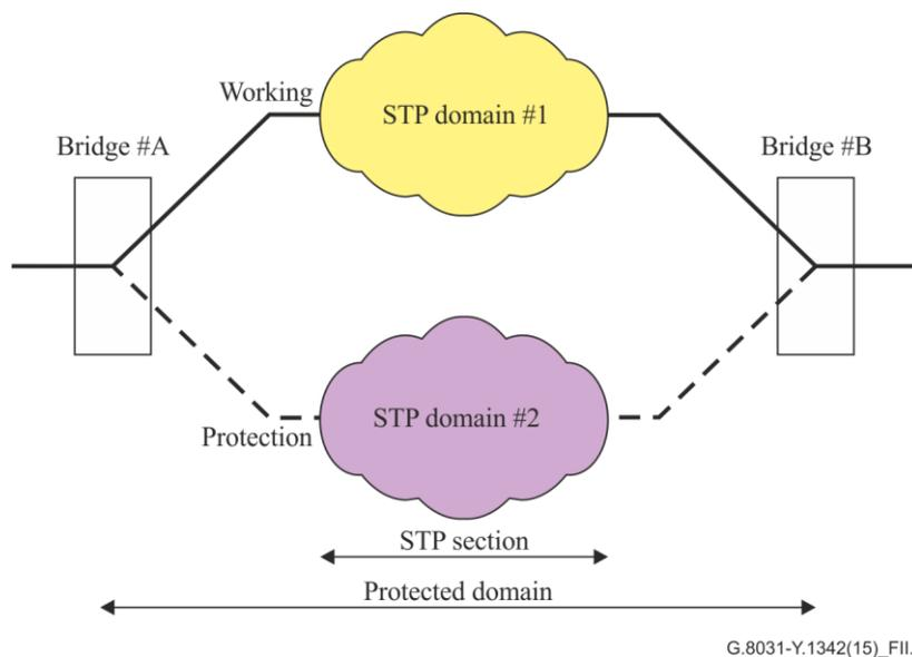
**Figure II.2 – Overlapping between the protected domain and STP**
