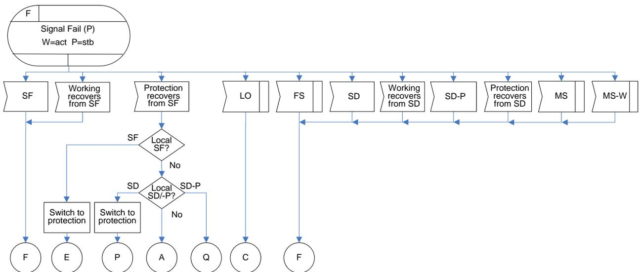
**Figure IV.37 – SF-P(W=act/P=stb) state for 1+1 unidirectional protection switching**
