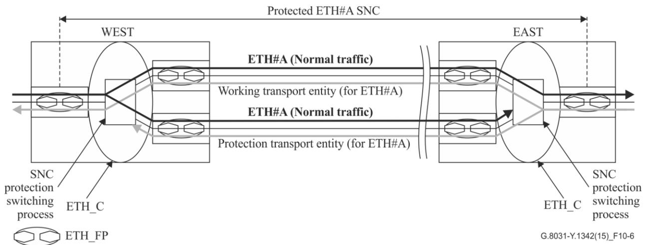
**Figure 10-6 – 1+1 unidirectional protection switching architecture**
