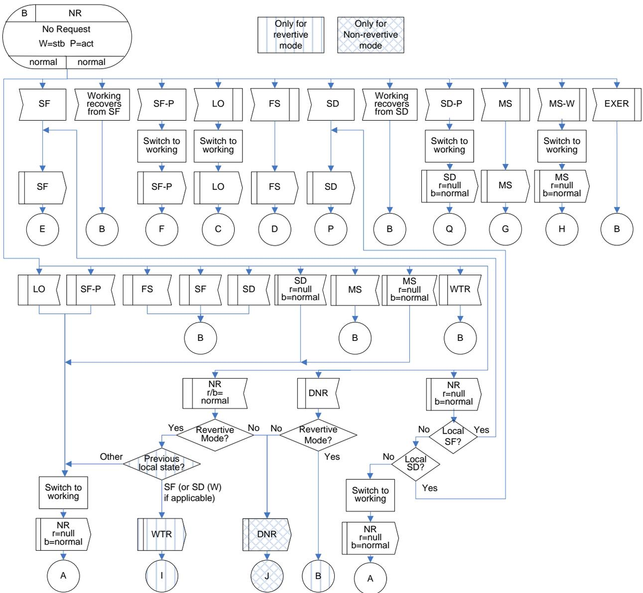
**Figure IV.18 – NR(r/b=normal) state for 1+1 bidirectional protection switching**
