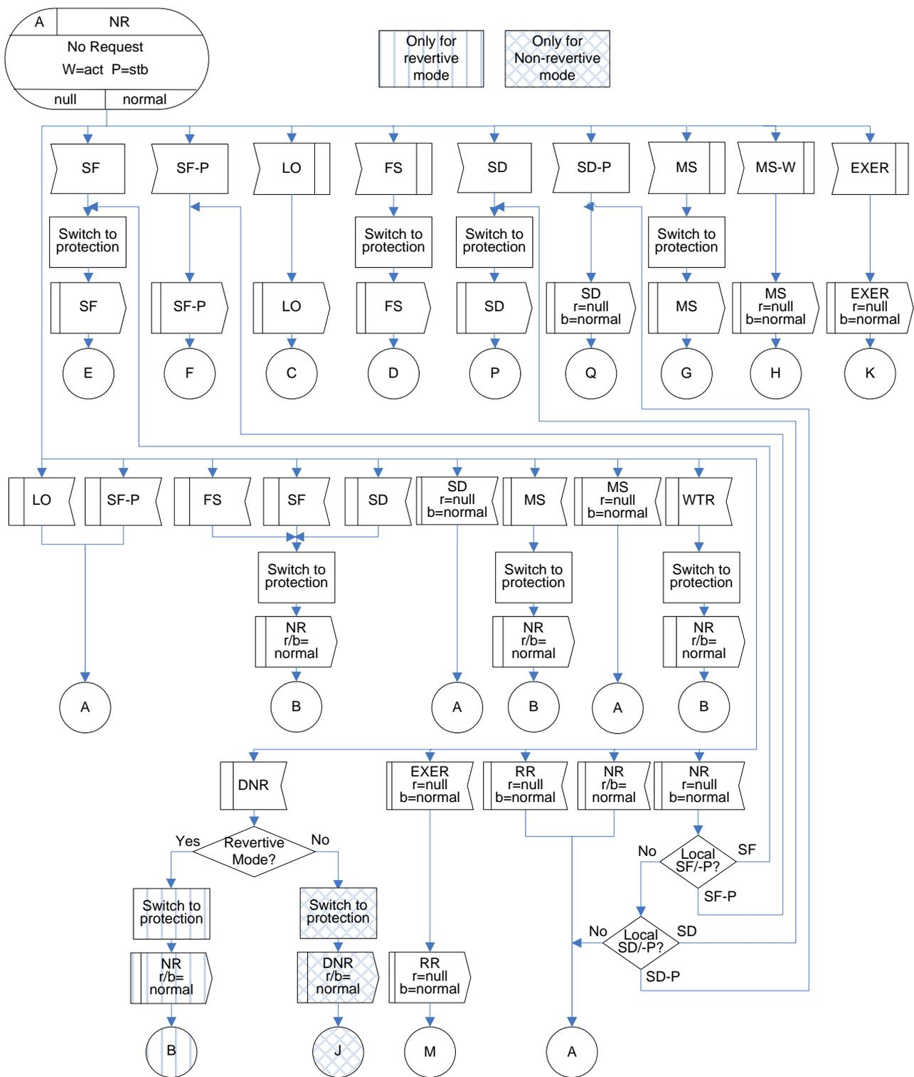
Figure IV.17 – NR(r=null, b=normal) state for 1+1 bidirectional protection switching
