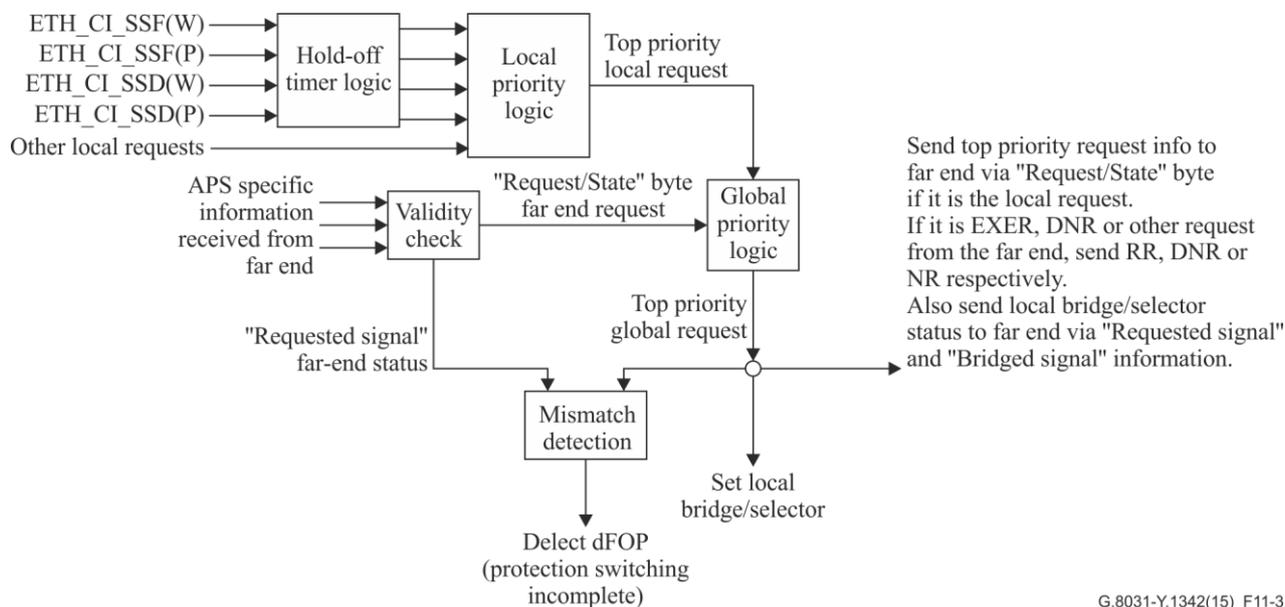
**Figure 11-3 – Principle of 1+1/1:1 linear protection switching algorithm**
