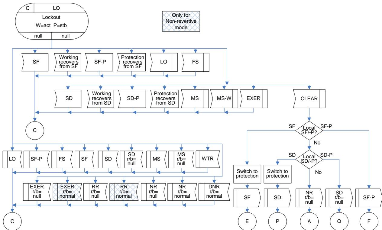
Figure IV.3 – LO(r/b=null) state for 1:1 bidirectional protection switching
