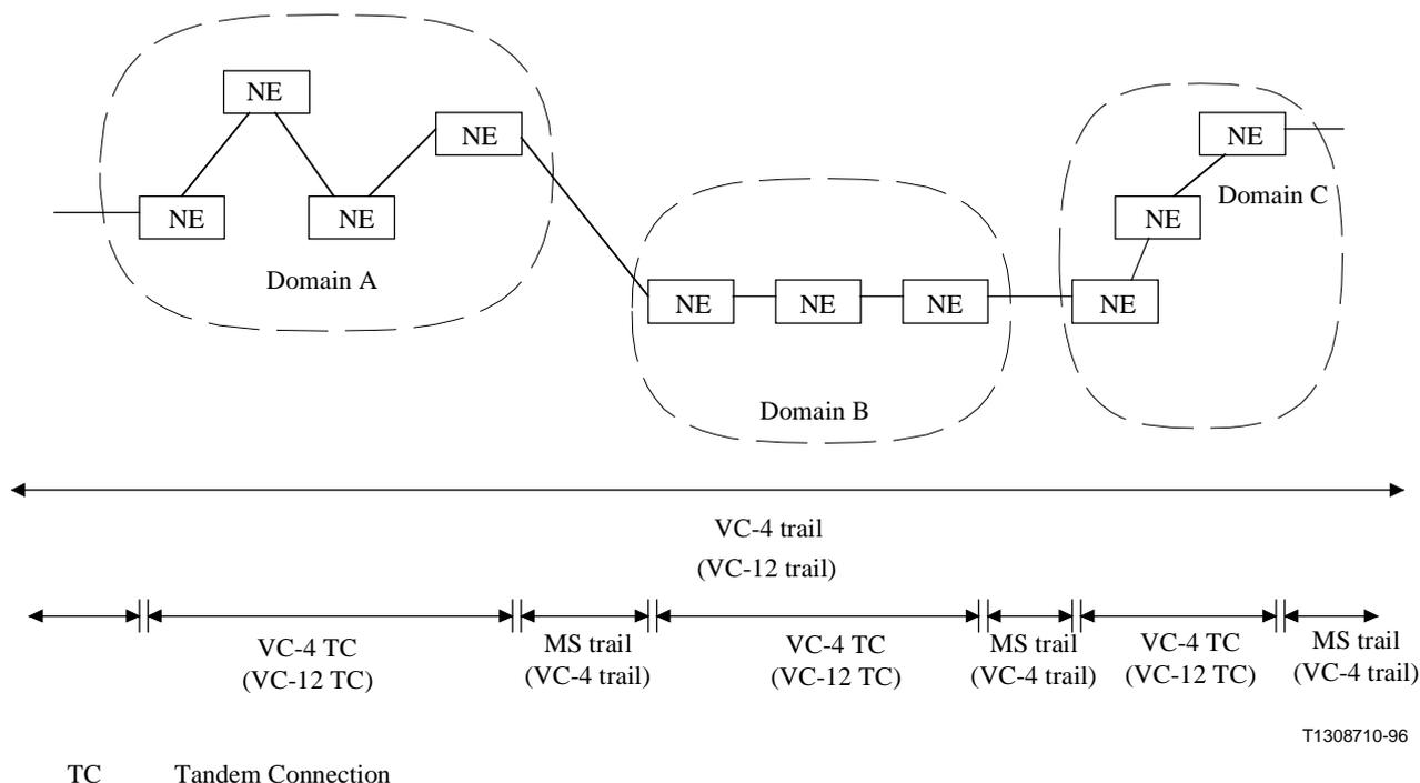
**Figure 6-2/G.803 – Multi-operator domain VC-*n* trail, monitored via tandem connections**
