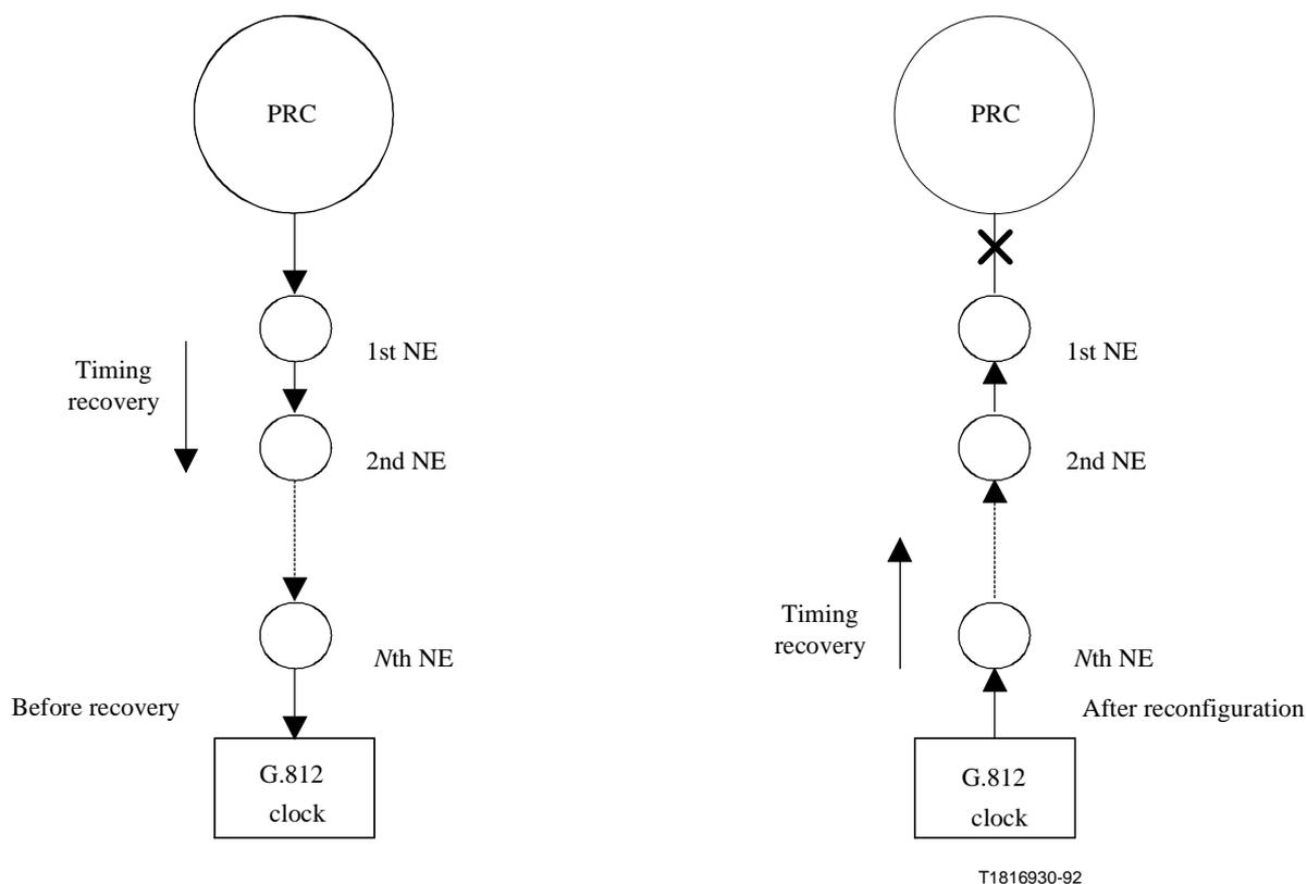
**Figure 8-6/G.803 – Reconfiguration example**
