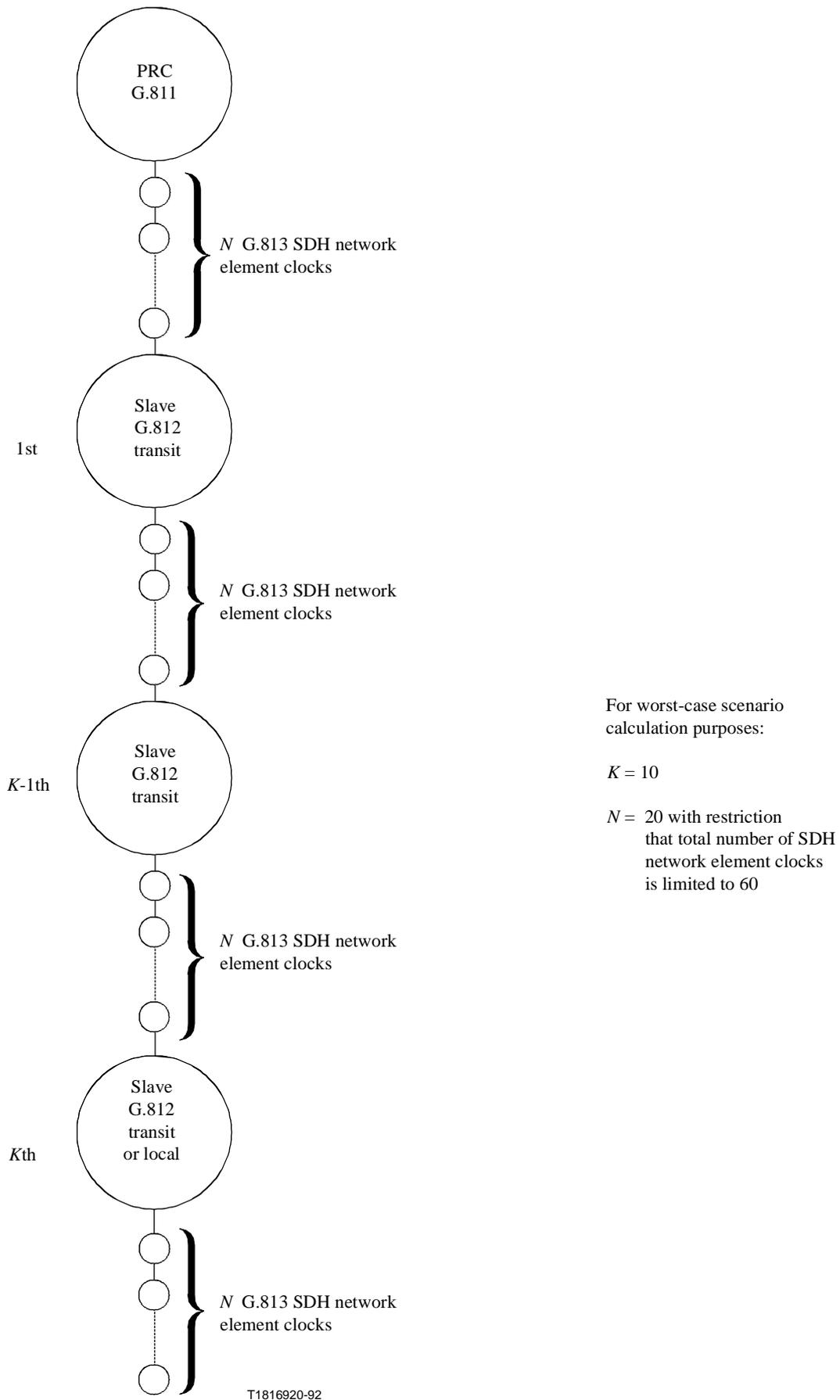
**Figure 8-5/G.803 – Synchronization network reference chain**
