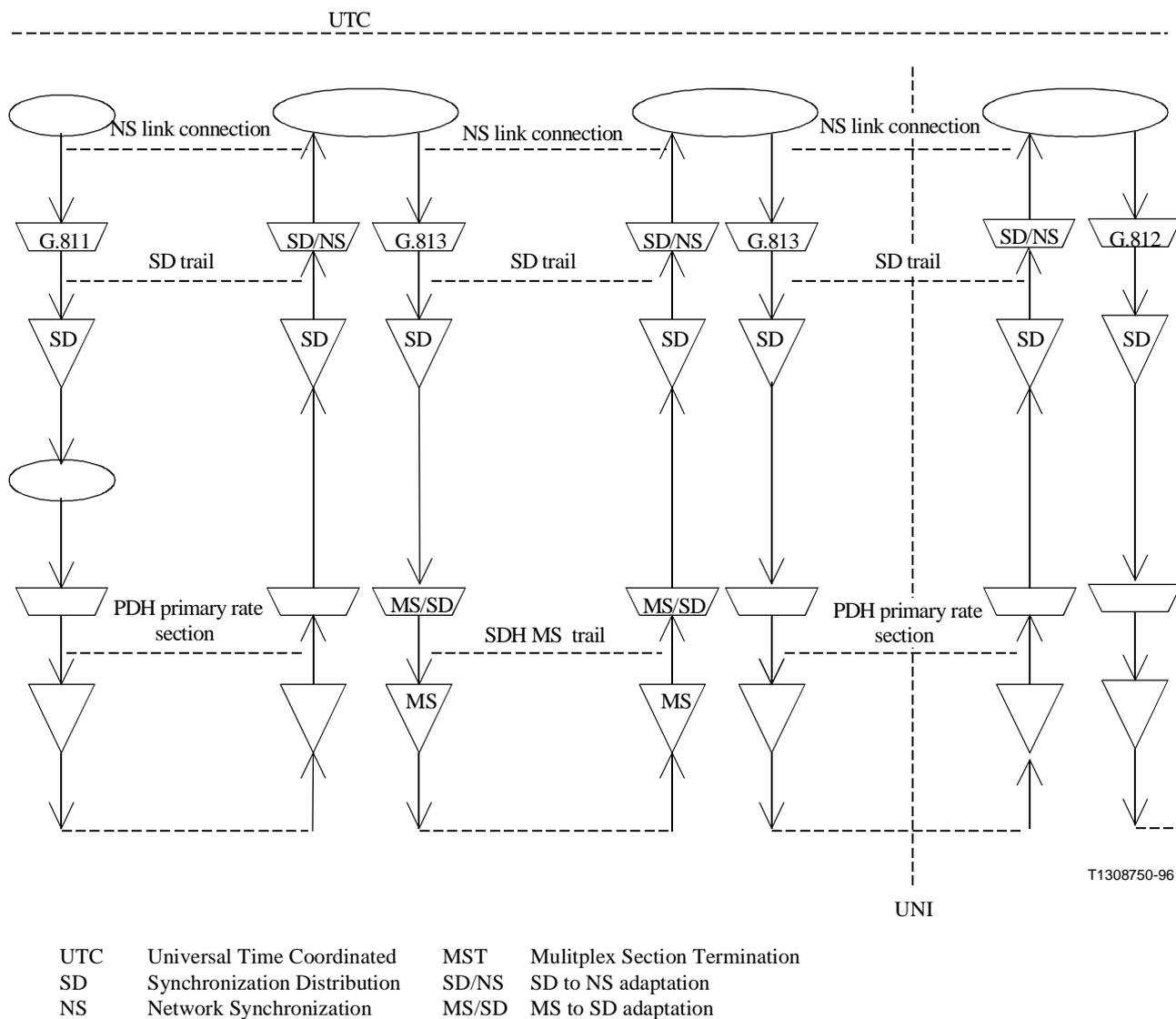
**Figure 8-4/G.803 – Example of synchronization distribution across a PDH UNI**
