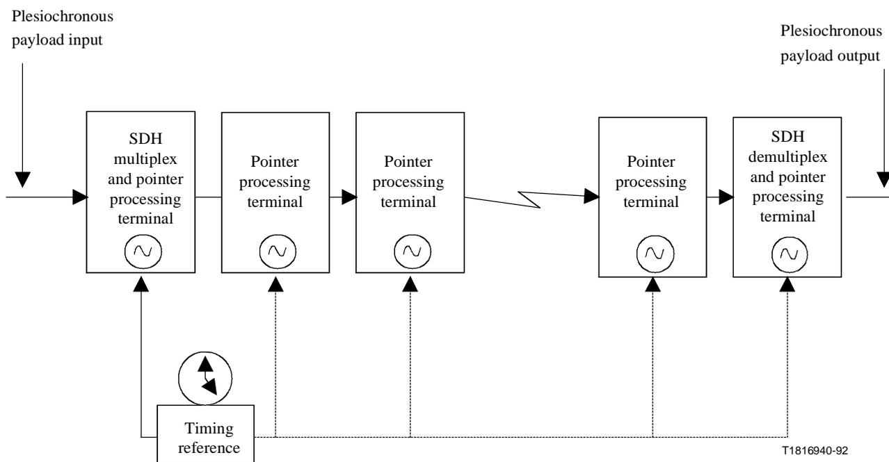
**Figure 8-7/G.803 – SDH network model for pointer activity simulation**
