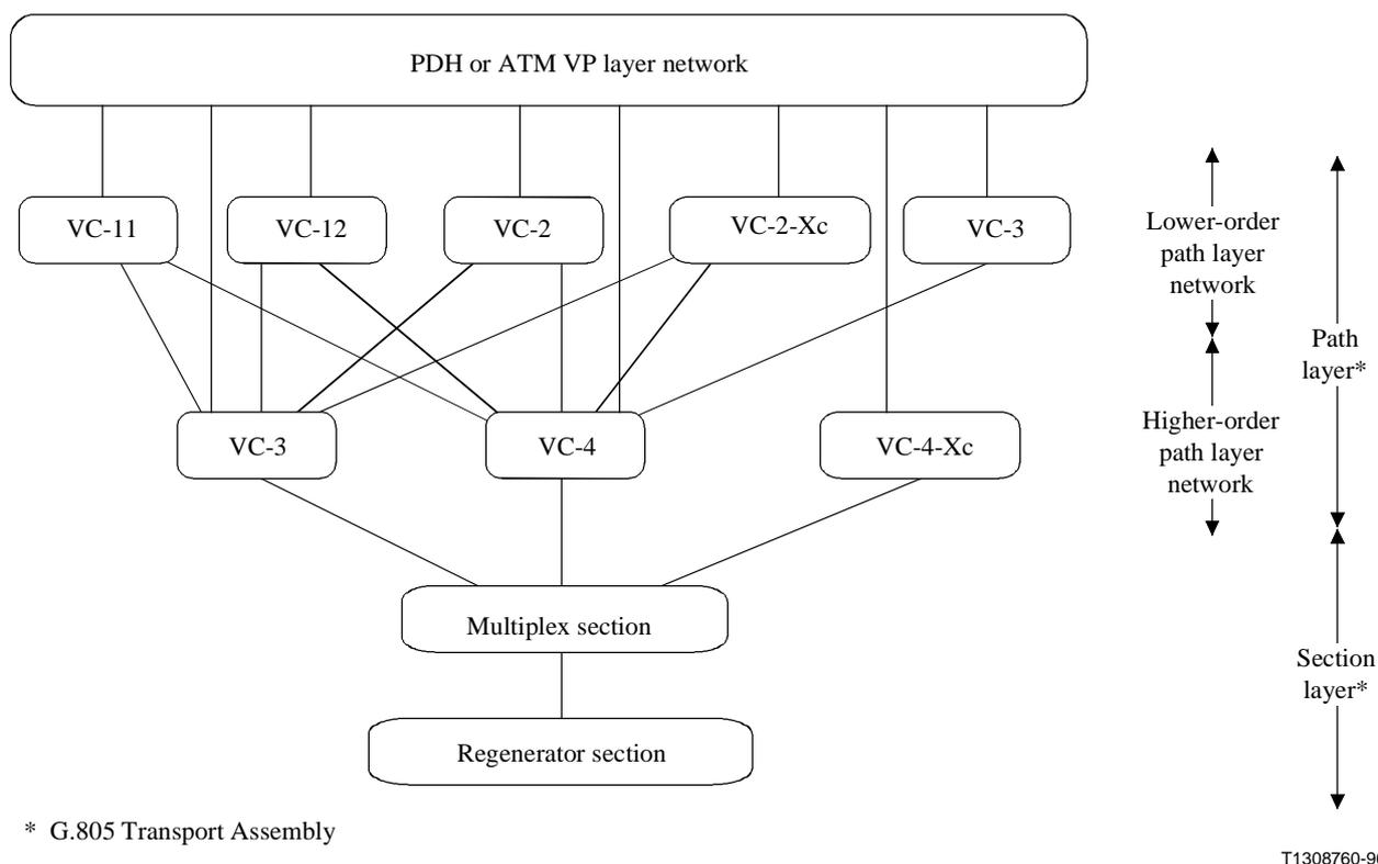
**Figure I.1/G.803 – SDH Layer networks**
