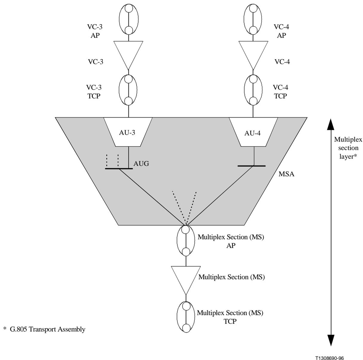
Figure 5-3/G.803 – Multiplex Section (MS) supporting VC-3 and VC-4
