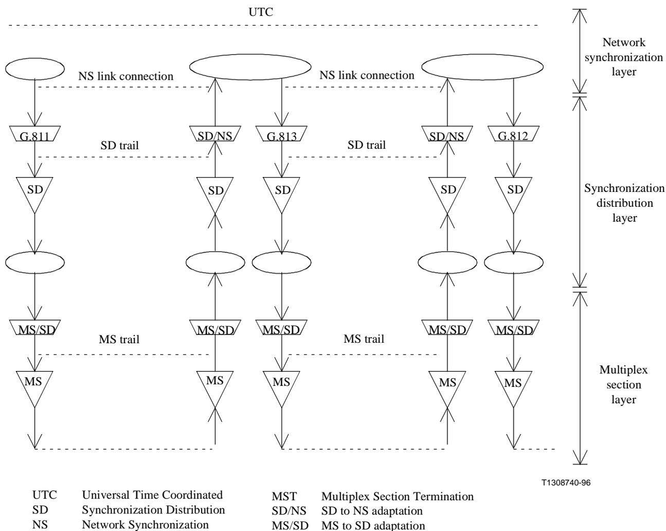
**Figure 8-3/G.803 – Example of synchronization distribution showing the synchronization layers**
