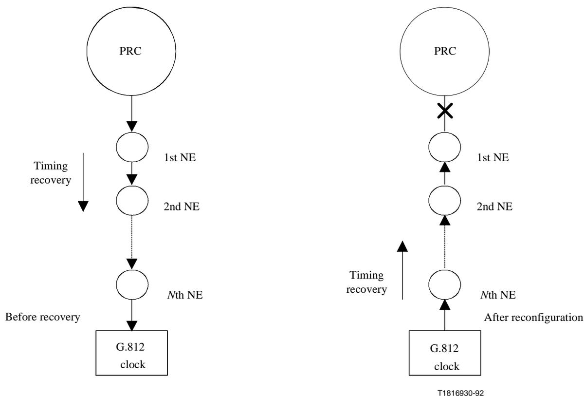
**Figure 8-6/G.803 – Reconfiguration example**
