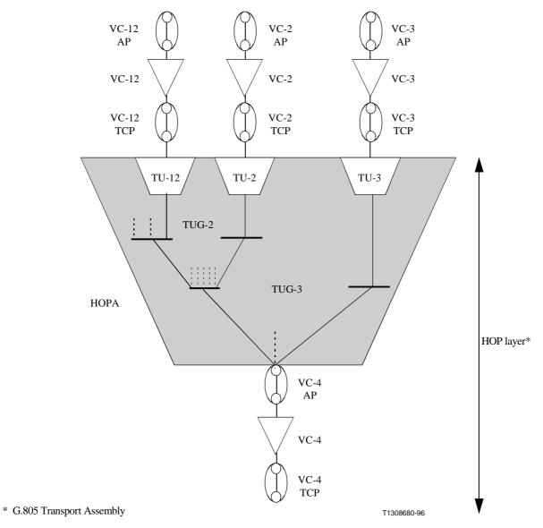
Figure 5-2/G.803 – VC-4 supporting multiple client layer networks
