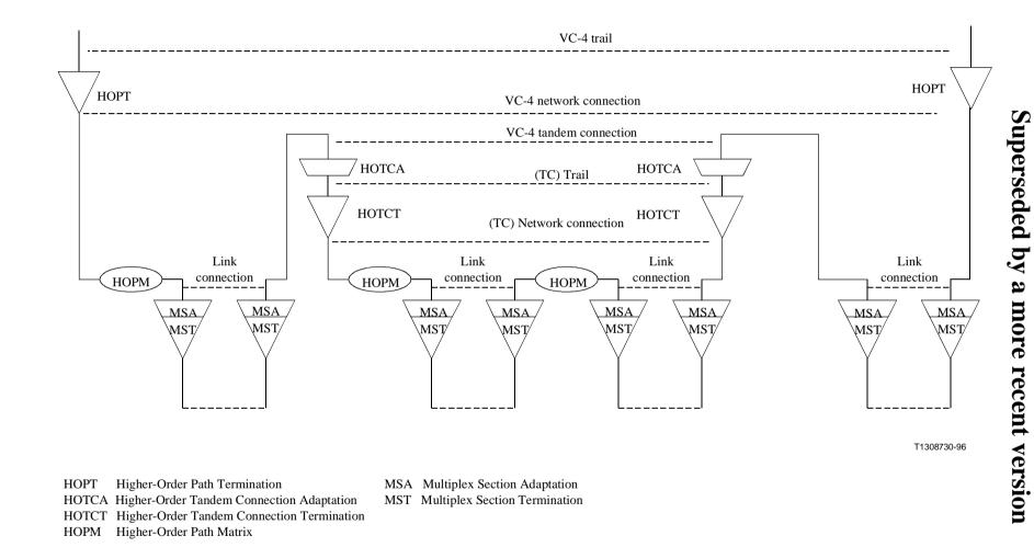
Figure 6-4/G.803 – Example of a VC-trail with a tandem connection in an intermediate operator domain
