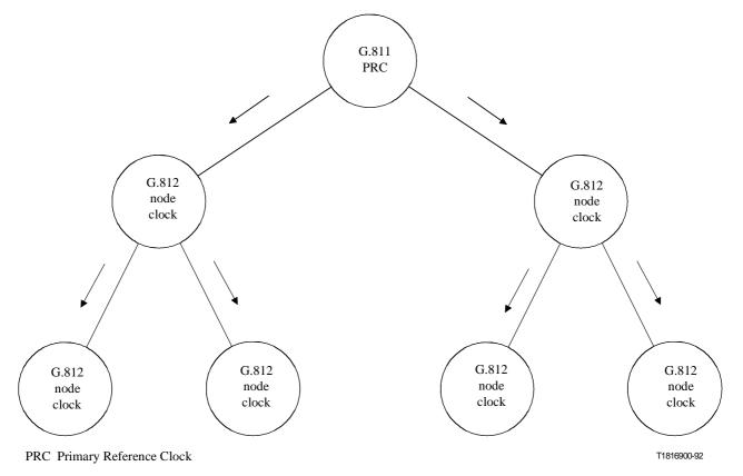
Figure 8-2/G.803 – Synchronization network architecture inter-node distribution
