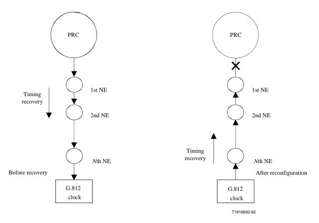
**Figure 8-6/G.803 – Reconfiguration example**
