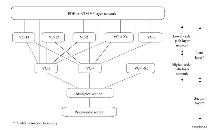
Figure I.1/G.803 – SDH Layer networks
