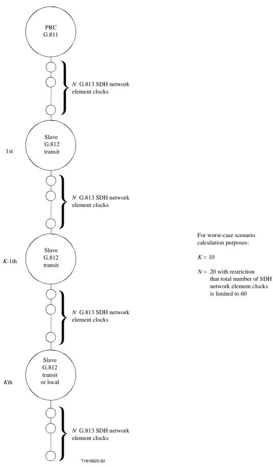
Figure 8-5/G.803 – Synchronization network reference chain
