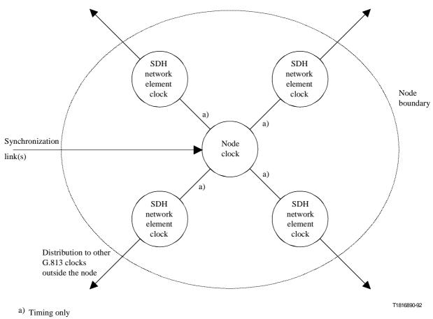
Figure 8-1/G.803 – Synchronization network architecture intra-node distribution
