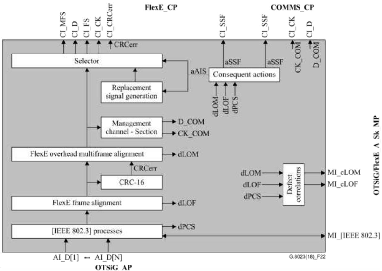
Figure 6-22 – OTSiG M-AI/FlexE\_A\_Sk processes
