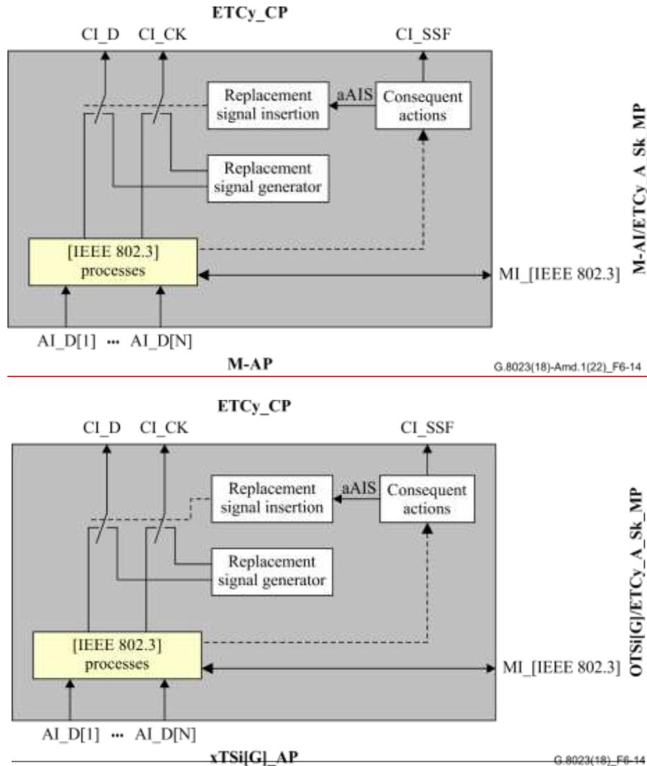
**Figure 6-14 –  $\times$ TSi[G]M-AI/ETCy\_A\_Sk processes**
