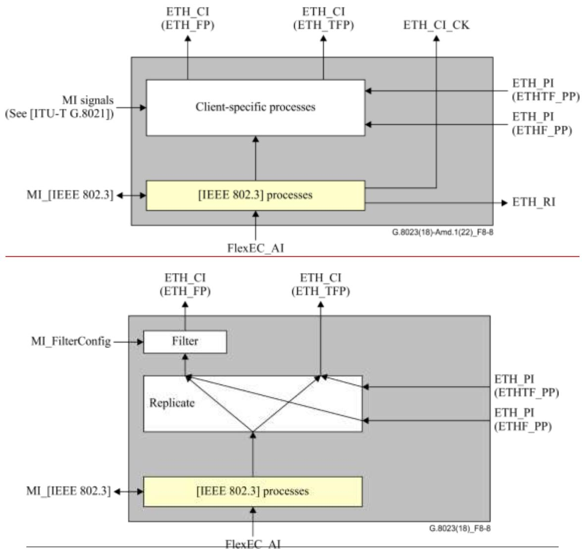
**Figure 8-8 – FlexEC/ETH\_A\_Sk processes**
