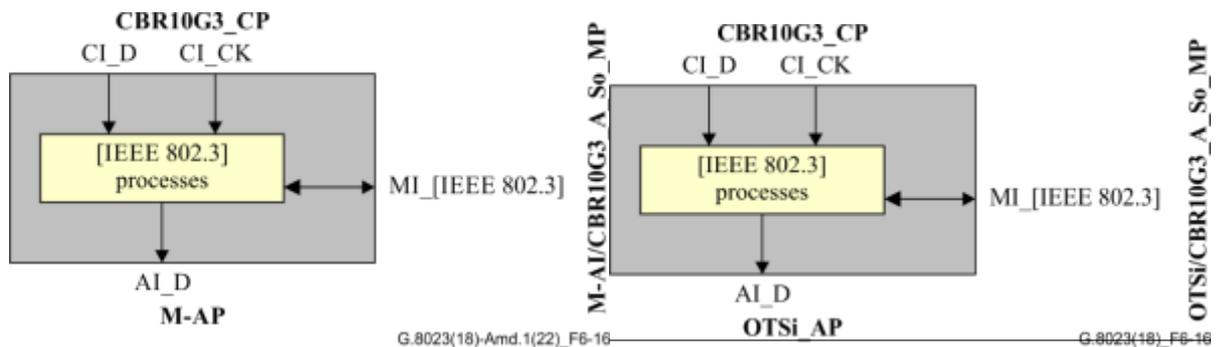
**Figure 6-16 – OTSiM-AI/CBR10G3\_A\_So processes**
