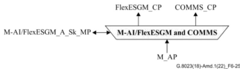
**Figure 6-25 – M-AI/FlexESGM A Sk function**
