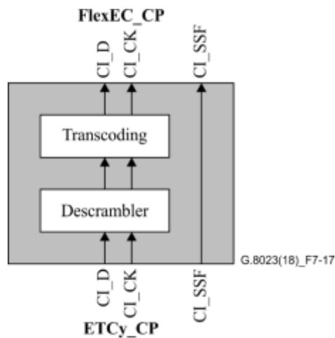
**Figure 7-17 – ETCy>FlexEC processes (y = 10GR, 25GR)**
