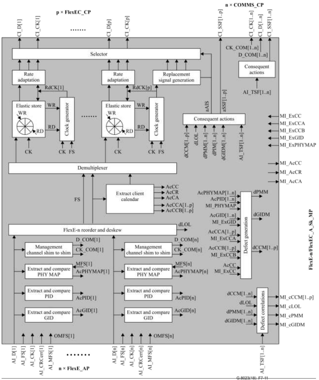
Figure 7-11 – FlexE-n/FlexEC\_A\_Sk processes
