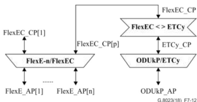
**Figure 7-12 – FlexEC<>ETCy function position**
