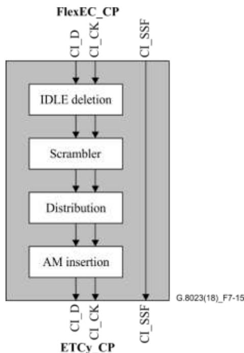
**Figure 7-15 – FlexEC>ETCy processes (y = 40GR, 50GR, 100GR)**
