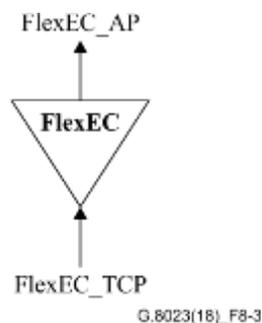
**Figure 8-3 – FlexEC\_TT\_Sk function**
