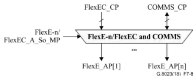
**Figure 7-8 – FlexE-n/FlexEC\_A\_So function**
