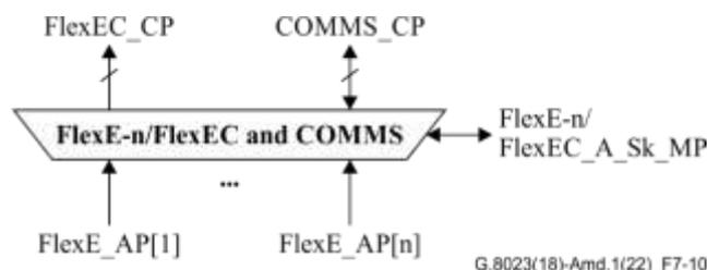
**Figure 7-10 – FlexE-n/FlexEC\_A\_Sk function**
