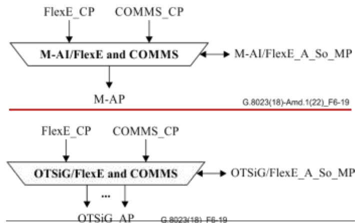
**Figure 6-19 –  $\Theta$ TSiGM-AI/FlexE\_A\_So function**
