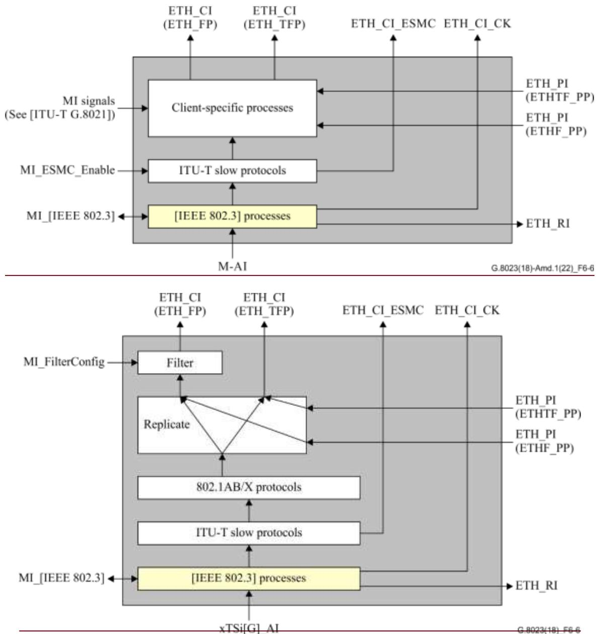
**Figure 6-6 –  $xTSi[G]M-AI/ETH\_A\_Sk$  process**
