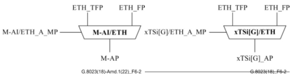
**Figure 6-2 –  $\text{xTSi[G]}$  M-AI to ETH adaptation function**
