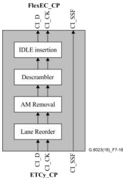
**Figure 7-18 – ETCy>FlexEC processes (y = 40GR, 50GR, 100GR)**
