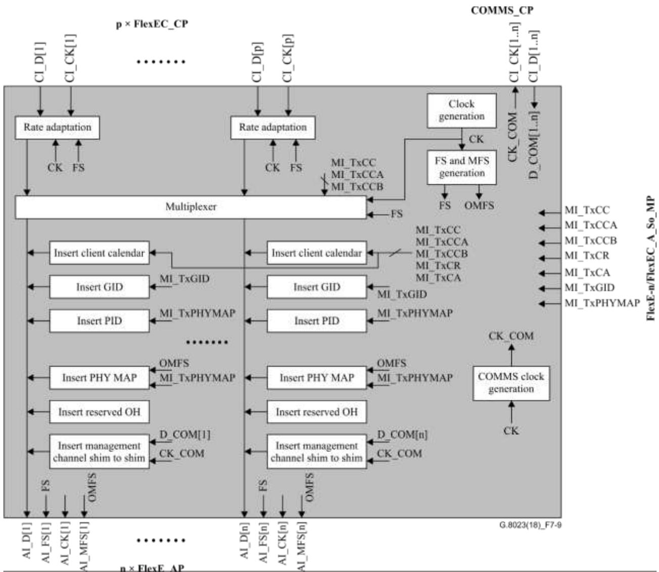
**Figure 7-9 – FlexE-n/FlexEC\_A\_So processes**
