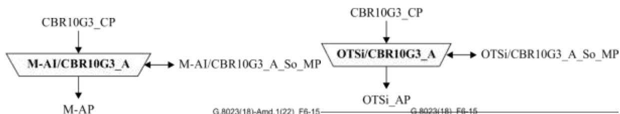
**Figure 6-15 –  $\Theta$ TSiM-AI/CBR10G3\_A\_So function**
