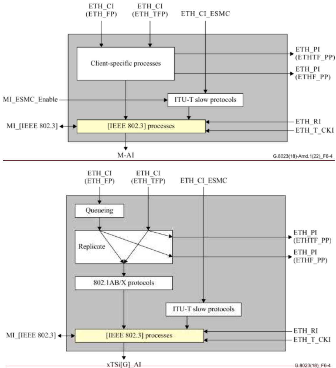
**Figure 6-4 –  $\bar{x}$ TSi[G]M-AI/ETH\_A\_So process**
