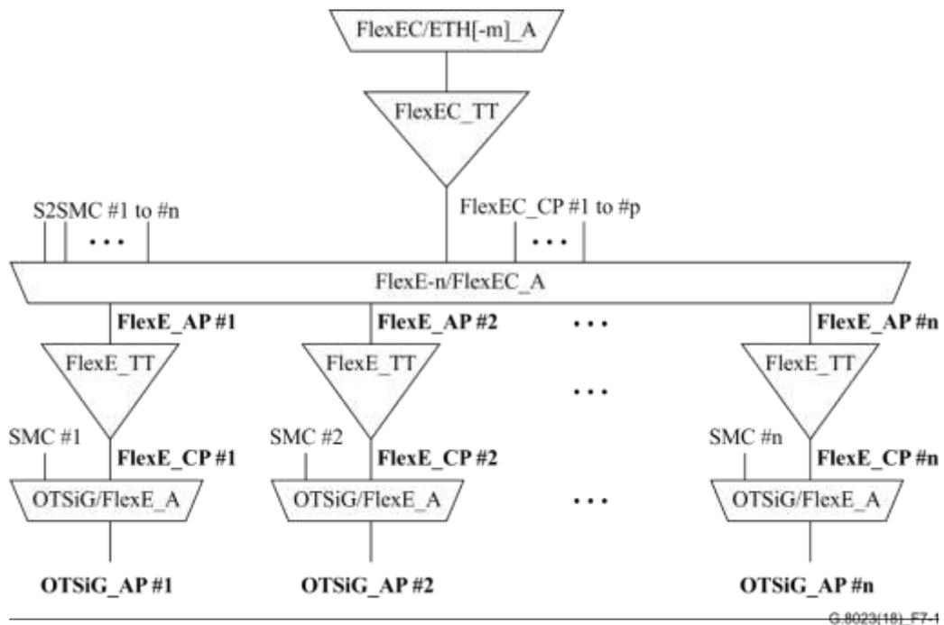
**Figure 7-1 – FlexE and FlexE client adaptation functions**
