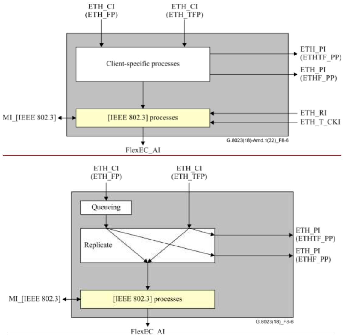
**Figure 8-6 – FlexEC/ETH\_A\_So processes**
