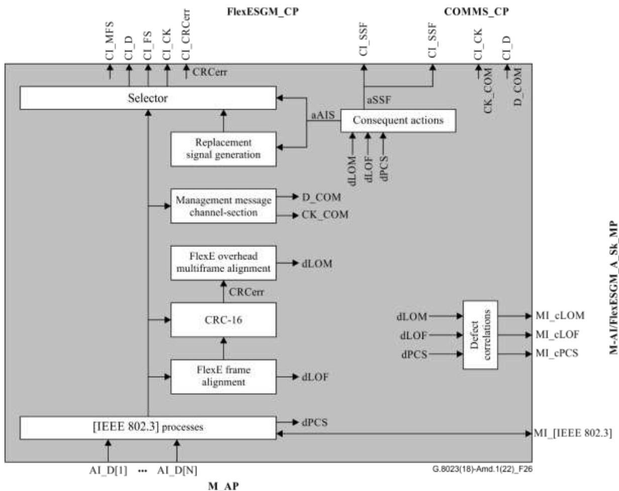
**Figure 6-26 – M-AI/FlexESGM A Sk processes**
