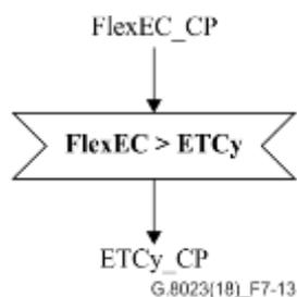
**Figure 7-13 – FlexEC>ETCy function**
