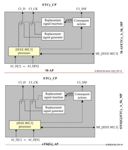
Figure 6-14 - xTSi[G]M-AI/ETCy\_A\_Sk processes
