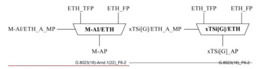
Figure 6-2 – **xTSi[G]M-AI** to ETH adaptation function
