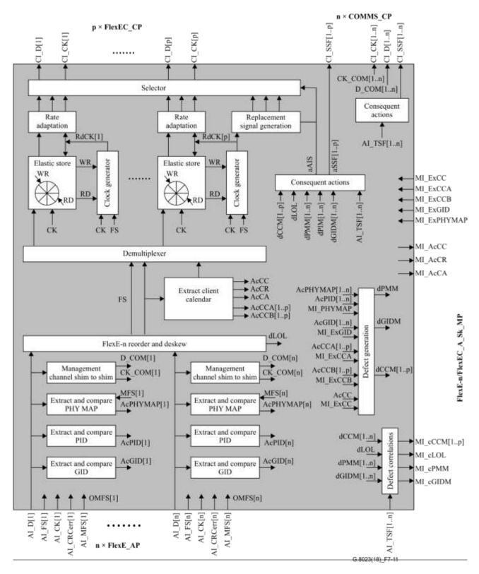
Figure 7-11 – FlexE-n/FlexEC\_A\_Sk processes
