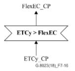
Figure 7-16 – ETCy>FlexEC function
