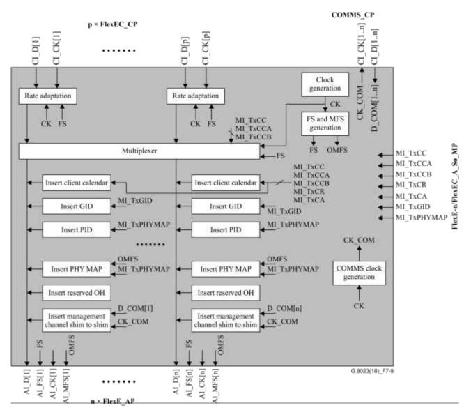
Figure 7-9 – FlexE-n/FlexEC\_A\_So processes
