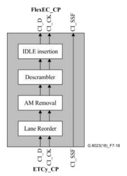
Figure 7-18 – ETCy>FlexEC processes (y = 40GR, <u>50GR</u>, 100GR)
