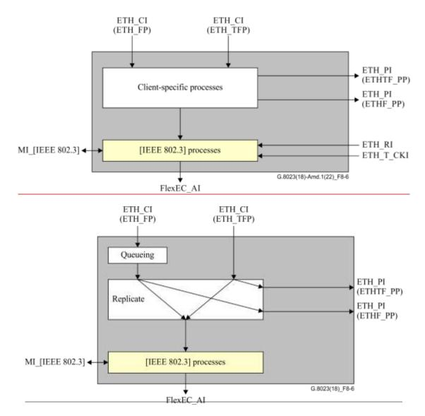
Figure 8-6 – FlexEC/ETH\_A\_So processes
