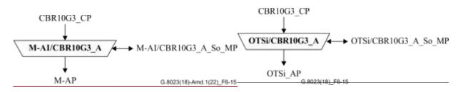
Figure 6-15 - OTSiM-AI/CBR10G3\_A\_So function
