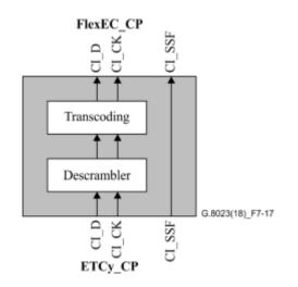
Figure 7-17 – ETCy>FlexEC processes (y = 10GR, 25GR)
