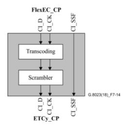
Figure 7-14 – FlexEC>ETCy processes (y = 10GR, 25GR)
