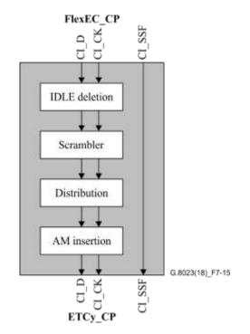
Figure 7-15 – FlexEC>ETCy processes (y = 40GR, <u>50GR</u>, 100GR)
