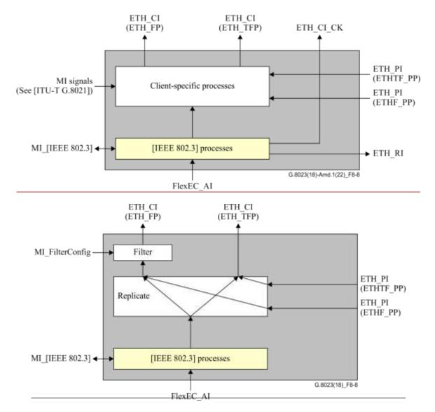
Figure 8-8 – FlexEC/ETH\_A\_Sk processes
