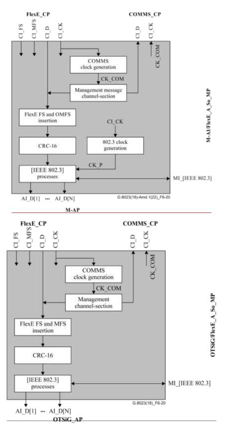
Figure 6-20 – OTSiGM-AI/FlexE\_A\_So processes
