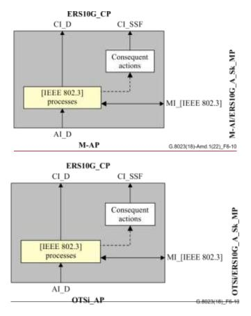
Figure 6-10 - OTSiM-AI/ERS10G\_A\_Sk processes
