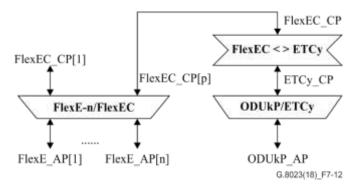
Figure 7-12 – FlexEC<>ETCy function position
