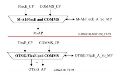
Figure 6-19 – OTSiGM-AI/FlexE\_A\_So function
