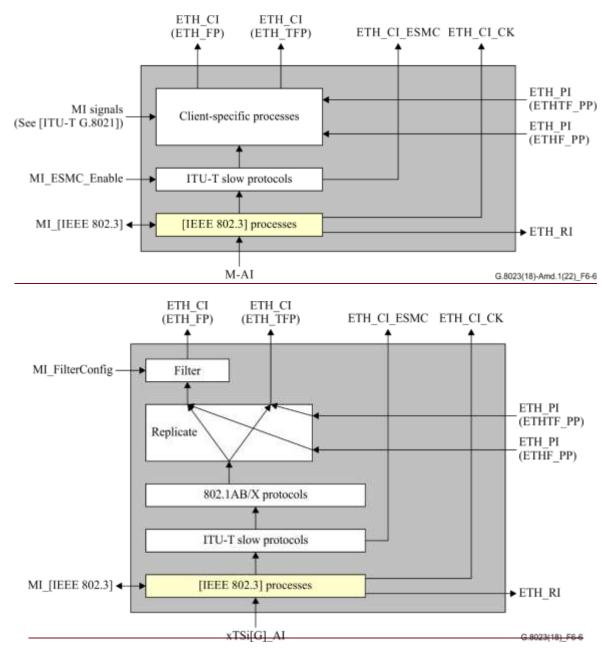
Figure 6-6 – **\*TSi[G]M-AI/ETH\_A\_Sk** process
