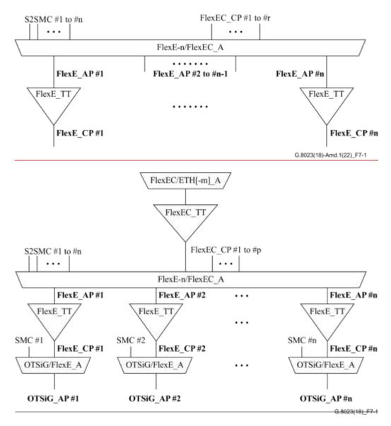
**Figure 7-1 – FlexE and FlexE client adaptation functions**
