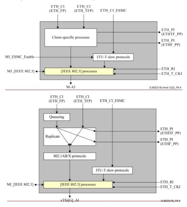
Figure 6-4 - **\*TSi[G]M-AI/ETH\_A\_So process**
