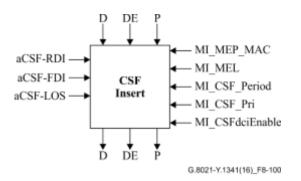
**Figure 8-100 – CSF insert process**
