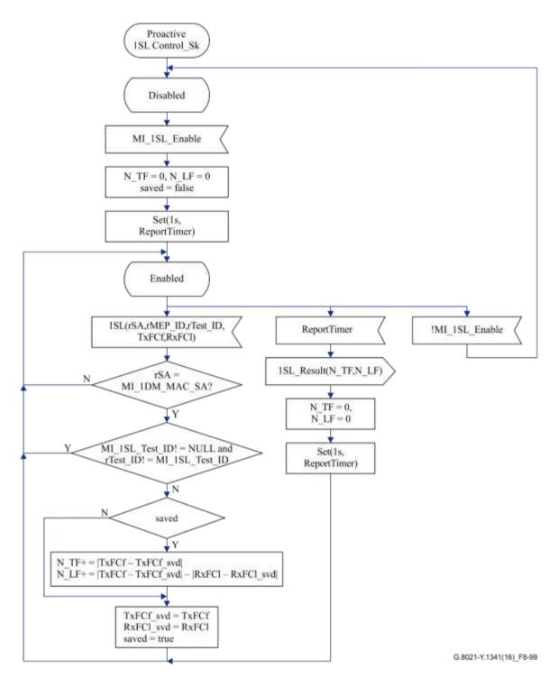
Figure 8-99 – Proactive 1SL Control\_Sk process
