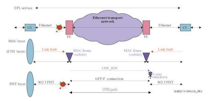
**Figure II.3 – Fault on egress**
