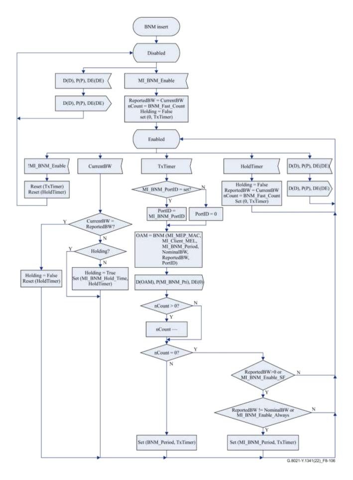
Figure 8-106 – BNM insert behaviour
