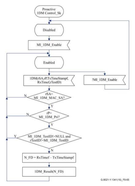
Figure 8-65 – Proactive 1DM Control\_Sk process
