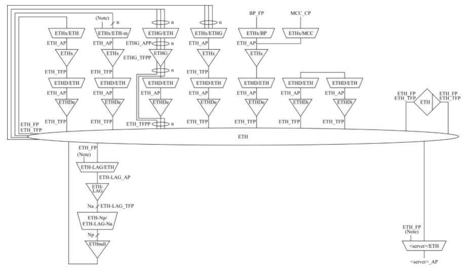
NOTE - ETH\_TFP interface of adaptation functions towards the ETH\_FT functions connects to logical link control. See [ITU-T G.8010] and function definition for details.
