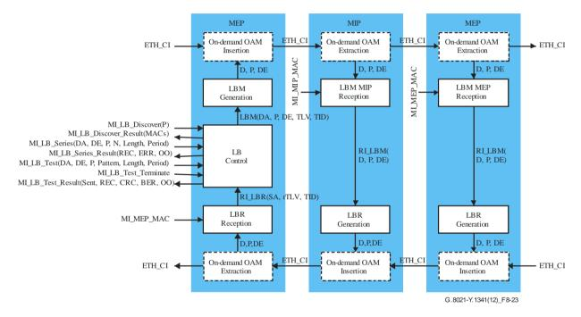
Figure 8-23 – Overview of processes involved with loopback
