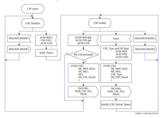
Figure 8-101 – CSF insert behaviour
