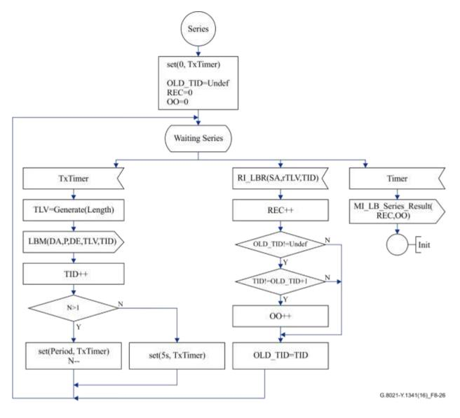
Figure 8-26 – LB control series behaviour
