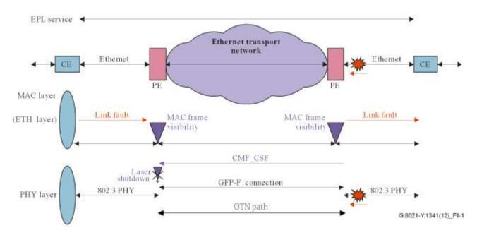
**Figure II.1 – Fault on ingress**
