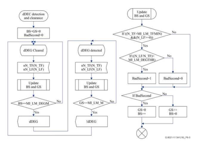
Figure 6-3 – dDEG detection and clearance process
