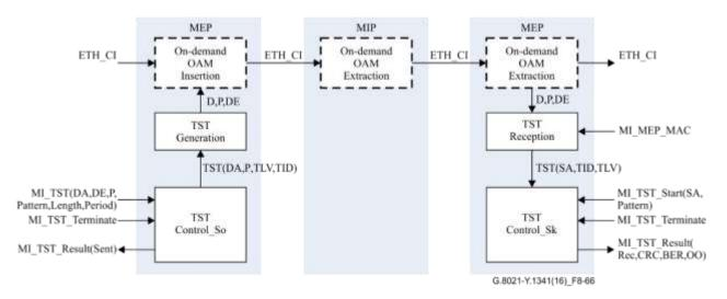
Figure 8-66 – Overview of processes involved with the test protocol
