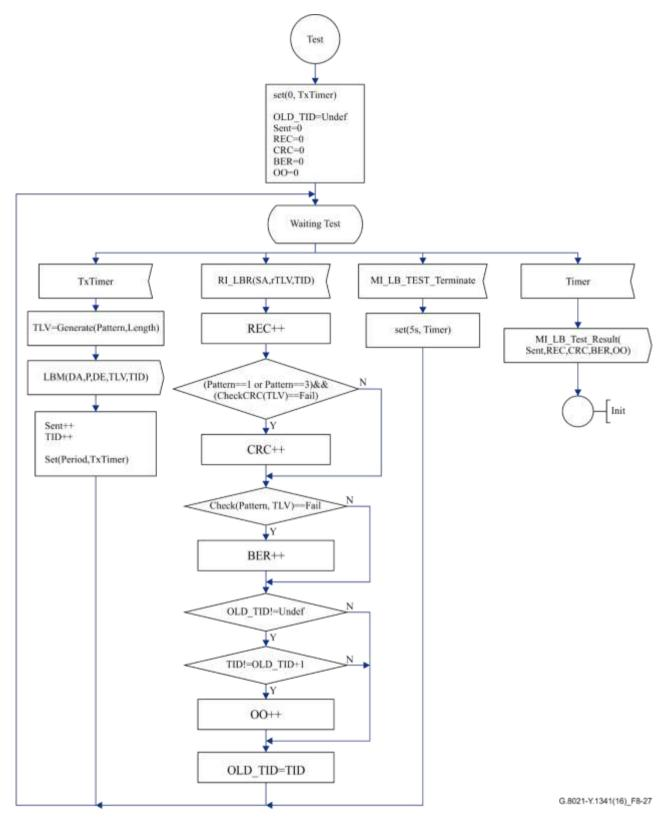
Figure 8-27 – LB control test behaviour
