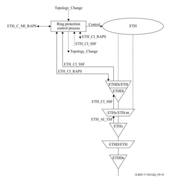
Figure 9-10 – Ring protection atomic functions and control process
