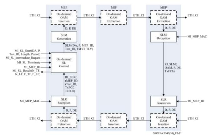
Figure 8-81 – Overview of processes involved with an on-demand single-ended synthetic loss measurement protocol
