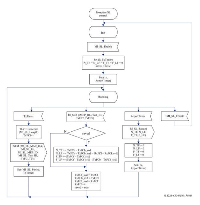
Figure 8-84 – Proactive SL control behaviour
