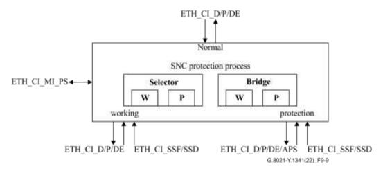
Figure 9-9 – SNC/S protection process
