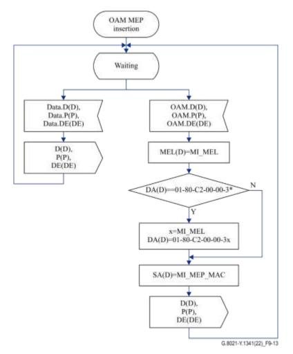
Figure 9-13 – OAM MEP insertion behaviour
