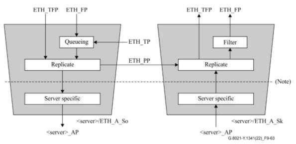
NOTE - This dashed line is shown for reference only. It corresponds to the ISS interface in the [IEEE 802.1Q] model.
