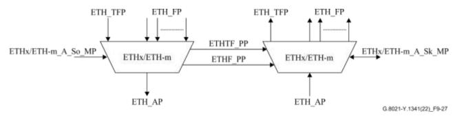
Figure 9-27 – ETHx/ETH-m\_A source and sink symbols
