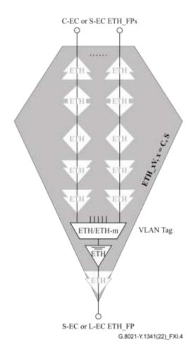
Figure XI.4 – Layer processor to ITU-T G.8021 atomic functions expansion
