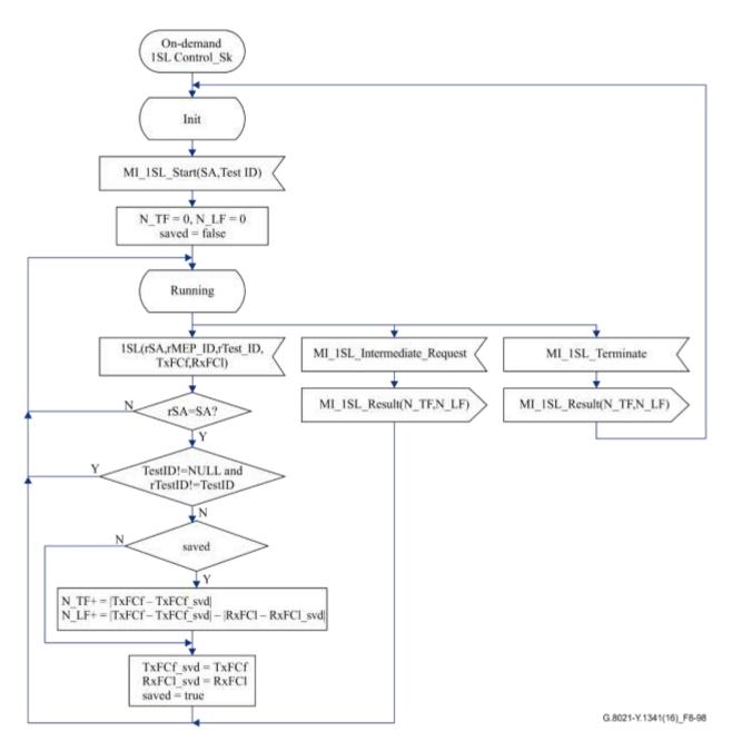
Figure 8-98 – On-demand 1SL Control\_Sk process
