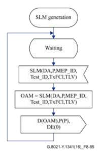
Figure 8-85 – SLM generation behaviour
