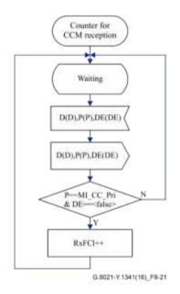
Figure 8-21 – Counter behaviour for CCM reception
