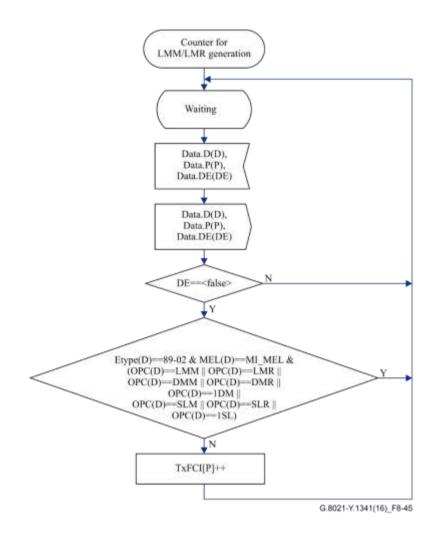
Figure 8-45 – Counter behaviour for LMM/LMR generation
