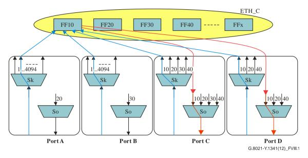
Figure VIII.1 – Example of configuration for ingress VID filtering
