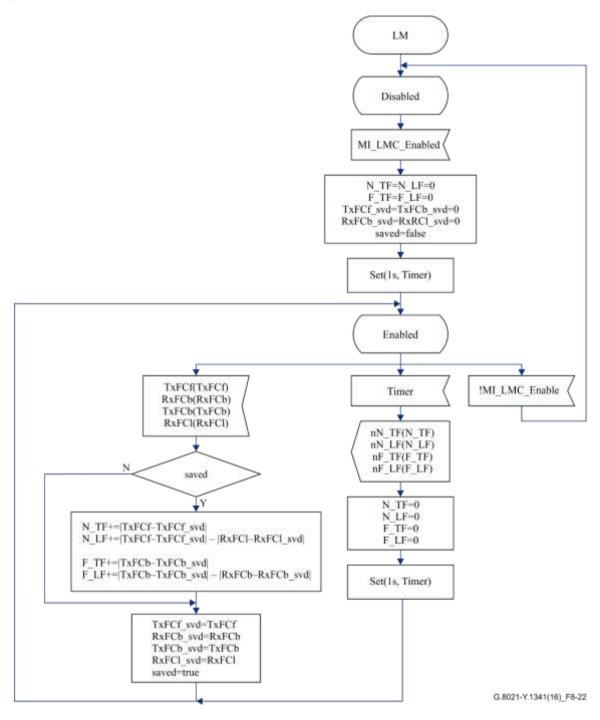
Figure 8-22 – LM process behaviour
