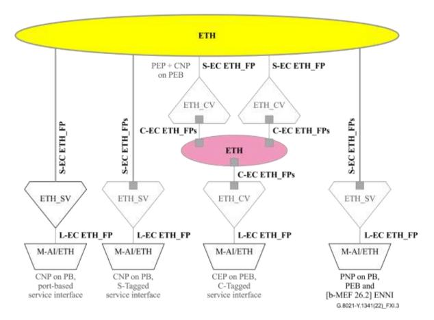
Figure XI.3 – Layer processor-based model for basic ETH equipment types
