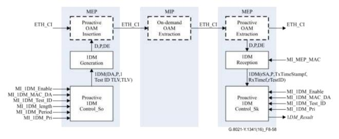
Figure 8-58 – Overview of processes involved with proactive dual-ended delay measurement
