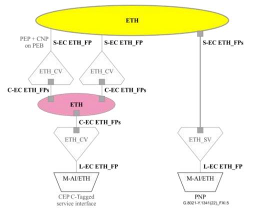
Figure XI.5 – PEB – layer processor and edge processor functions
