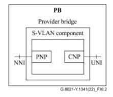
Figure XI.2 – Provider bridge (PB)
