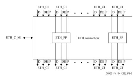
Figure 9-6 – ETH connection function with ETH\_FF processes
