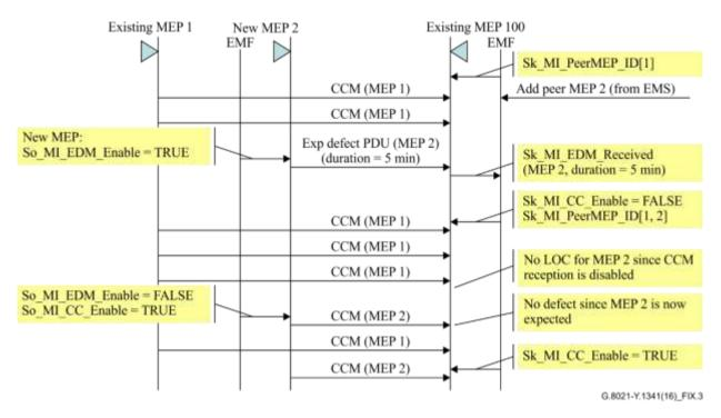
Figure IX.3 – Example showing EDM used to handle a new MEP
