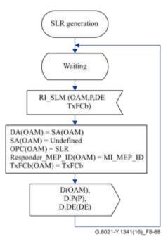
Figure 8-88 – SLR generation behaviour
