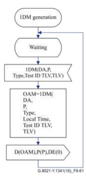
Figure 8-61 – 1DM generation behaviour
