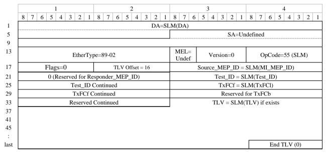
Figure 8-86 – SLM traffic unit
