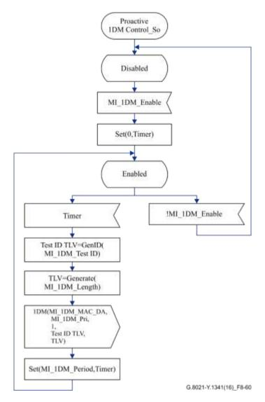
Figure 8-60 – Proactive 1DM Control\_So behaviour
