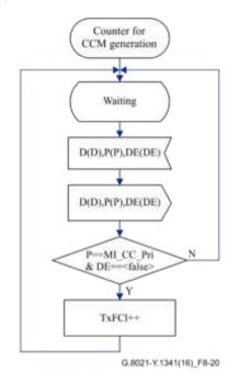
Figure 8-20 – Counter behaviour for CCM generation
