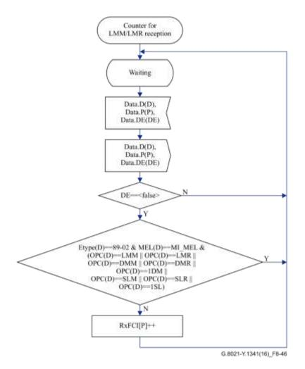
Figure 8-46 – Counter behaviour for LMM/LMR reception
