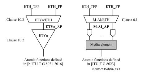
Figure X.1 – Mapping between ETYn/ETH and M-AIETH adaptation functions
