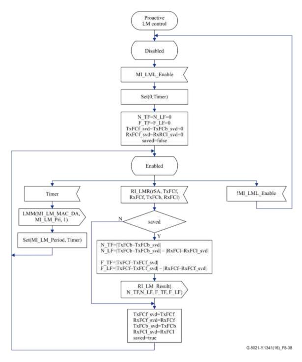
Figure 8-38 – Proactive LM control behaviour
