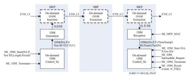
Figure 8-57 - Overview of processes involved with on-demand dual-ended delay measurement
