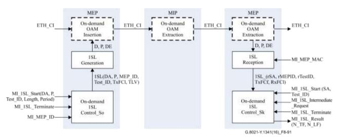
Figure 8-91 – Overview of processes involved with on-demand dual-ended synthetic loss measurement
