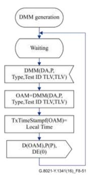
Figure 8-51 – DMM generation behaviour
