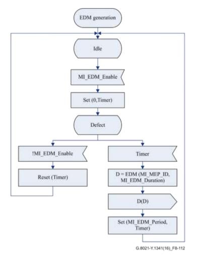
Figure 8-112 – EDM Generation behaviour
