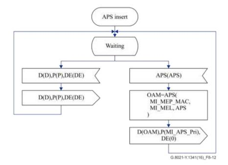
Figure 8-12 – APS insert behaviour
