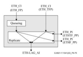
Figure 9-75 – ETH-LAG/ETH\_A\_So process
