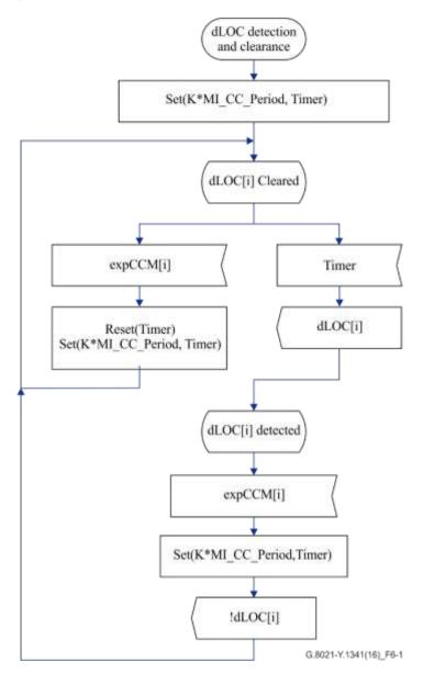
Figure 6-1 – dLOC[] detection and clearance process
