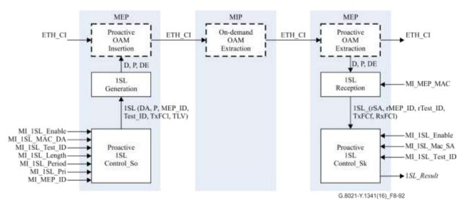
Figure 8-92 – Overview of processes involved with proactive dual-ended synthetic loss measurement
