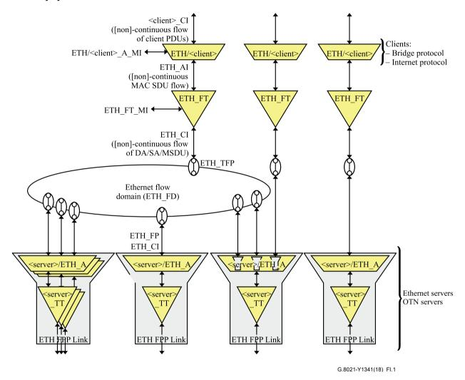
Figure I.1 – Ethernet atomic functions in several possible applications
