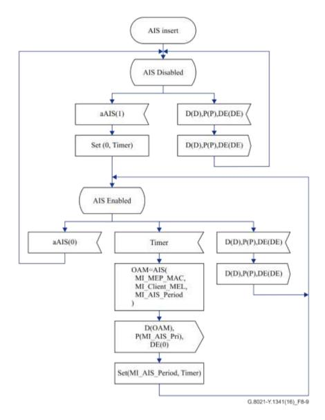
Figure 8-9 – AIS insert behaviour
