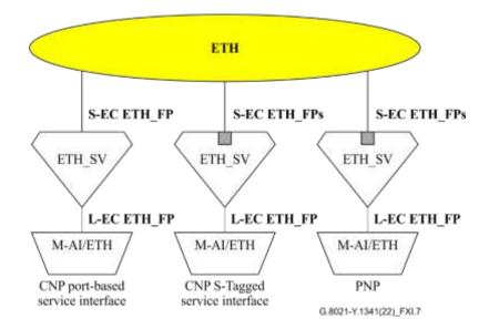
Figure XI.7 – PB – layer processor and edge processor functions
