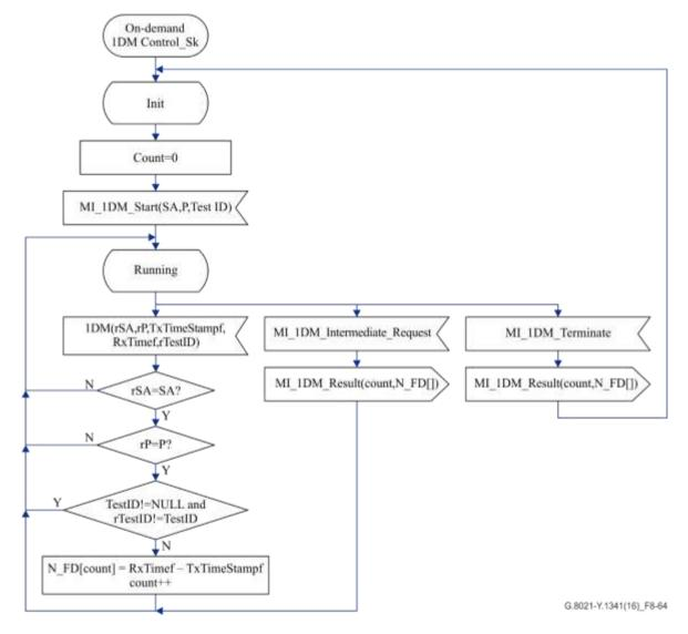
Figure 8-64 – On-demand 1DM Control\_Sk process
