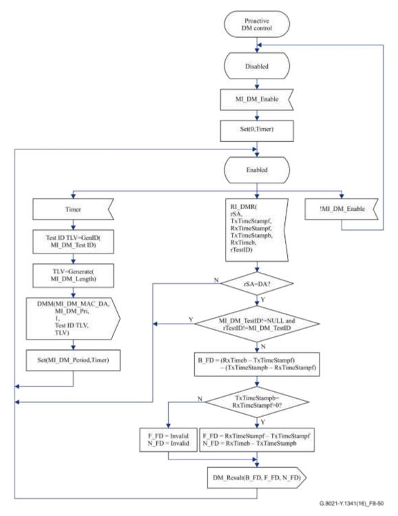
Figure 8-50 – Proactive DM control behaviour
