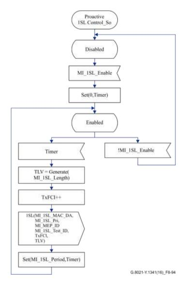
Figure 8-94 – Proactive 1SL Control\_So behaviour
