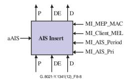
Figure 8-8 – AIS insert process
