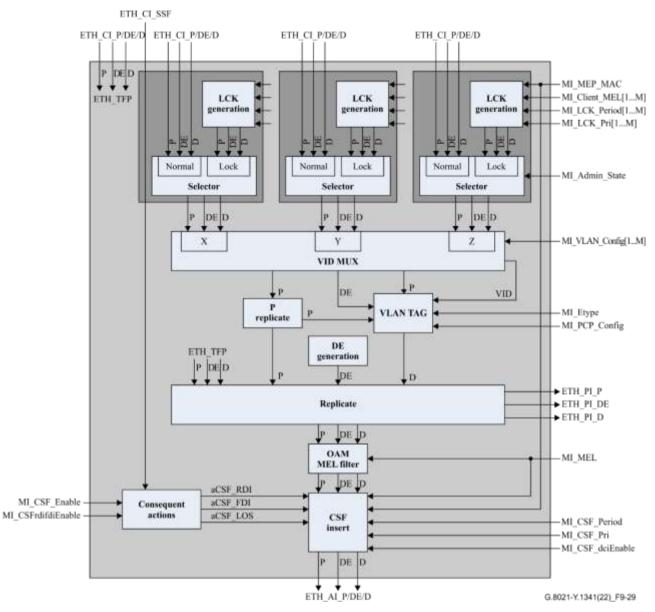
Figure 9-29 – ETHx/ETH-m\_A\_So process
