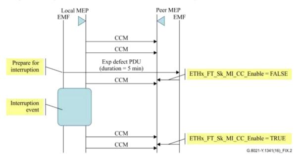
Figure IX.2 – Example showing EDM used to handle an interruption event
