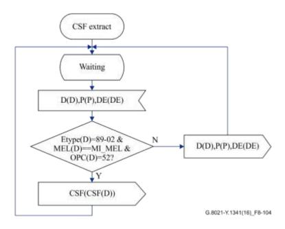
Figure 8-104 – CSF extract behaviour
