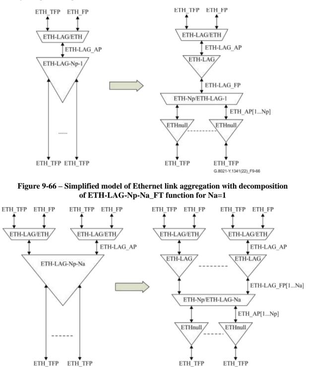
Figure 9-67 – Generic model of Ethernet link aggregation with decomposition of ETH-LAG-Np-Na\_FT function
