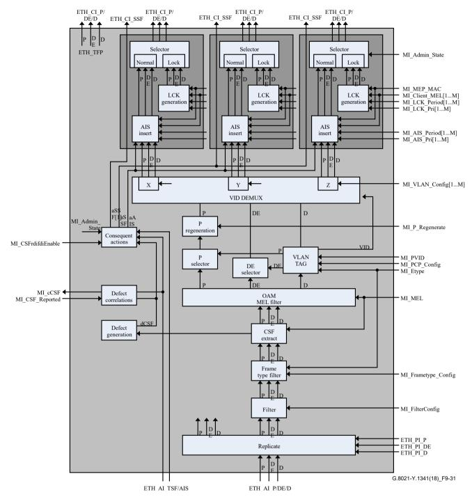
Figure 9-31 – ETHx/ETH-m\_A\_Sk process
