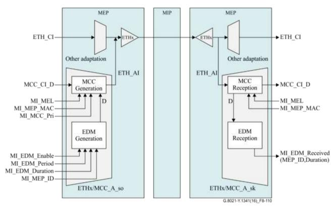
**Figure 8-110 – Overview of Expected Defect processes**
