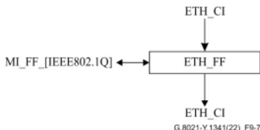
**Figure 9-7 – ETH flow forwarding process**
