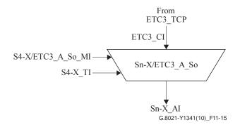
Figure 11-15 - Sn-X/ETC3\_A\_So symbol
