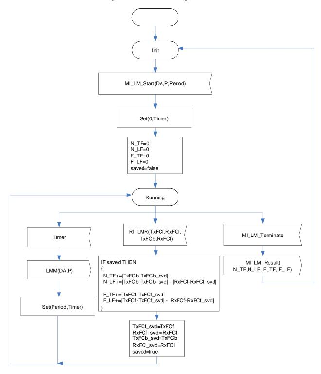
Figure 8-34 – LM Control behaviour
