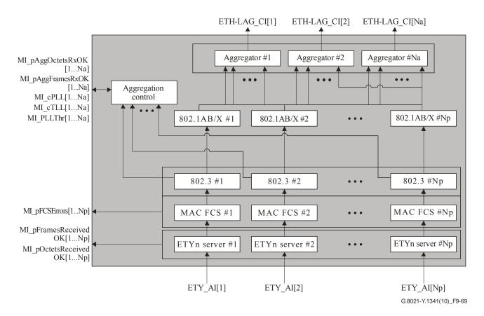
Figure 9-69 – ETY-Np/ETH-LAG-Na\_A\_Sk process
