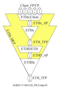
Figure III.2 – Expanded MEP compound function
