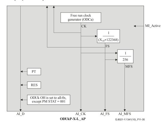
Figure 11-35 – ODUkP-X-L specific source process
