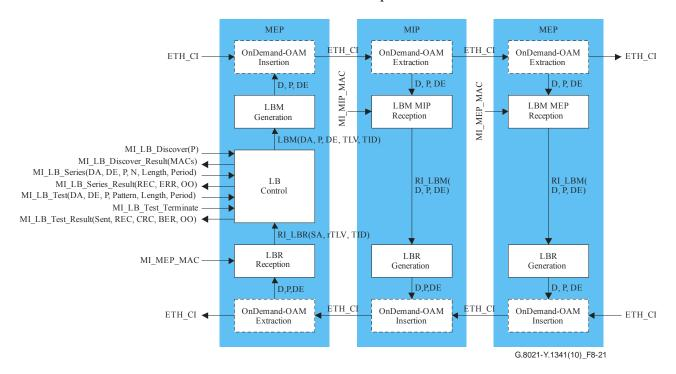
Figure 8-21 – Overview of processes involved with Loopback
