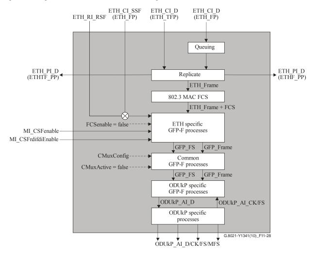
Figure 11-28 – ODUkP/ETH\_A\_So process
