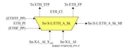
Figure 11-7 – Sn-X-L/ETH\_A\_Sk symbol
