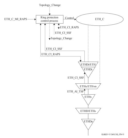
Figure 9-11 – Ring protection atomic functions and control process
