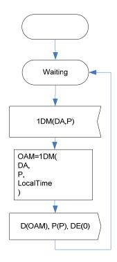
Figure 8-51 – 1DM Generation behaviour
