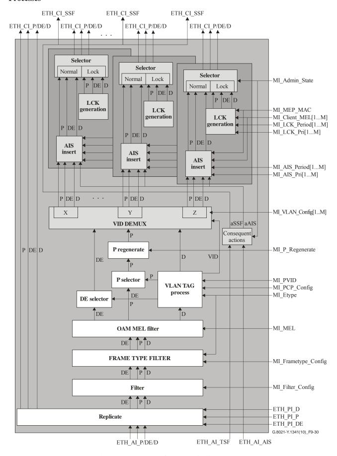
Figure 9-30 – ETHx/ETH-m\_A\_Sk process
