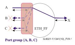
Figure VII.1 – Principle of operation of the port group function
