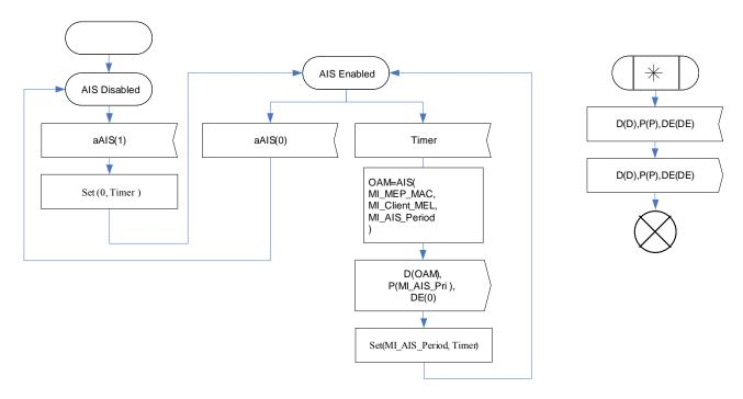
Figure 8-9 – AIS Insert behaviour
