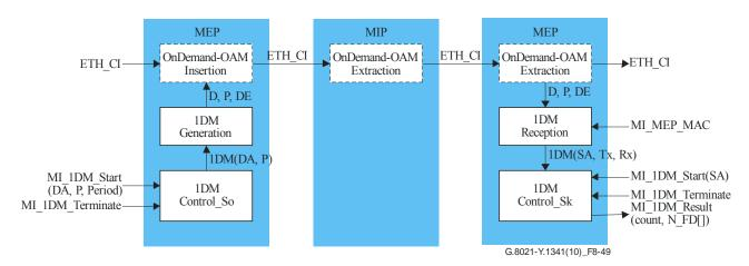
Figure 8-49 – Overview of processes involved with one-way delay measurement
