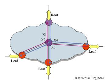
Figure VII.4 – Application example of the asymmetric VLANs
