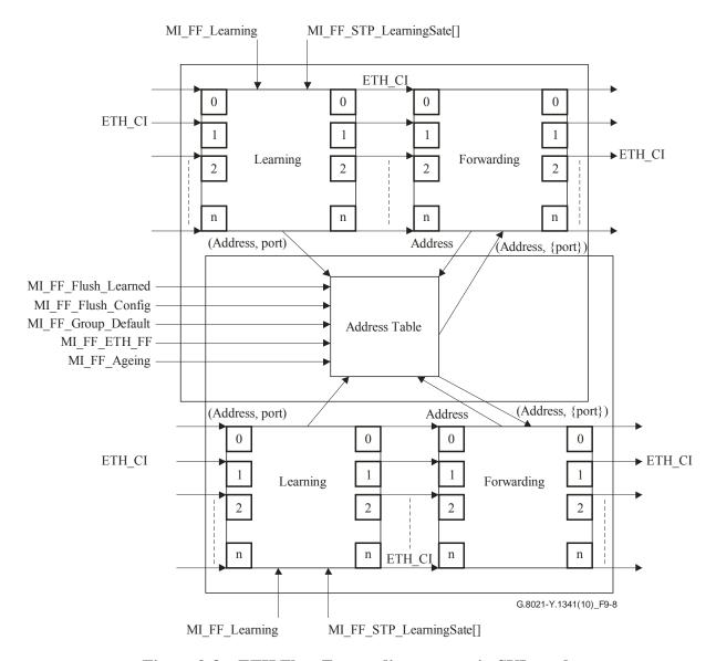
Figure 9-8 – ETH Flow Forwarding process in SVL mode
