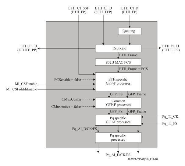
Figure 11-20 - Pq/ETH\_A\_So process
