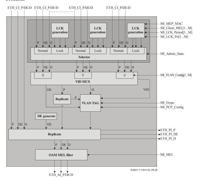
Figure 9-28 – ETHx/ETH-m\_A\_So process
