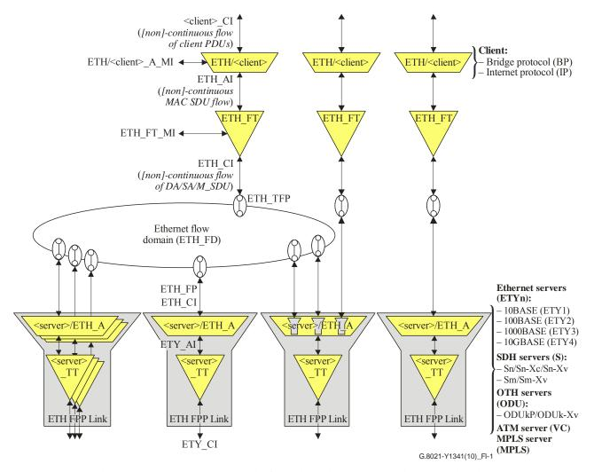
Figure I.1 – Ethernet atomic functions in some possible applications
