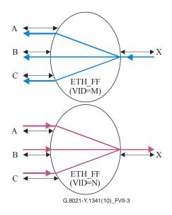
Figure VII.3 – Principle of the asymmetric VLANs
