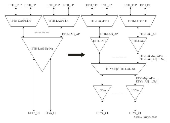
Figure 9-65 – Generic model of Ethernet link aggregation with decomposition of ETH-LAG-Np-Na TT function
