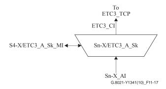
Figure 11-17 – Sn-X/ETC3\_A\_Sk symbol
