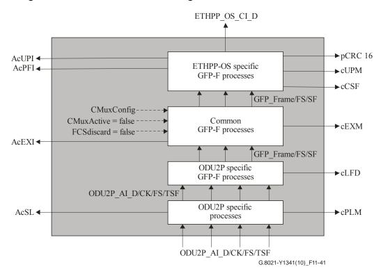
Figure 11-41 – ODU2P/ETHPP-OS\_A\_Sk process
