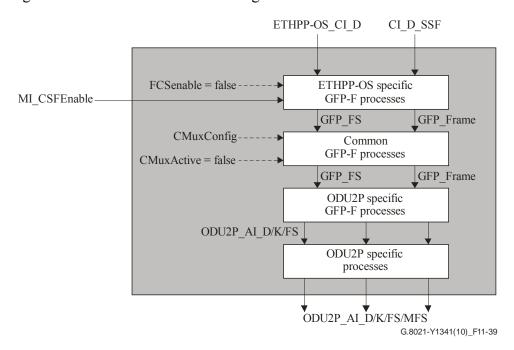
Figure 11-39 – ODU2P/ETHPP-OS\_A\_So process
