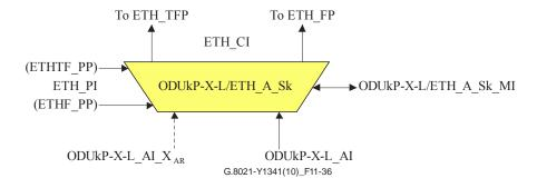
Figure 11-36 – ODUkP-X-L/ETH\_A\_Sk symbol
