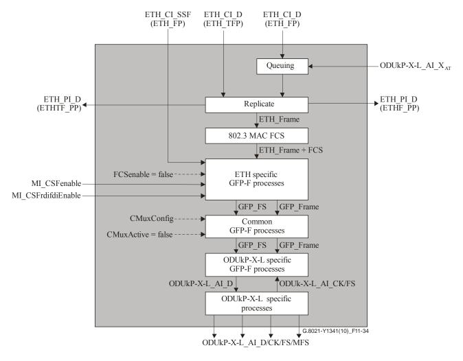
Figure 11-34 – ODUkP-X-L/ETH\_A\_So process
