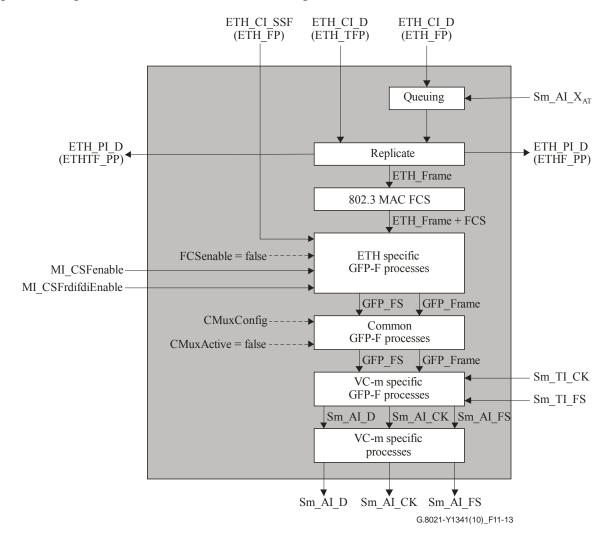
Figure 11-13 – Sm-X-L/ETH\_A\_So process
