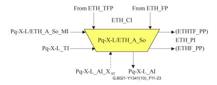
Figure 11-23 - Pq-X-L/ETH\_A\_So symbol
