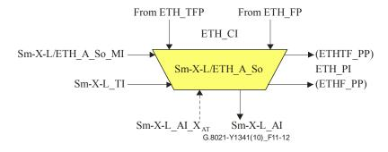
Figure 11-12 – Sm-X-L/ETH\_A\_So symbol
