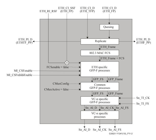
Figure 11-2 – Sn/ETH\_A\_So process
