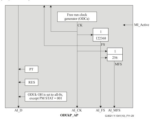
Figure 11-29 – ODUkP specific source process
