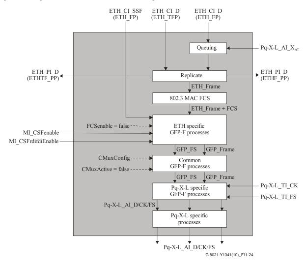
Figure 11-24 – Pq-X-L/ETH\_A\_So process
