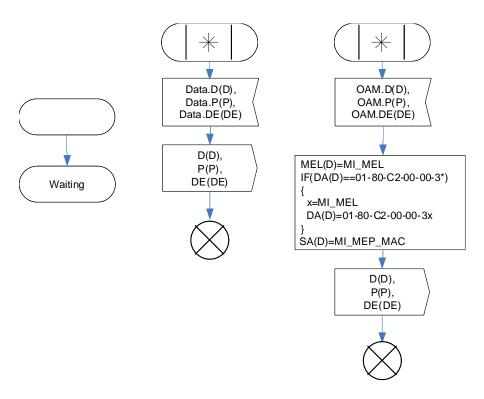
Figure 9-14 – OAM MEP insertion behaviour
