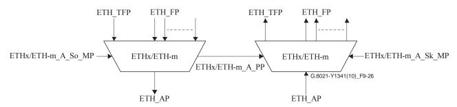
Figure 9-26 – ETHx/ETH-m\_A Source and Sink symbols
