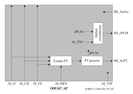
Figure 11-32 – ODUkP specific sink process
