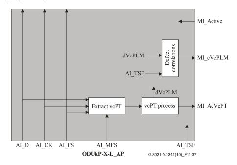
Figure 11-37 – ODUkP-X-L specific sink process
