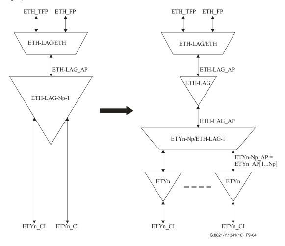
Figure 9-64 – Simplified model of Ethernet link aggregation with decomposition of ETH-LAG-Np-Na\_TT function for Na=1
