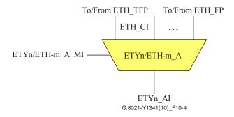
Figure 10-4 – ETYn Server to ETH-m adaptation function
