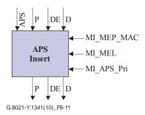
Figure 8-11 – APS Insert process
