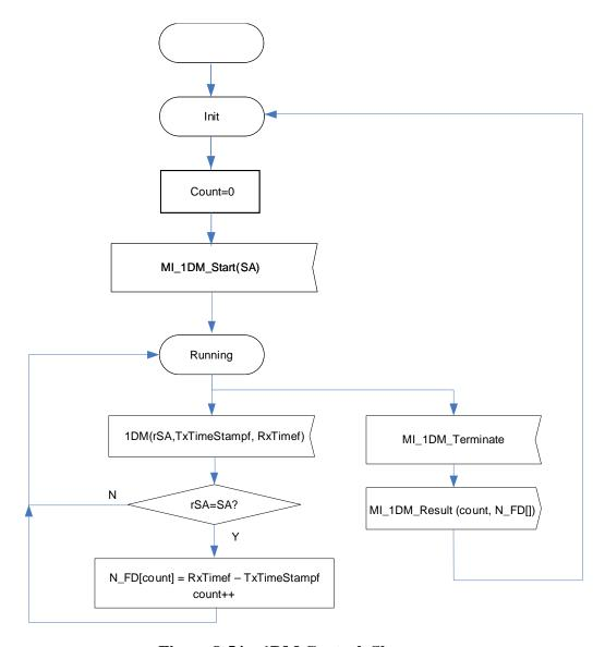
Figure 8-54 – 1DM Control\_Sk process
