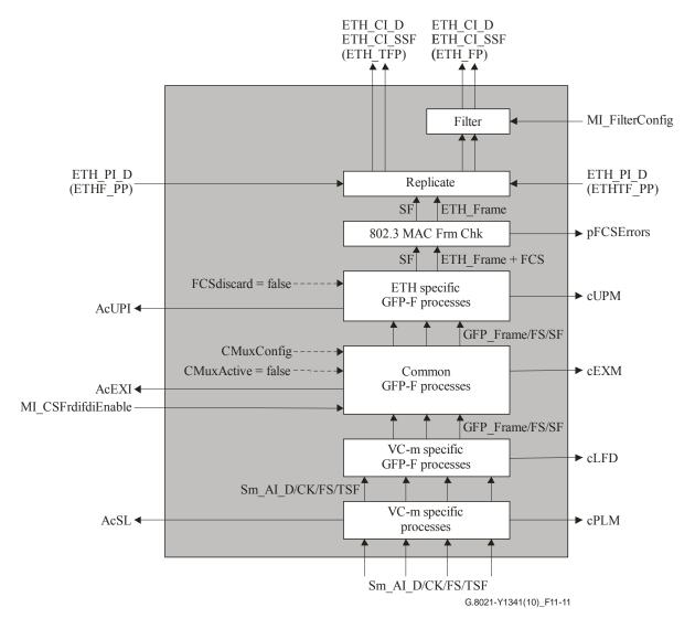
Figure 11-11 – Sm/ETH\_A\_Sk process
