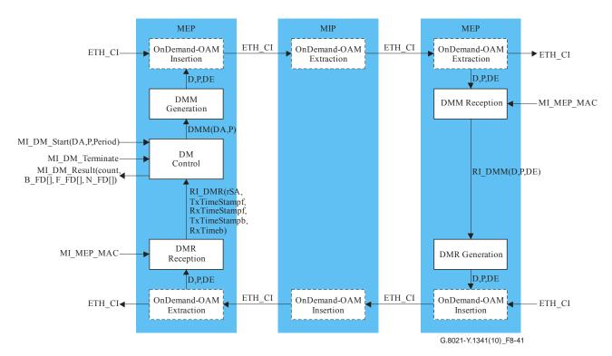
Figure 8-41 – Overview of processes involved with delay measurement
