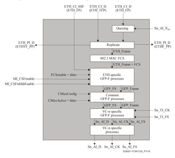
Figure 11-6 – Sn-X-L/ETH\_A\_So process
