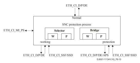
Figure 9-10 – SNC/S Protection process
