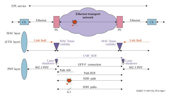
Figure II.2 – Fault within carrier network
