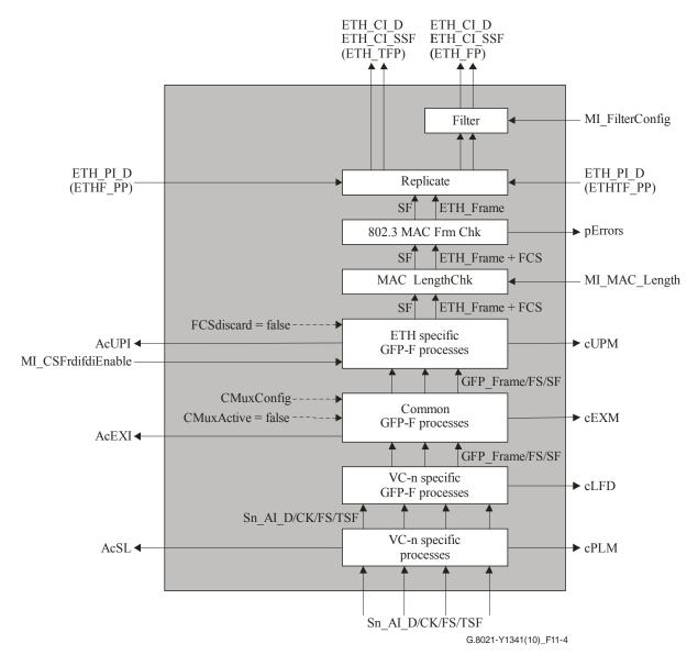
Figure 11-4 – Sn/ETH\_A\_Sk process
