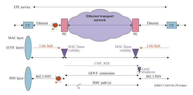
Figure II.3 – Fault on egress
