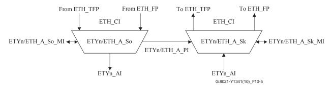
Figure 10-5 – ETYn/ETH\_A Source and Sink adaptation functions
