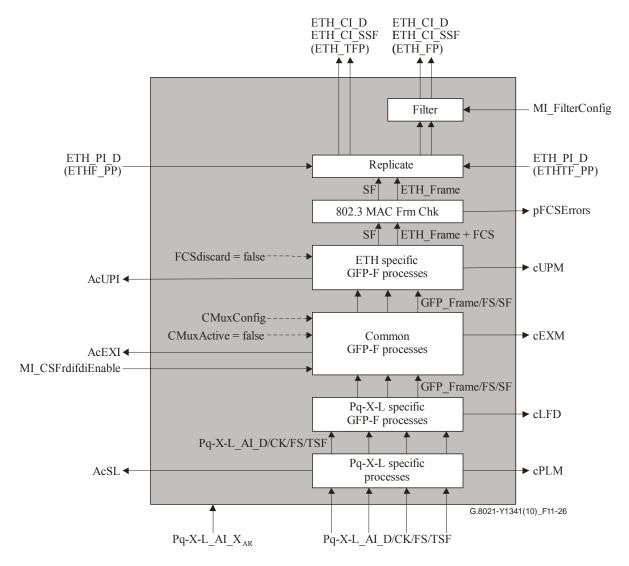
Figure 11-26 – Pq-X-L/ETH\_A\_Sk process
