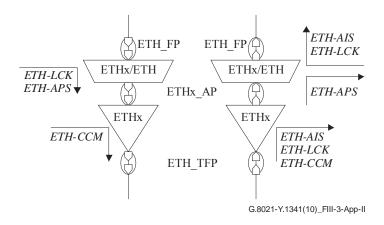
Figure III.3 – ETH path, tandem connection, section flow termination function and adaptation
