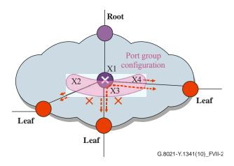
Figure VII.2 – Application example of the port group function
