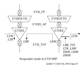
Figure III.8 – ETH diagnostic adaptation and flow termination function for MIPs
