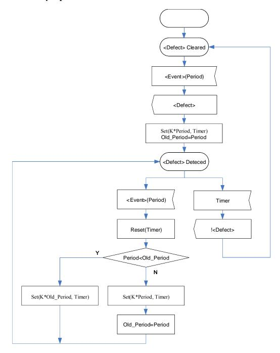
Figure 6-2 – Defect detection and clearance process for dUNL, dMMG, dUNM, dUNP, dUNPr, dAIS, dLCK
