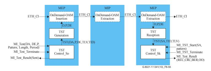
Figure 8-55 – Overview of processes involved with Test protocol
