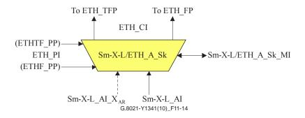
Figure 11-14 – Sm-X-L/ETH\_A\_Sk symbol
