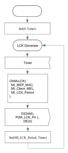
Figure 8-4 – LCK Generation process behaviour
