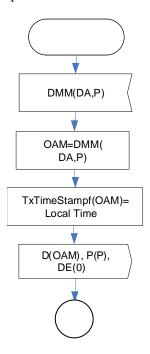
Figure 8-43 – DMM Generation behaviour
