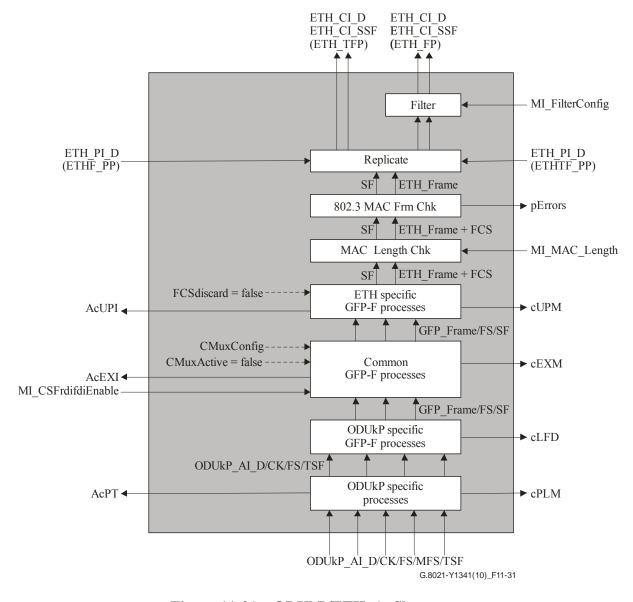
Figure 11-31 – ODUkP/ETH\_A\_Sk process
