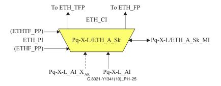
Figure 11-25 – Pq-X-L/ETH\_A\_Sk symbol
