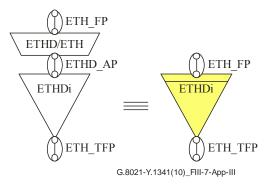
Figure III.7 – ETH half MIP compound function
