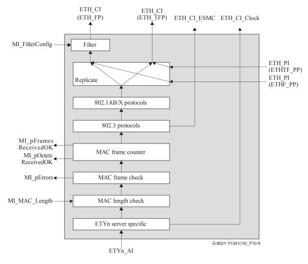
Figure 10-9 - ETYn/ETH\_A\_Sk process
