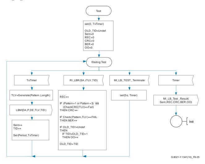
Figure 8-25 – LB Control Test behaviour
