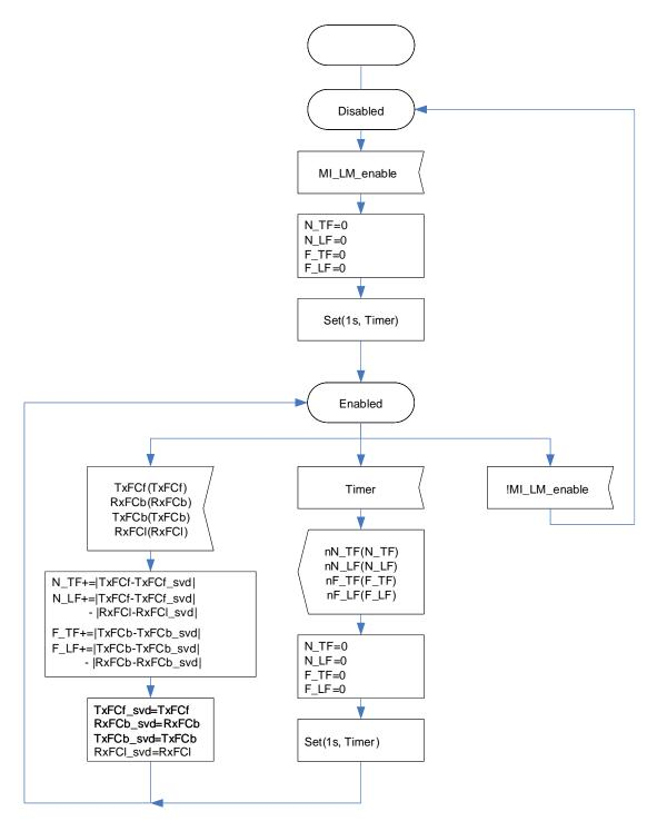
Figure 8-20 – LM process behaviour
