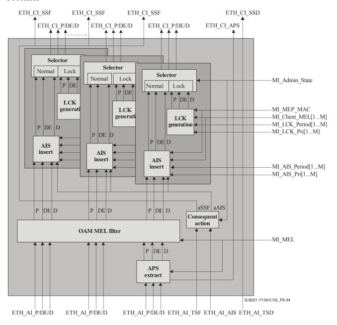
Figure 9-34 – ETHG/ETH\_A\_Sk process
