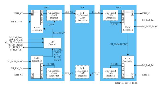
Figure 8-33 – Overview of processes involved with loss measurement
