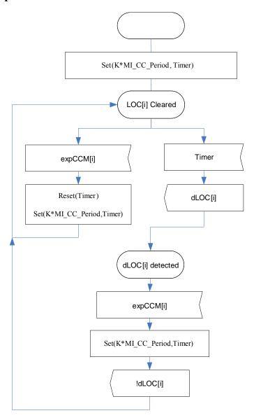
Figure 6-1 – dLOC[] detection and clearance process
