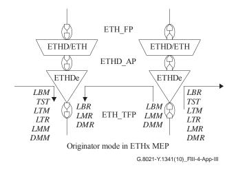
Figure III.4 – ETH diagnostic adaptation and flow termination function for MEPs
