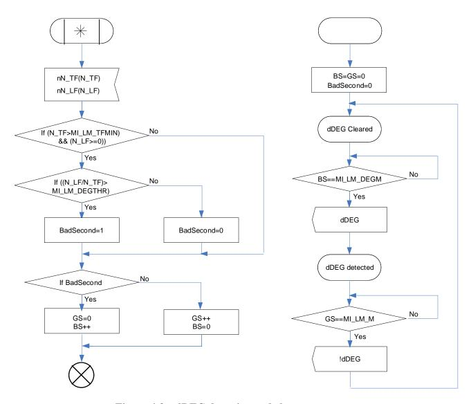
Figure 6-3 – dDEG detection and clearance process
