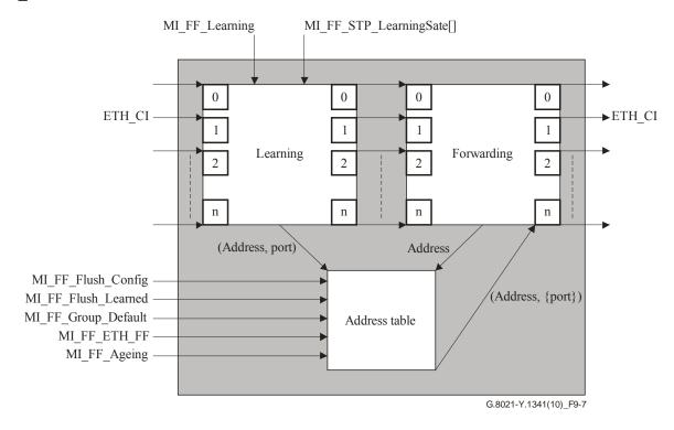
Figure 9-7 – ETH Flow Forwarding process
