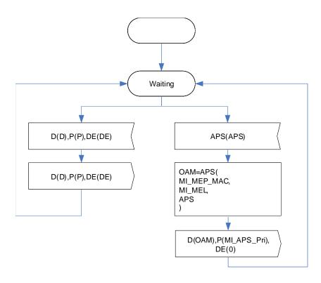
Figure 8-12 – APS Insert behaviour
