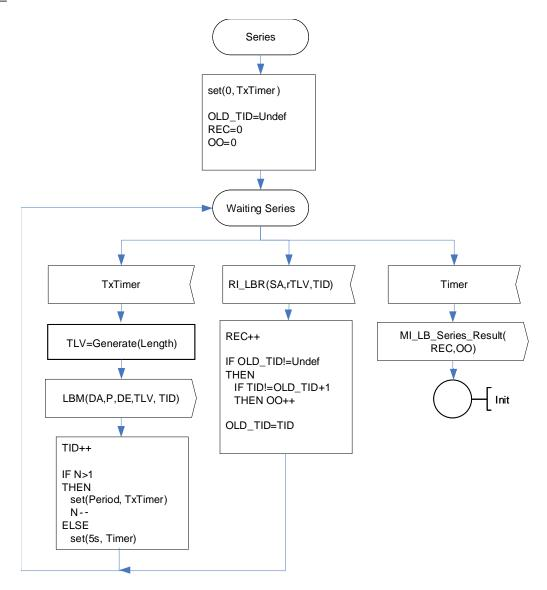
Figure 8-24 – LB Control Series behaviour
