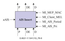
Figure 8-8 – AIS Insert process
