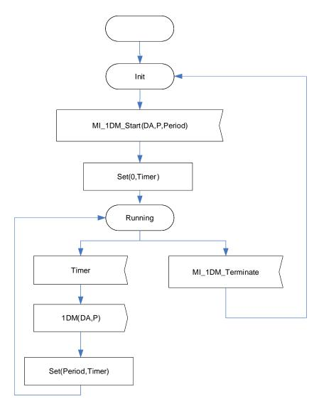
Figure 8-50 – 1DM Control\_So behaviour
