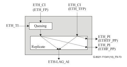
Figure 9-73 – ETH-LAG/ETH\_A\_So process
