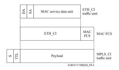
Figure A.2 – MPLS link header without common interworking indicators and with MAC FCS preservation
