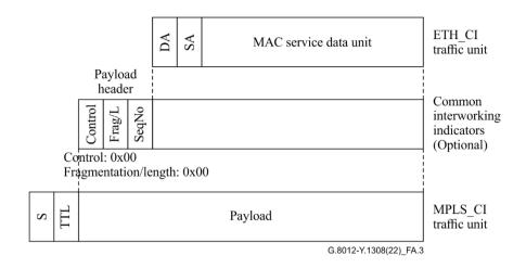
Figure A.3 – MPLS link header with common interworking indicators and without MAC FCS preservation
