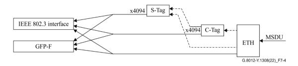
Figure 7-4 – Ethernet two-level multiplexing
