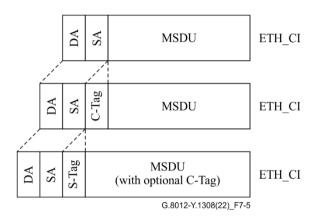
Figure 7-5 – Ethernet two-level multiplexing method
