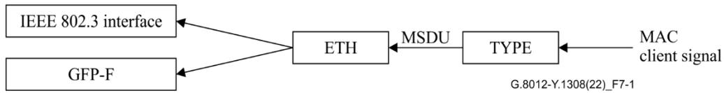
**Figure 7-1 – Ethernet mapping and multiplexing**
