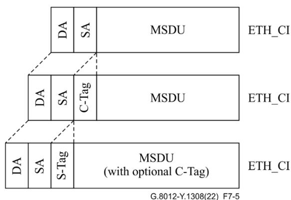
**Figure 7-5 – Ethernet two-level multiplexing method**
