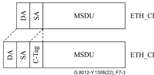
**Figure 7-3 – Ethernet single level multiplexing method**
