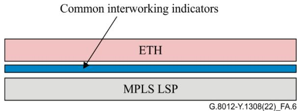
**Figure A.6 – Components of Ethernet over MPLS with common interworking indicators**
