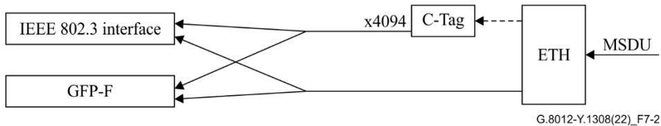
**Figure 7-2 – Ethernet single level multiplexing**
