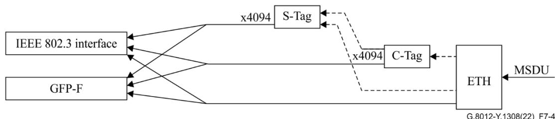
**Figure 7-4 – Ethernet two-level multiplexing**
