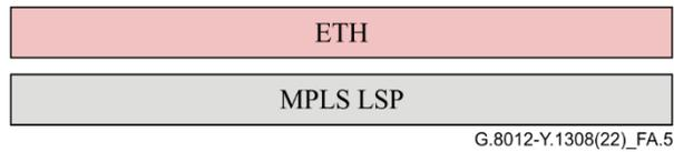
**Figure A.5 – Components of Ethernet over MPLS without common interworking indicators**
