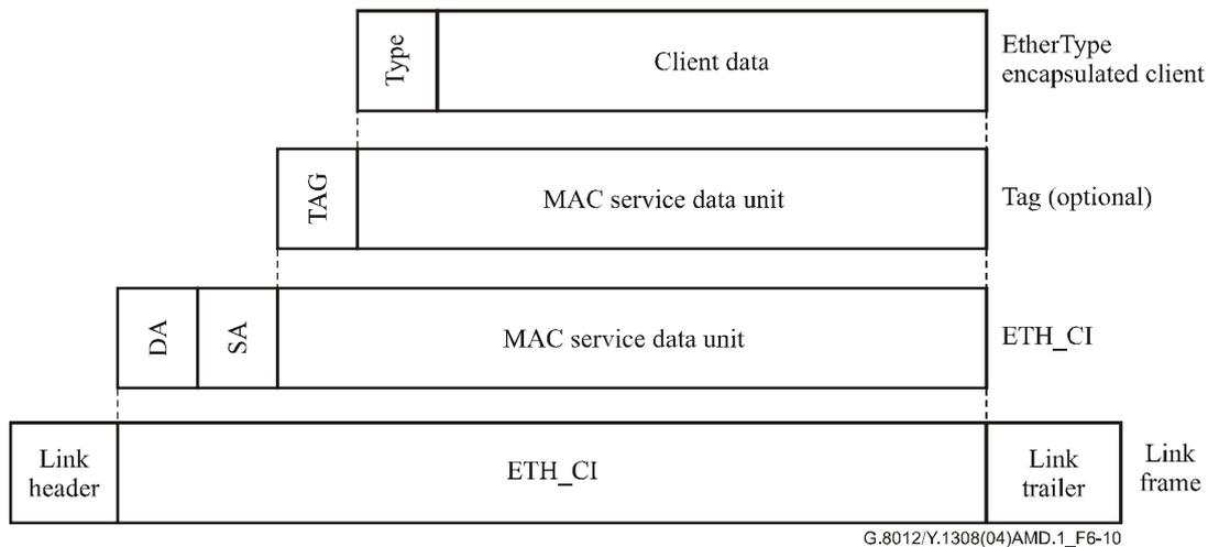
**Figure 6-10/G.8012/Y.1308 – Ethernet principle information containment**
