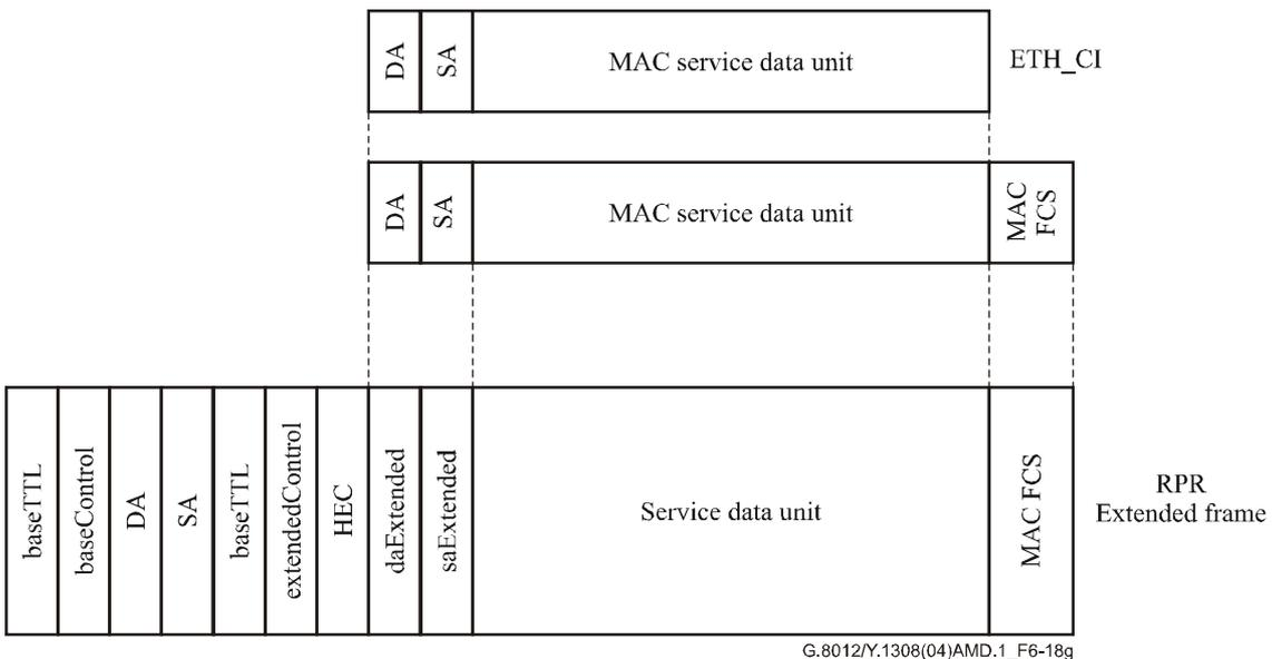
**Figure 6-18g/G.8012/Y.1308 – Extended type 2 RPR link frame**
