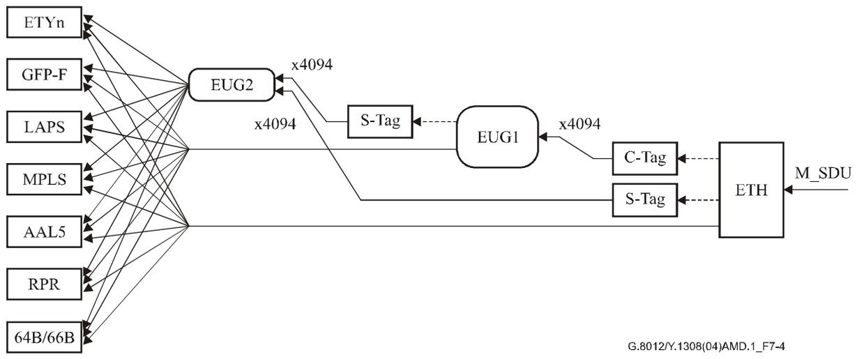
**Figure 7-4/G.8012/Y.1308 – Ethernet two-level multiplexing**
