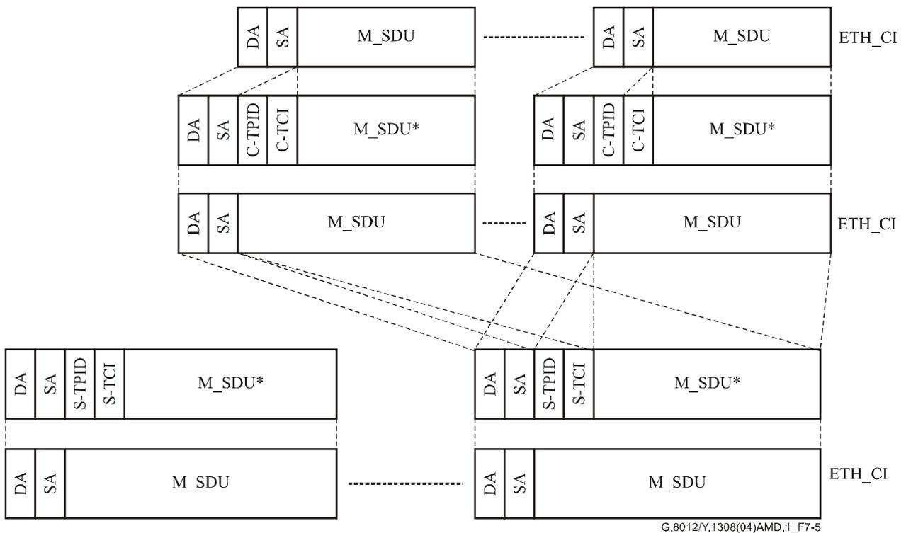
**Figure 7-5/G.8012/Y.1308 – Ethernet two-level multiplexing method**
