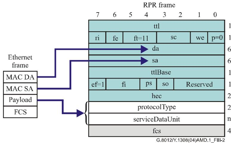
Figure III.2/G.8012/Y.1308 – Mapping Ethernet frame into 802.17 basic frame
