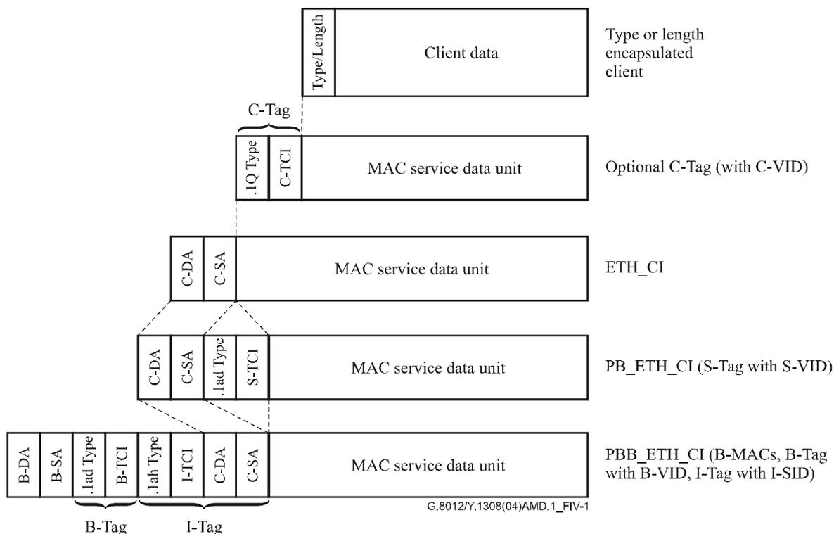
**Figure IV.1/G.8012/Y.1308 – PBB Ethernet principle information containment for a one-to-one mapped S-tagged service interface**
