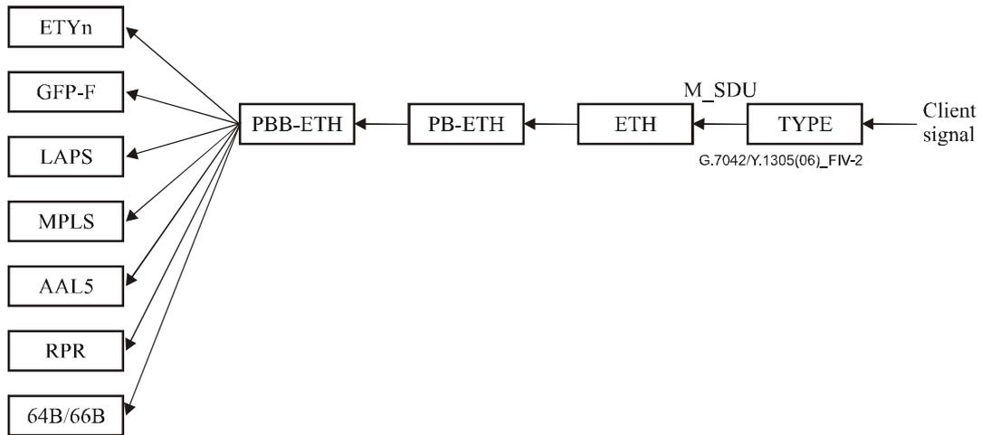
**Figure IV.2/G.8012/Y.1308 – Ethernet mapping and multiplexing with PB and PBB**
