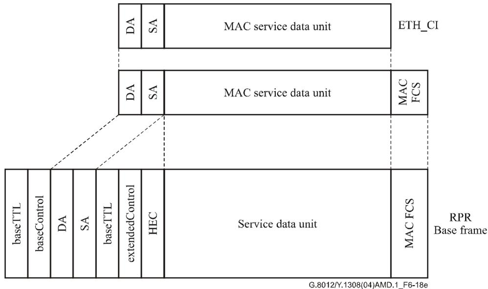
Figure 6-18e/G.8012/Y.1308 – Basic RPR link frame
