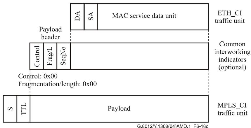
**Figure 6-18c/G.8012/Y.1308 – MPLS link header with common interworking indicators and without MAC FCS preservation**
