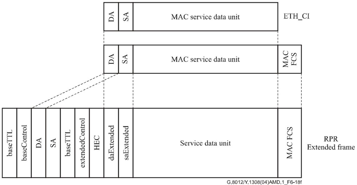
**Figure 6-18f/G.8012/Y.1308 – Extended type 1 RPR link frame**
