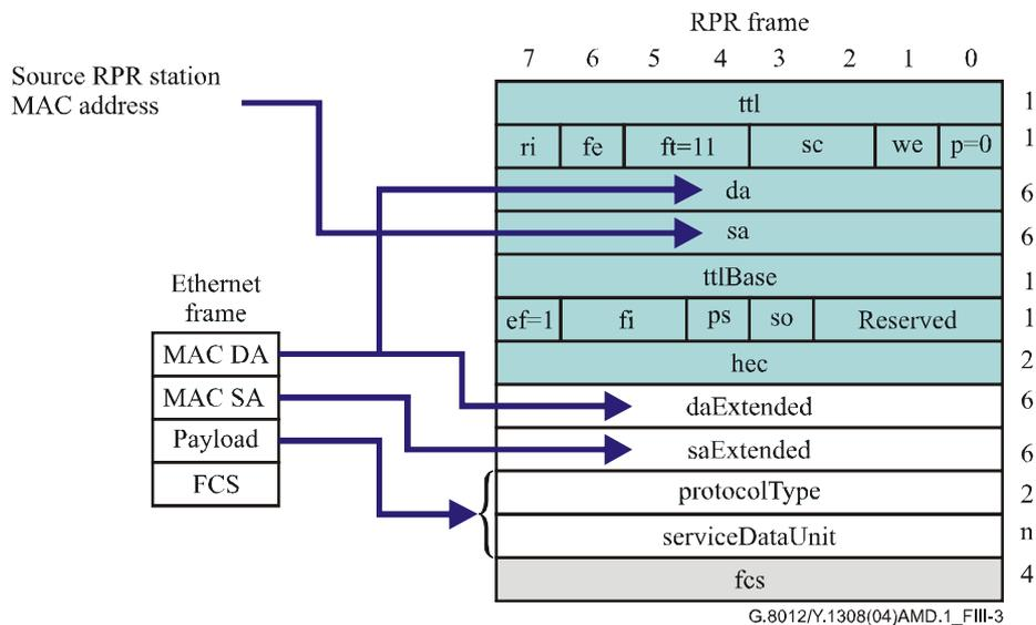
Figure III.3/G.8012/Y.1308 – Mapping Ethernet frame into 802.17 extended frame – Type 1
