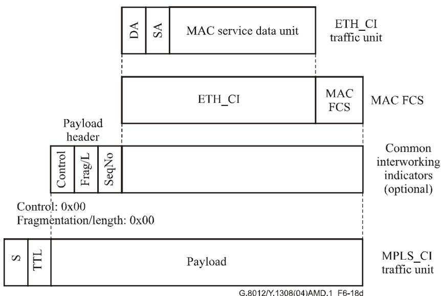
**Figure 6-18d/G.8012/Y.1308 – MPLS link header with common interworking indicators and MAC FCS preservation**
