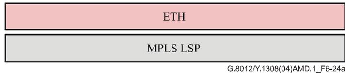
**Figure 6-24a/G.8012/Y.1308 – Components of the Ethernet over MPLS-NNI without common interworking indicators**
