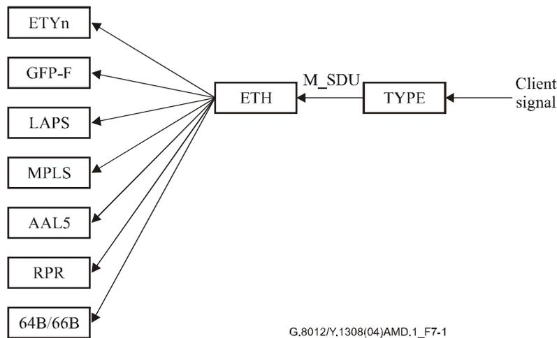
**Figure 7-1/G.8012/Y.1308 – Ethernet mapping and multiplexing**
