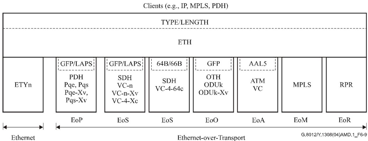
**Figure 6-9/G.8012/Y.1308 – Structure of the ETH interfaces**
