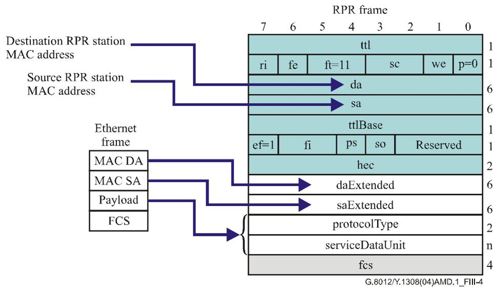
**Figure III.4/G.8012/Y.1308 – Mapping Ethernet frame into 802.17 extended frame – Type 2**
