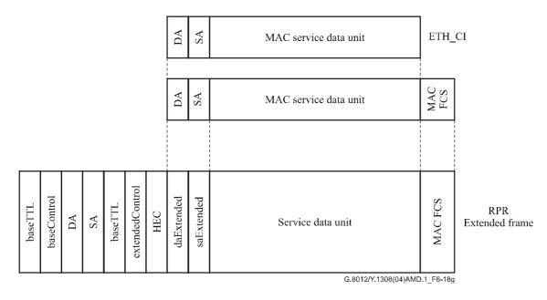
Figure 6-18g/G.8012/Y.1308 – Extended type 2 RPR link frame
