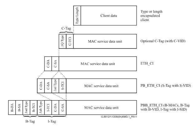
Figure IV.1/G.8012/Y.1308 – PBB Ethernet principle information containment for a one-to-one mapped S-tagged service interface
