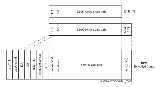
Figure 6-18f/G.8012/Y.1308 – Extended type 1 RPR link frame
