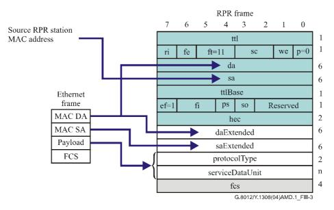
Figure III.3/G.8012/Y.1308 – Mapping Ethernet frame into 802.17 extended frame – Type 1
