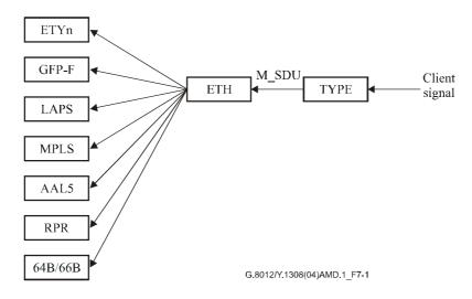
Figure 7-1/G.8012/Y.1308 – Ethernet mapping and multiplexing
