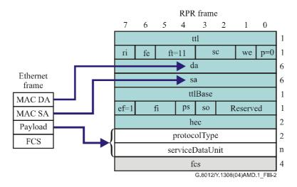
Figure III.2/G.8012/Y.1308 – Mapping Ethernet frame into 802.17 basic frame
