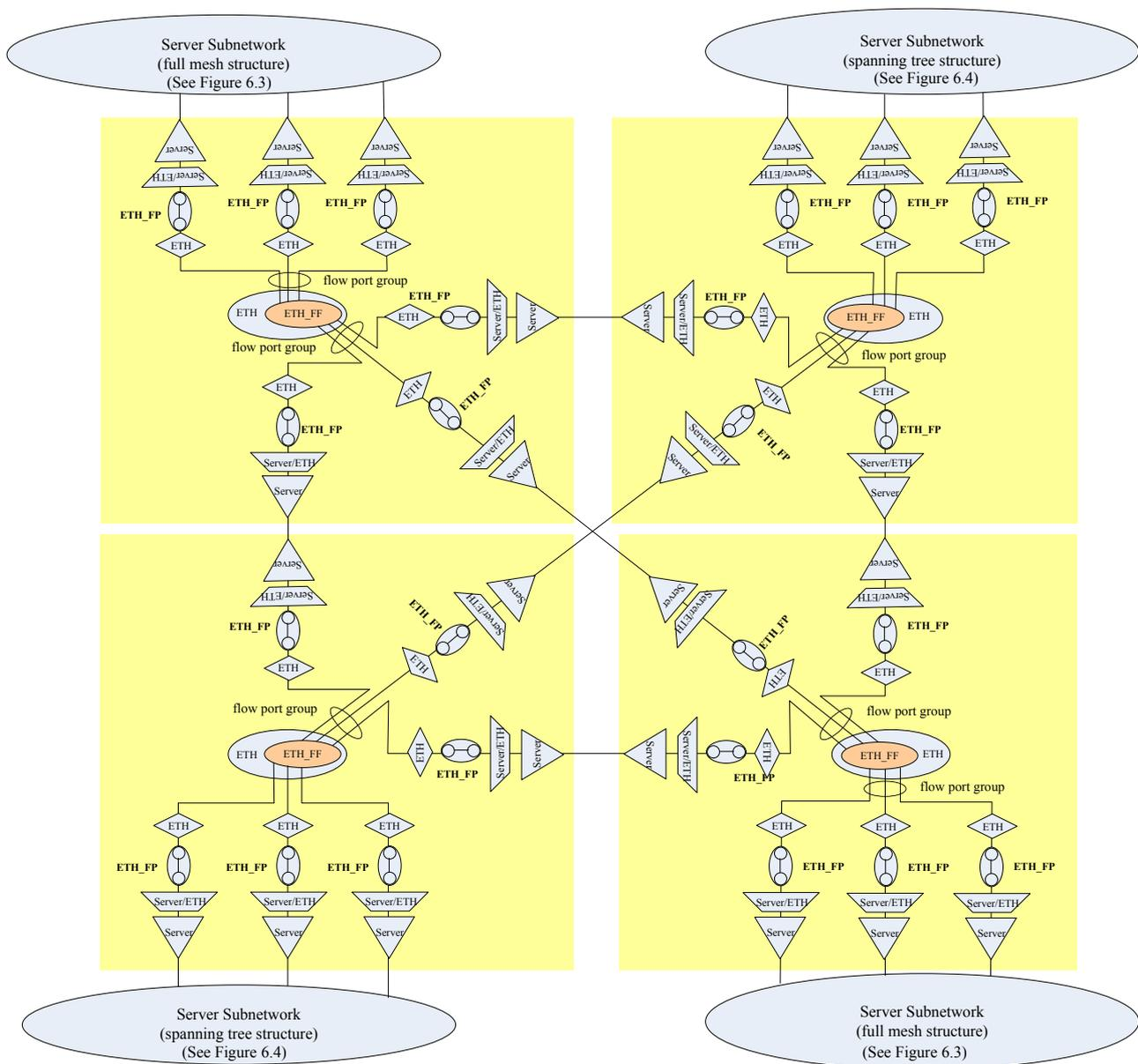
**Figure 6-5 – EPLAN service architecture (full mesh with flow port grouping, multiple domains)**
