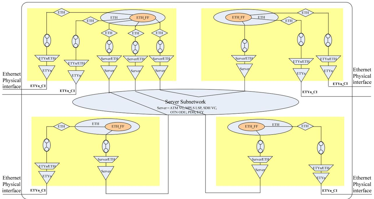
**Figure 6-4 – EPLAN service architecture (spanning tree, single domain)**
