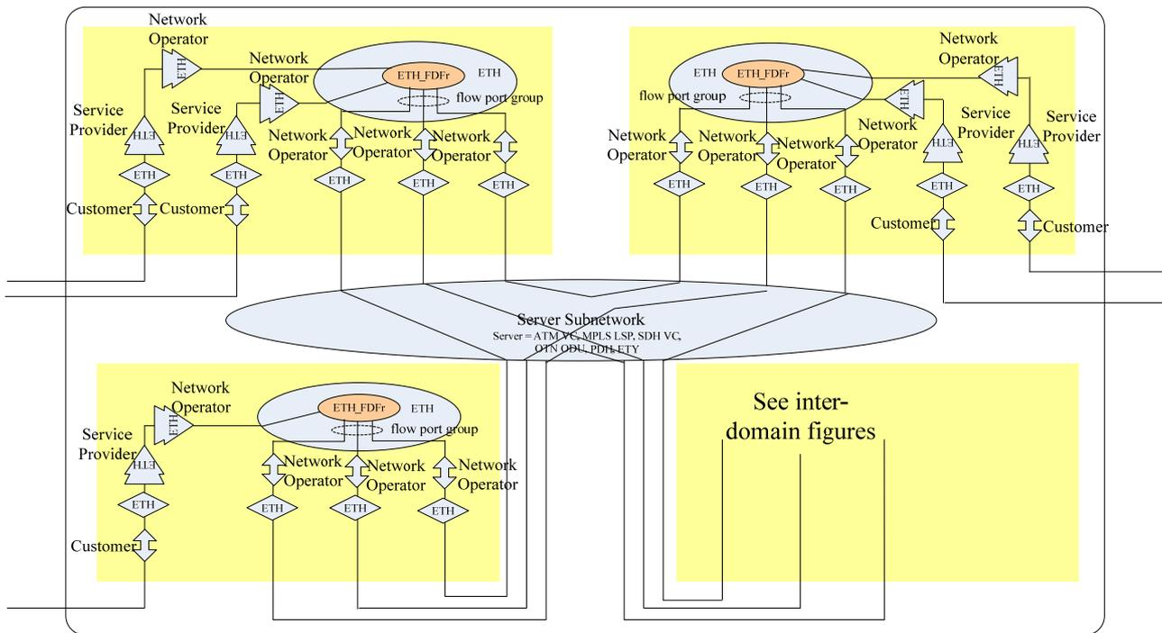
**Figure 7-5 – Basic ETH MEP and MIP functions for the multipoint-to-multipoint Ethernet connection segment within the domain of one transport operator**
