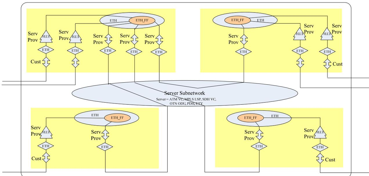
**Figure 7-2 – Basic ETH MEP and MIP functions for the example in Figure 6-4**
