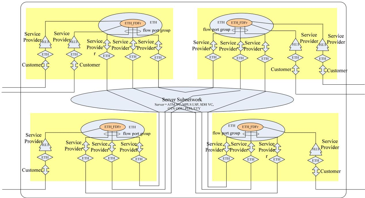
**Figure 7-1 – Basic ETH MEP and MIP functions for the example in Figure 6-3**
