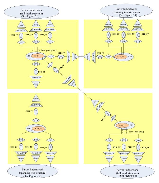
Figure 6-6 – EPLAN service architecture (spanning tree, multiple domains)
