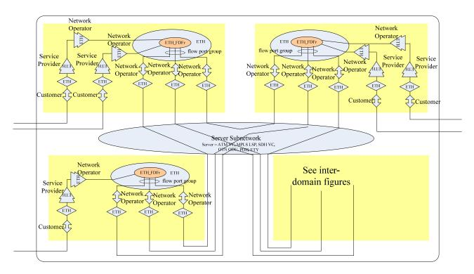
Figure 7-5 – Basic ETH MEP and MIP functions for the multipoint-to-multipoint Ethernet connection segment within the domain of one transport operator
