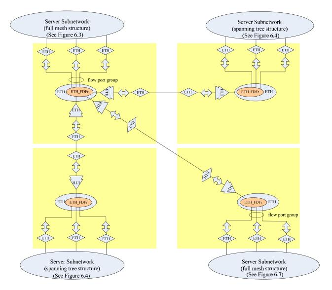
Figure 7-4 – Basic ETH MEP and MIP functions for the example in Figure 6-6
