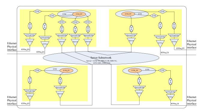
Figure 6-4 – EPLAN service architecture (spanning tree, single domain)
