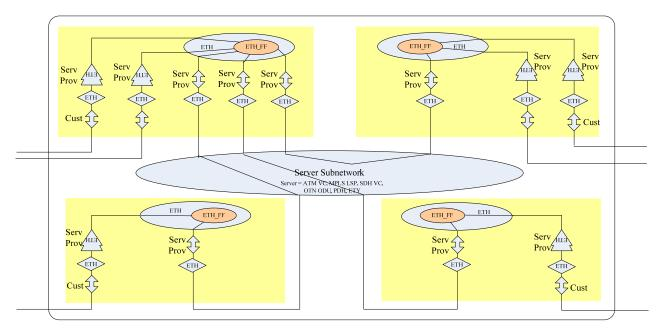
Figure 7-2 – Basic ETH MEP and MIP functions for the example in Figure 6-4
