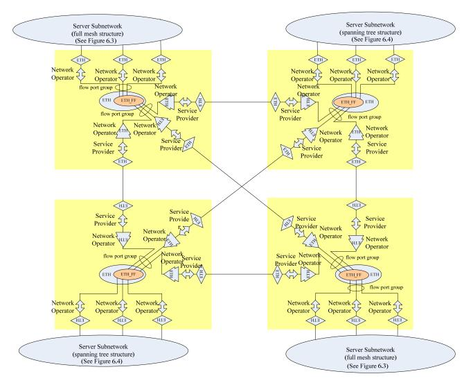
Figure 7-3 – Basic ETH MEP and MIP functions for the example in Figure 6-5
